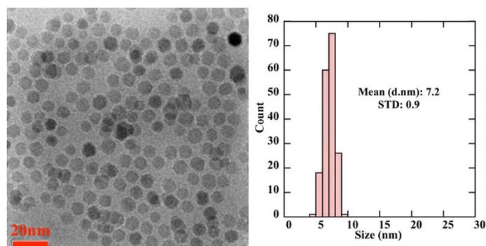
**Figure S1.** TEM micrograph of oleylamine coated magnetic nanoparticles on the left and histogram of particles size distribution on the right. Reprinted from (46) - Reproduced by permission of The Royal Society of Chemistry
