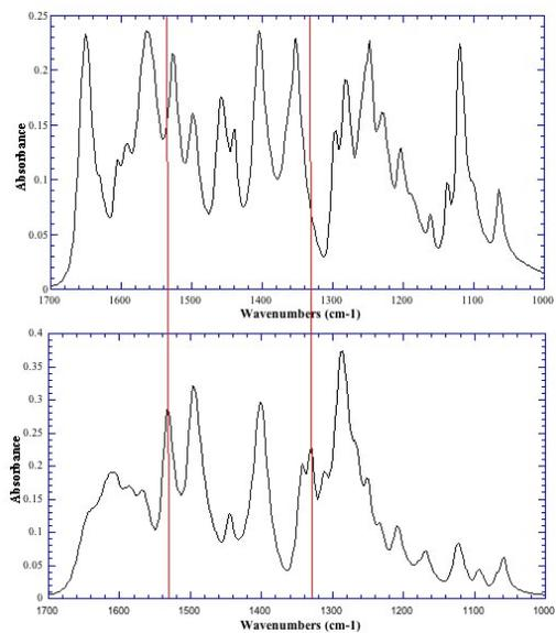
**Figure S2.** FTIR of DOPA (Top) and NitroDOPA (Bottom). Symmetric and asymmetric stretching from the NO<sub>2</sub> peaks at 1330 and 1532 cm<sup>-1</sup>. Reprinted from (46) - Reproduced by permission of The Royal Society of Chemistry.
