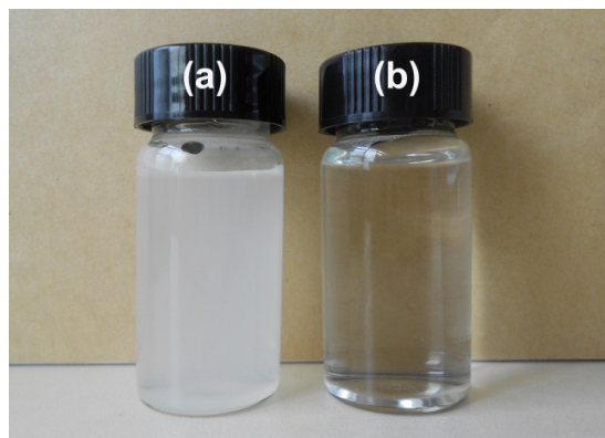
Figure S9. The image for solubility contrast between (a) CN-H 2 SO 4 and (b) acidified g-C 3 N 4 : 20 mg samples in 50 g of 0.5 M hydrochloric acid aqueous solution at 60 °C.
