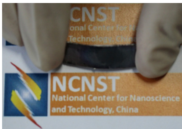
Figure S3. The photograph of the flexible as-prepared MoS 2 /graphite foil electrode.
