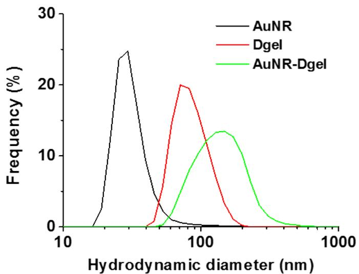
**Figure S1.** Hydrodynamic diameter distributions of AuNR, Dgel, and AuNR-Dgel determined by dynamic light scattering.
