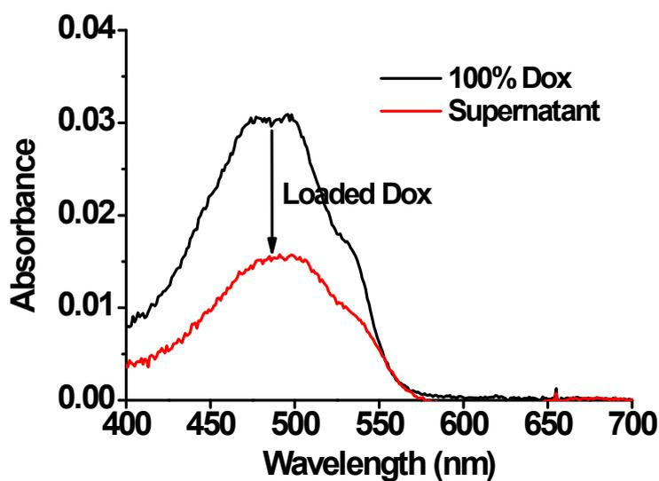
**Figure S3.** Absorption spectra of Dox before loading to the AuNR-Dgel (100% Dox) and the remained Dox supernatant measured after centrifugation of Dox-AuNR-Dgel at 5,000 g. The amount of loaded Dox was calculated using the absorbance decrease at 480 nm.
