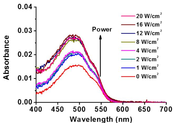
**Figure S4.** Absorption spectra of the Dox-AuNR-Dgel supernatant measured after laser irradiations at different power densities followed by centrifugation at 5,000 g. The percentage of released Dox was calculated using the absorbance increase at 480 nm.
