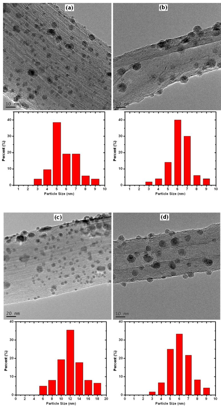
**Figure S6:** High resolution TEM images of (a) NiO-CNT-H<sub>2</sub> (thick), (b) NiO-CNT-H<sub>2</sub> (thin), (c) NiO-CNT-Ar (thick), and (d) NiO-CNT-Ar (thin). The bottom panels show the particle size distributions. The average particle sizes in NiO-CNT-H<sub>2</sub> (thick), NiO-
