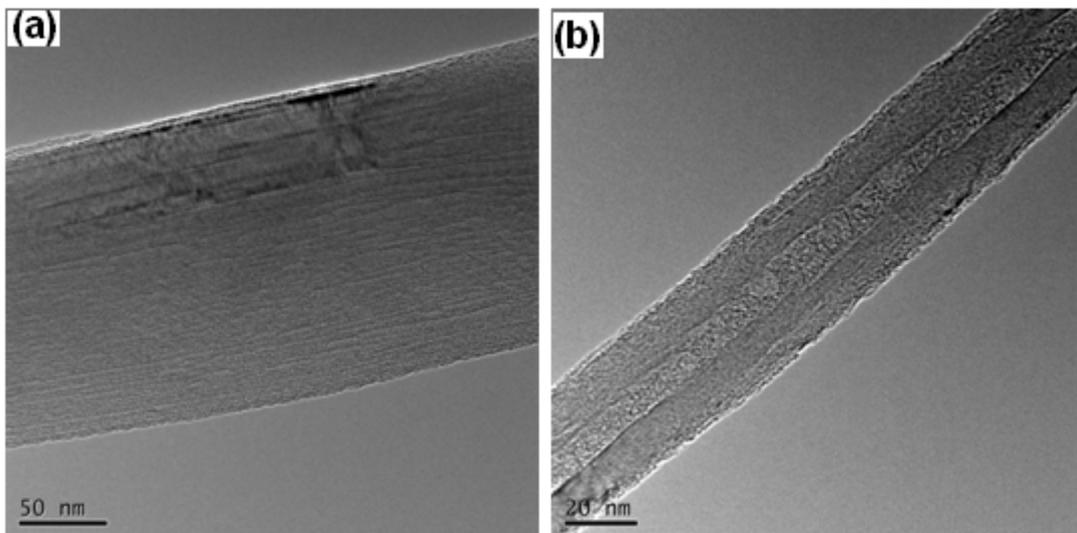
**Figure S1:** Magnified TEM images of (a) thick and (b) thin CNTs.
