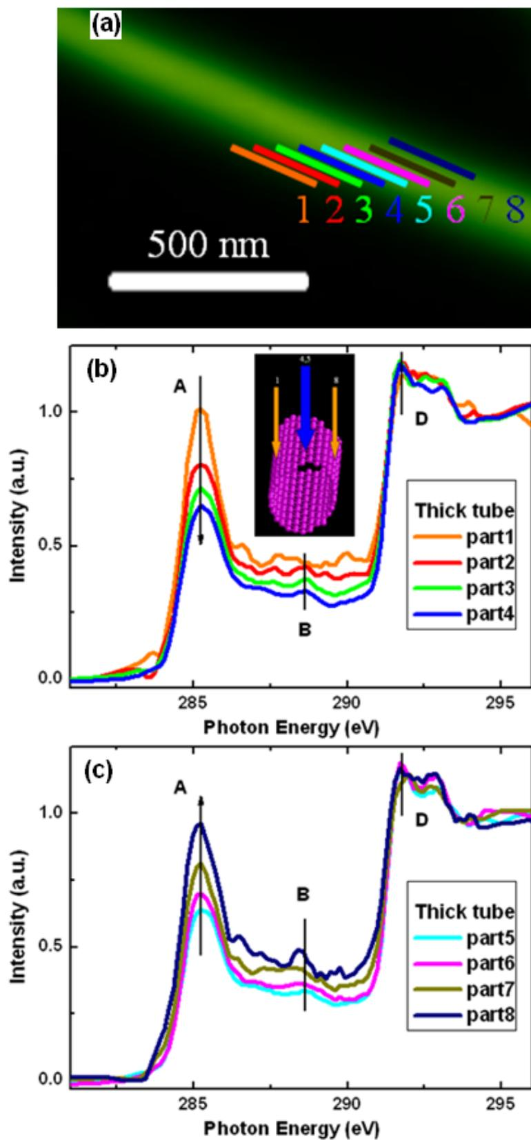
**Figure S4:** (a) STXM map of a thick tube; (b) and (c): C *K*-edge XANES spectra of a thick tube measured at different positions (1-8).
