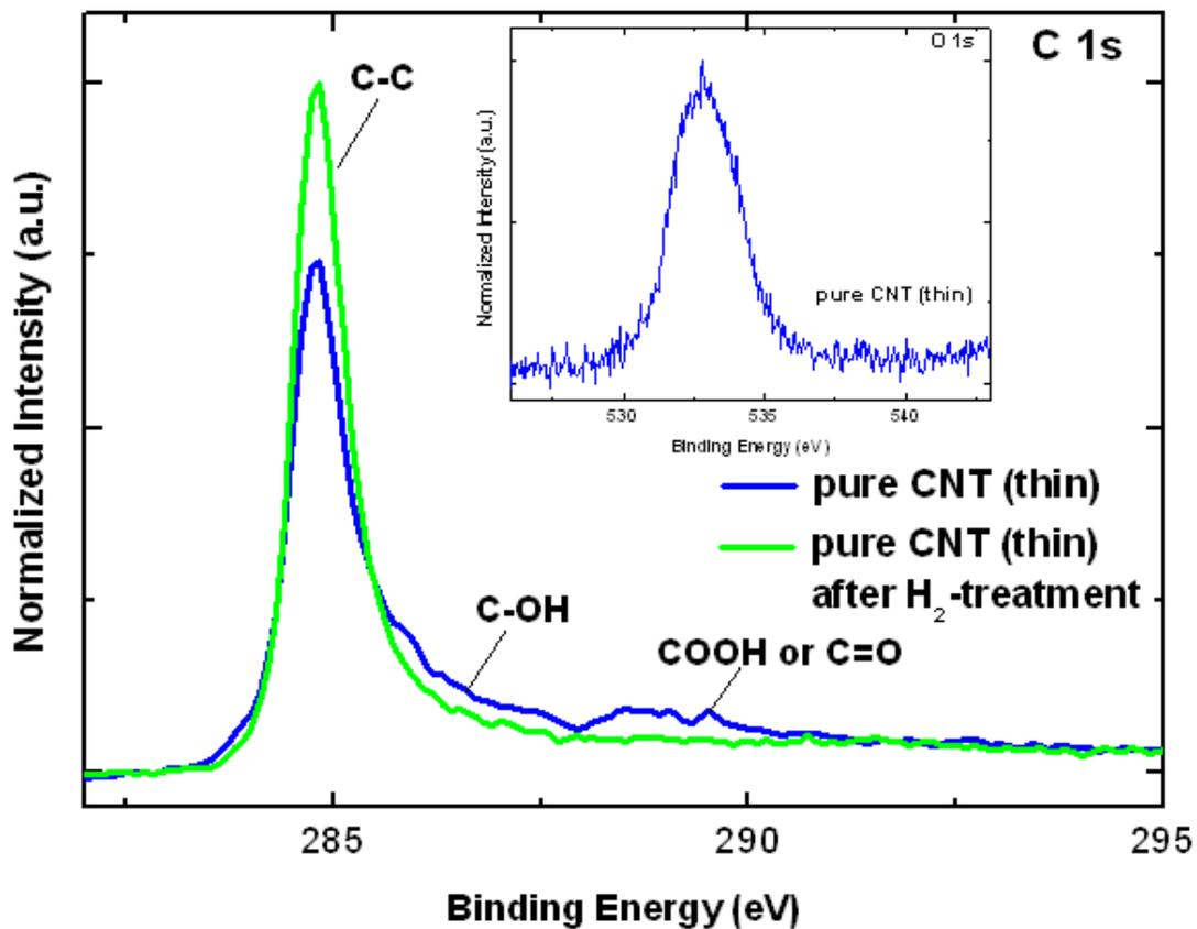
**Figure S2:** C 1s XPS results of pure CNT (thin) and pure CNT (thin) after H<sub>2</sub>-treatment.
