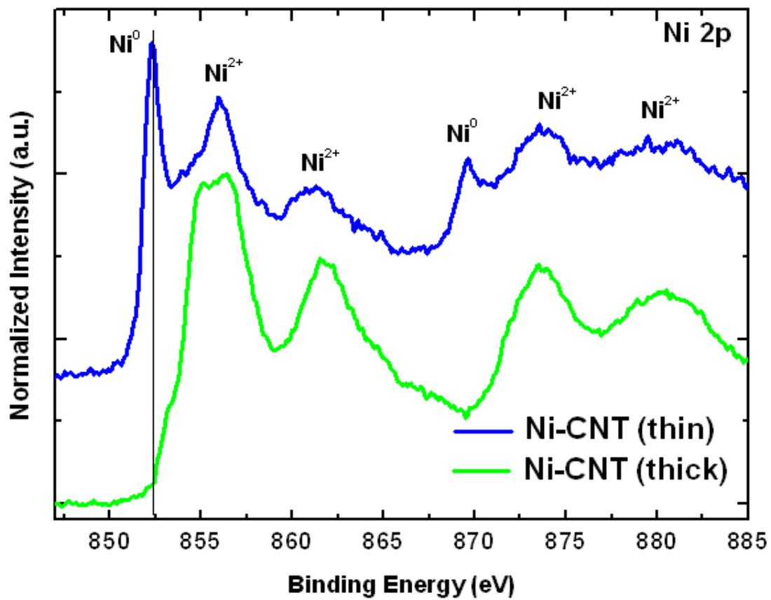
Figure S5: Ni 2p XPS results of Ni-CNT (thin) and Ni-CNT (thick).
