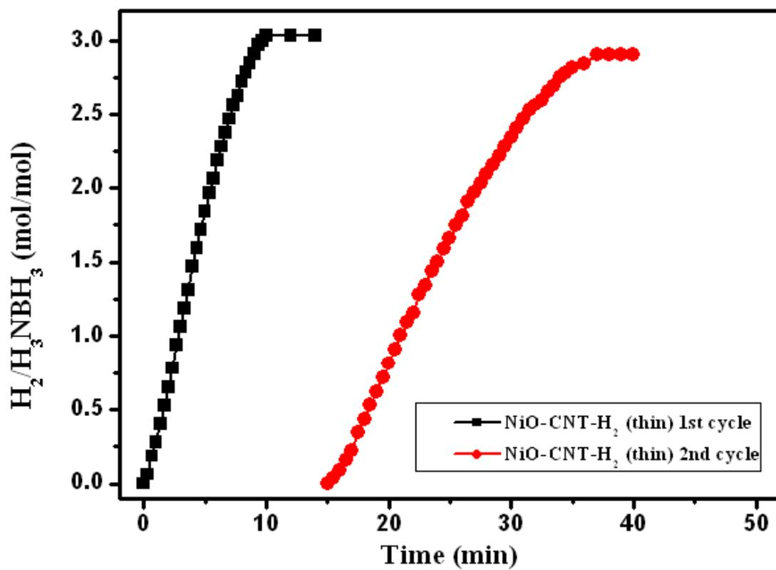
**Figure S7:** Stability test of NiO-CNT-H<sub>2</sub> (thin) in 2 runs for the hydrolysis of AB. The TOF value decreases from 19.07 to 7.2 (about 40% left).
