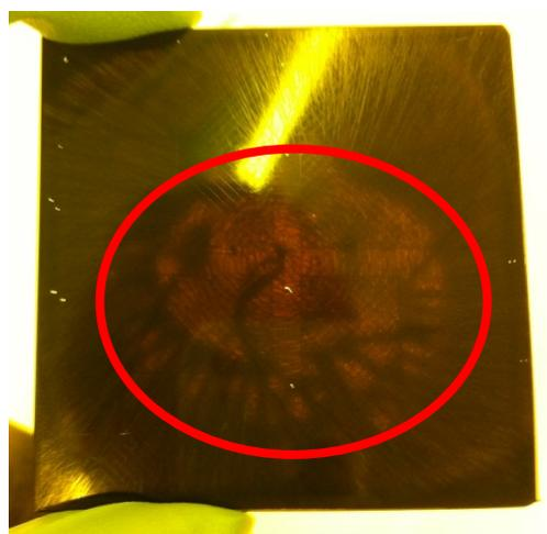
**Fig. S2** Picture of the PbS QD film on ITO glass (5 cm x 5 cm) after direct deposition of PEDOT:PSS
