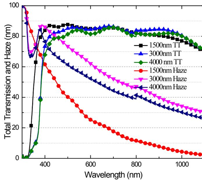
Figure S2. Spectra of the TT and the haze factor for periodically textured ZnO fabricated with different diameters of PS sphere
