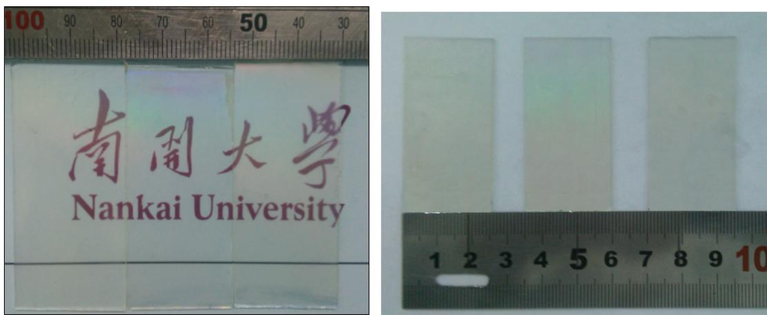
**The periodically textured ZnO thin films fabricated with different diameters of PS spheres**
