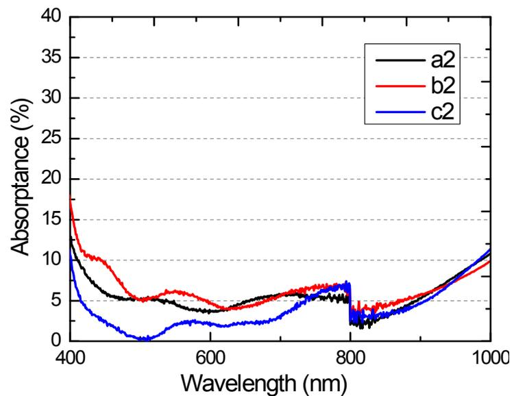
Figure S3. The absorption spectra of the periodically double-layer HZO/AZO TCFEs fabricated with different etching times.
