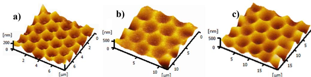
Figure S1. AFM images of the periodically textured ZnO thin films fabricated with different diameters of PS spheres: a) 1500nm, b) 3000nm, c) 4000nm
