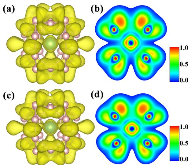
**Fig. S16** Isosurface of electron localization function (ELF) with the value of 0.75 and the contour plots of ELF within one plane through the principal axis of the endohedral D<sub>3h</sub> cage for MoB<sub>24</sub> (a, b) and WB<sub>24</sub> (c, d), respectively.
