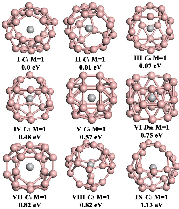
**Fig. S1** Structures of low-lying isomers of  $TiB_{24}$ . Bottom labels are point-group symmetries, spin multiplicities and relative energies to the ground state at PBE0/Ti/Stuttgart/B/6-311G\* level of theory, zero-point energy corrections were included for all isomers at the same level of theory.
