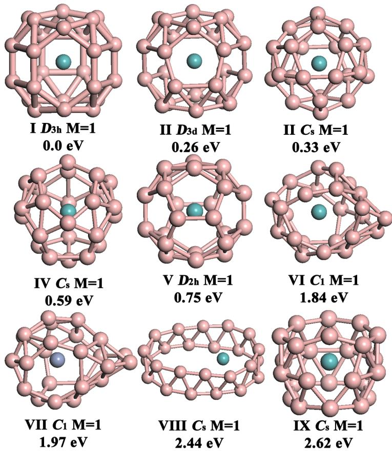
**Fig. S5** Structures of low-lying isomers of  $\text{MoB}_{24}$ . Bottom labels are point-group symmetries, spin multiplicities and relative energies to the ground state at PBE0/Mo/Stuttgart/B/6-311G\* level of theory, zero-point energy corrections were included for all isomers at the same level of theory.
