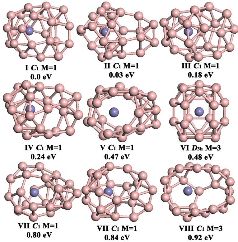
**Fig. S7** Structures of low-lying isomers of  $\text{FeB}_{24}$ . Bottom labels are point-group symmetries, spin multiplicities and relative energies to the ground state at PBE0/Fe/Stuttgart/B/6-311G\* level of theory, zero-point energy corrections were included for all isomers at the same level of theory.
