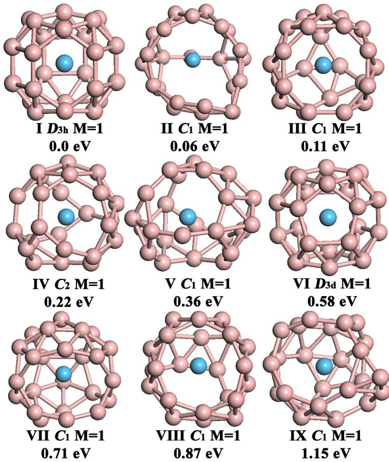
**Fig. S12** Structures of  $\text{HfB}_{24}^{2-}$  derived by re-optimizations of low-lying isomers of  $\text{HfB}_{24}$  in Fig. S3. Bottom labels are point-group symmetries, spin multiplicities and relative energies to the ground state at PBE0/Hf/Stuttgart/B/6-311+G\* level of theory, zero-point energy corrections were included for all isomers at the same level of theory.
