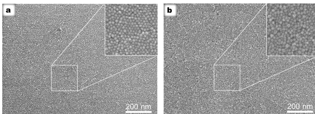
**Figure S8.** Wide-area SEM images of (a) a 120 nm thick film of oleate ITO NCs, and (b) a 130 nm thick film of octanoate ITO NCs on PET substrates fabricated by CSA. The zoomed-in images in the inset show the close-packed NC arrangement within the films in both cases.
