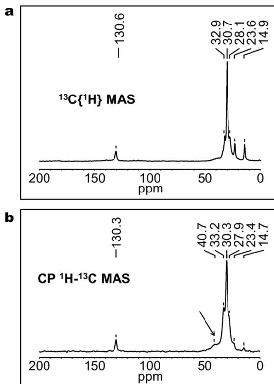
**Figure S7.** (a)  $^{13}\text{C}\{^1\text{H}\}$  MAS NMR spectrum and (b) cross-polarization  $^1\text{H}$ - $^{13}\text{C}$  MAS NMR spectrum of the oleate ITO NCs (the arrow points to the  $\alpha$ - $\text{CH}_2$  of oleylamine).
