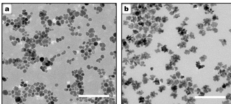
**Figure S2.** TEM images of ITO nanocrystals synthesized by mixing the In/Sn acetate precursors with both (a) octanoic acid and oleylamine, (b) butanoic acid and oleylamine in the beginning of the reaction and decomposed at 290 °C. Scale bars = 100 nm.
