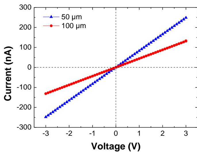
**Figure S9.** Typical current-voltage characteristics at 300 K of a 160 nm thick film of butanoate ITO NCs connected between two electrodes separated by gaps of 50  $\mu\text{m}$  (blue triangle symbols) and 100  $\mu\text{m}$  (red disk symbols).
