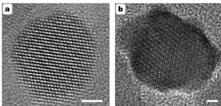
**Figure S4.** Representative HRTEM images of (a) octanoate and (b) butanoate ITO nanocrystals. Scale bars = 2 nm.
