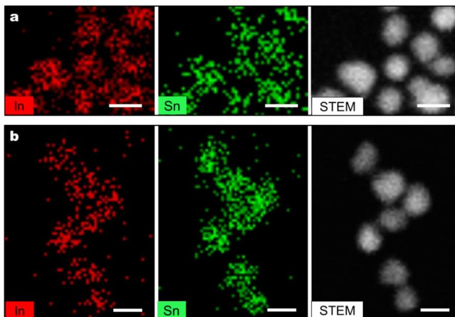
**Figure S5.** STEM-EDX elemental mappings of (a) octanoate and (b) butanoate stabilized ITO nanocrystals: indium map (left), tin map (center) and the corresponding overlay (right). Scale bars = 8 nm.
