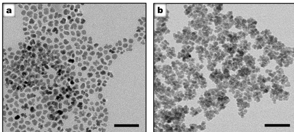
**Figure S1.** TEM images of ITO nanocrystals synthesized by auto-decomposition of (a) the In/Sn oleates (1:3 of In+Sn to oleic acid) and (b) the In/Sn octanoates (1:4 In+Sn to octanoic acid) at 290 °C. The NC morphology is different from that prepared by oleylamine injection at 290 °C, which yield spherical nanocrystals. Scale bars = 50 nm.
