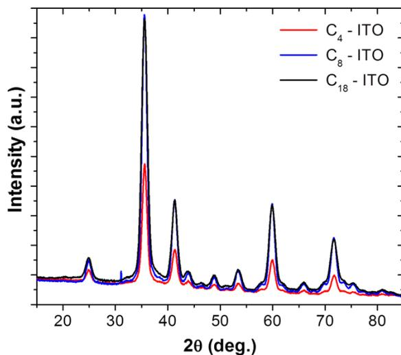
**Figure S3.** Typical powder XRD patterns of the oleate (black), octanoate (blue) and butanoate (red) ITO nanocrystals.
