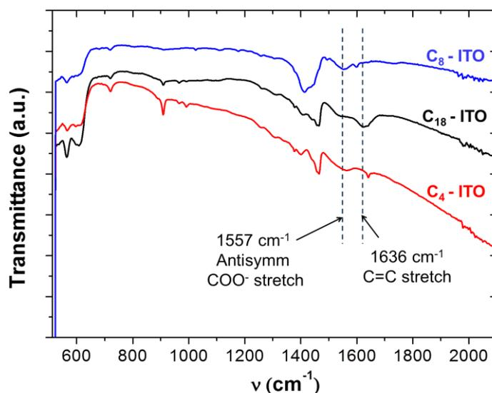
**Figure S6.** FT-IR of the oleate (black), octanoate (blue) and butanoate (red) stabilized ITO nanocrystals. The presence of carboxylate group is indicated by the broad signal at  $1557\text{ cm}^{-1}$ . Noteworthy is the absence of the C=C stretching signal at  $1636\text{ cm}^{-1}$ , in the octanoate ITO NC sample. A sharp signal around this frequency for butanoate ITO NC sample suggests the presence of free oleylamine.
