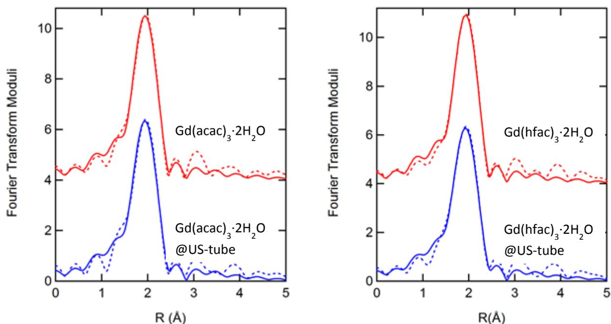
**Figure S2.** The Fourier transforms of the EXAFS data (dashed lines) and their fittings (full lines). On the left:  $\text{Gd}(\text{acac})_3 \cdot 2\text{H}_2\text{O}$  and  $\text{Gd}(\text{acac})_3 \cdot 2\text{H}_2\text{O}@US\text{-tubes}$ ; on the right:  $\text{Gd}(\text{hfac})_3 \cdot 2\text{H}_2\text{O}$  and  $\text{Gd}(\text{hfac})_3 \cdot 2\text{H}_2\text{O}@US\text{-tubes}$ .
