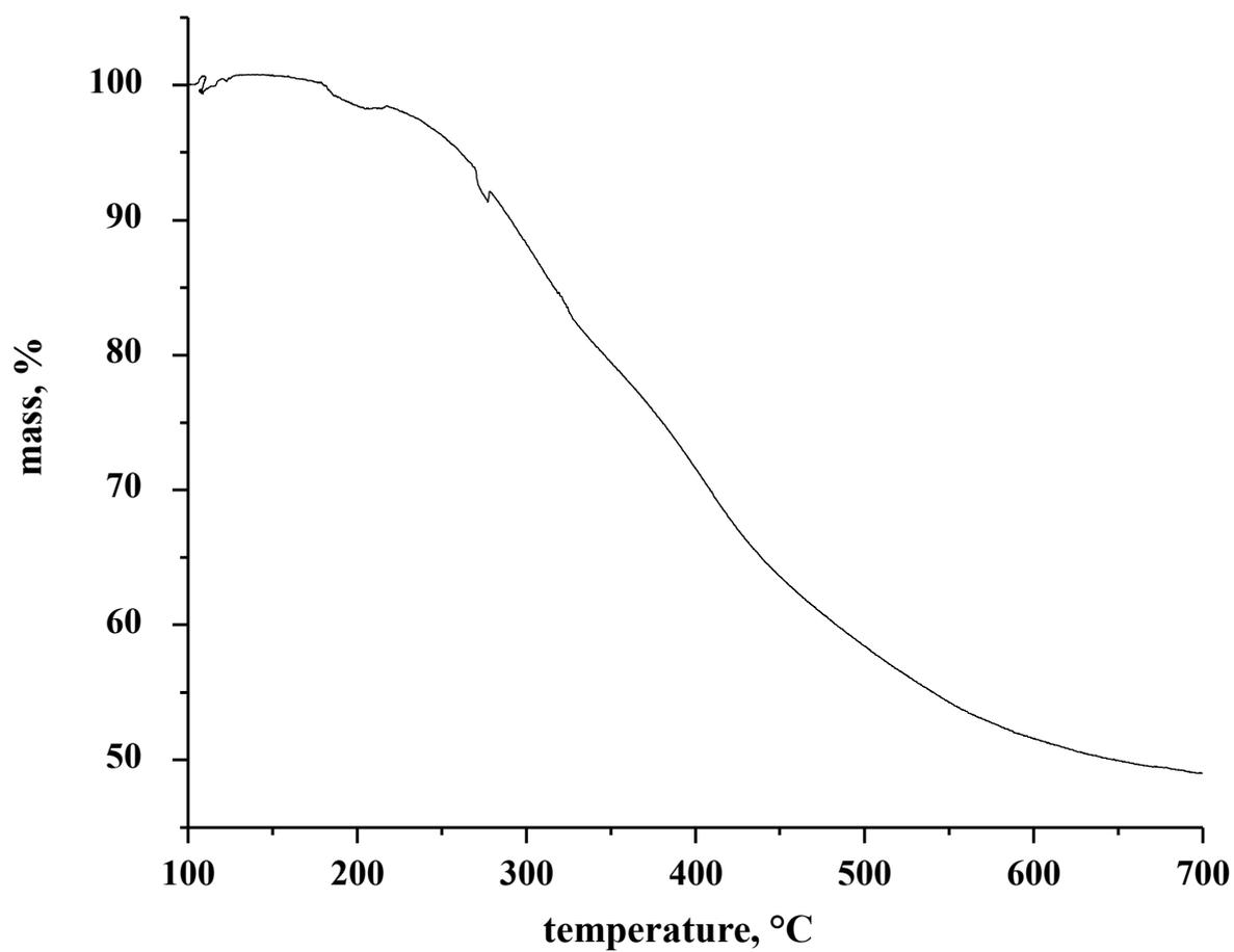
**Figure S3.** Thermal gravimetric analysis (TGA) of the PCP-Gd(acac)<sub>3</sub>•2H<sub>2</sub>O@US-tubes (functionalized 4 times) in an Ar atmosphere at a 10 °C min<sup>-1</sup> scan rate, from 100 to 700 °C.
