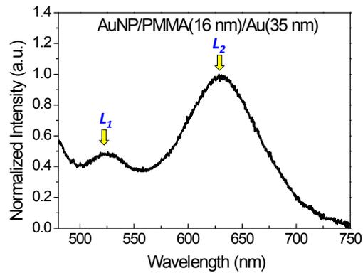
**Figure S2.** Measured dark-field scattering spectra for a single AuNP on a 16-nm-thick PMMA spacer on a 35-nm-thick Au film. The peak at ~535 nm and ~630 nm were attributed to  $L_1$  and  $L_2$  modes, respectively.
