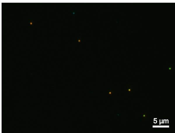
**Figure S4.** A representative dark-field image of AuNP/PMMA(16 nm)/Au film(35 nm). Both “green” and “red” particles can be observed. The formation of “red” particles in this case was attributed to the strong vertical image dipole coupling ( $L_2$ ) which can exist at sub-20-nm spacer thickness.
