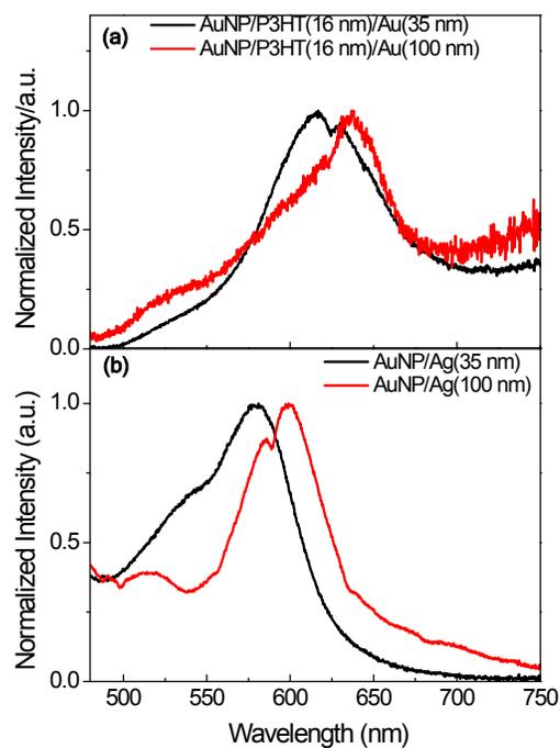
**Figure S1.** Single-particle dark-field spectroscopy of AuNP on (a) a thin P3HT spacer with underlying Au film of different thickness; (b) Ag film of different thickness. In both cases with the increase of thickness of underlying plasmonic metal substrate, the predominant peak at ~600 nm red shifts, which indicates a stronger interaction between vertically polarized LSPR and the image dipole.
