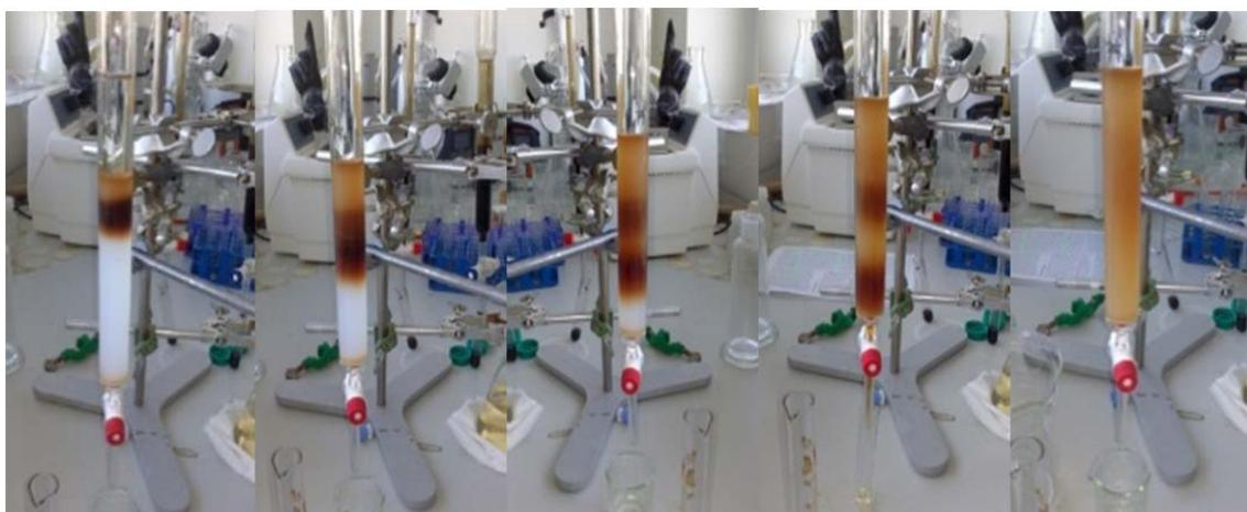
**Figure 8:** Sephadex G75-column purification/separation of the PEGylated products. Pictures were taken over the time of the purification to show separation into different fractions.
