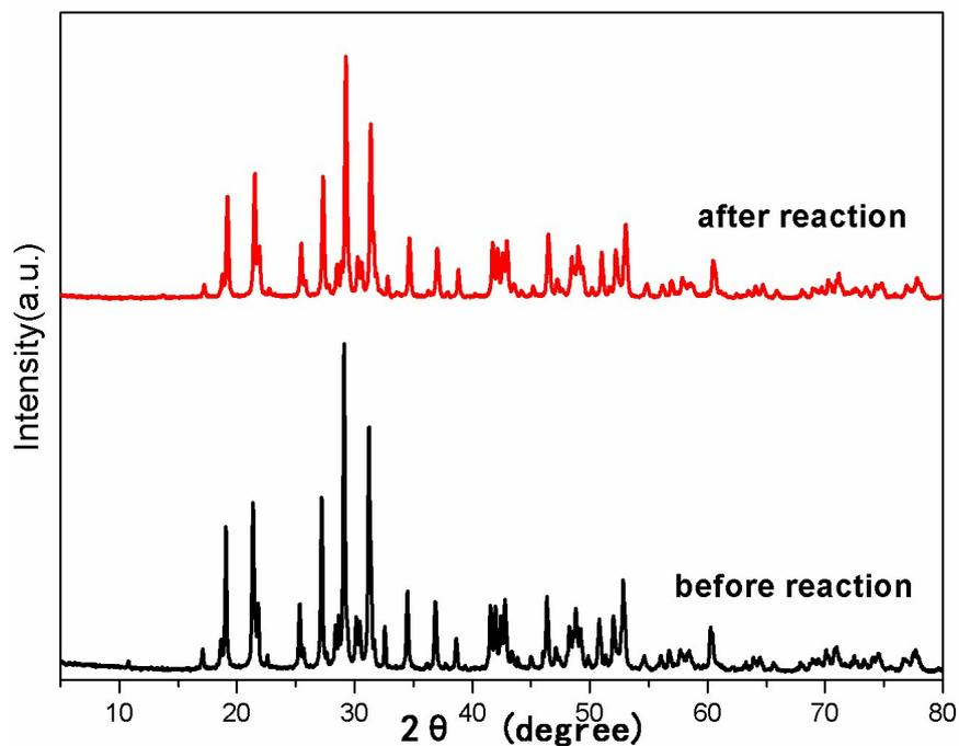
Fig. S5 XRD patterns of cal.  $140^\circ\text{C}$  after 5 cycles of degradation of MB solution
