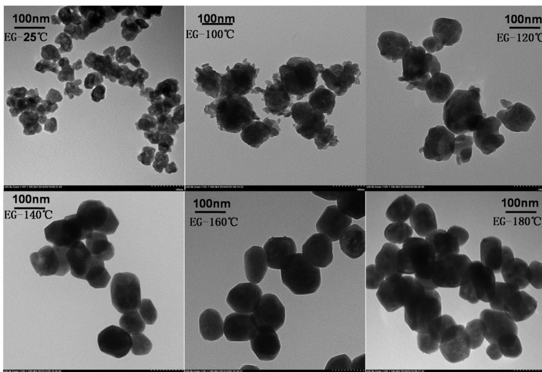
Fig. S1C TEM images of BiPO<sub>4</sub> synthesized at different reaction temperatures for 48 h
