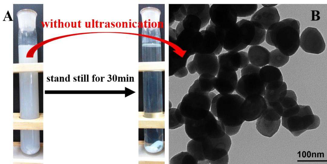
Fig. S7 Optical photos and TEM images of of catalysts cycled for 5 times without ultrasonication.
