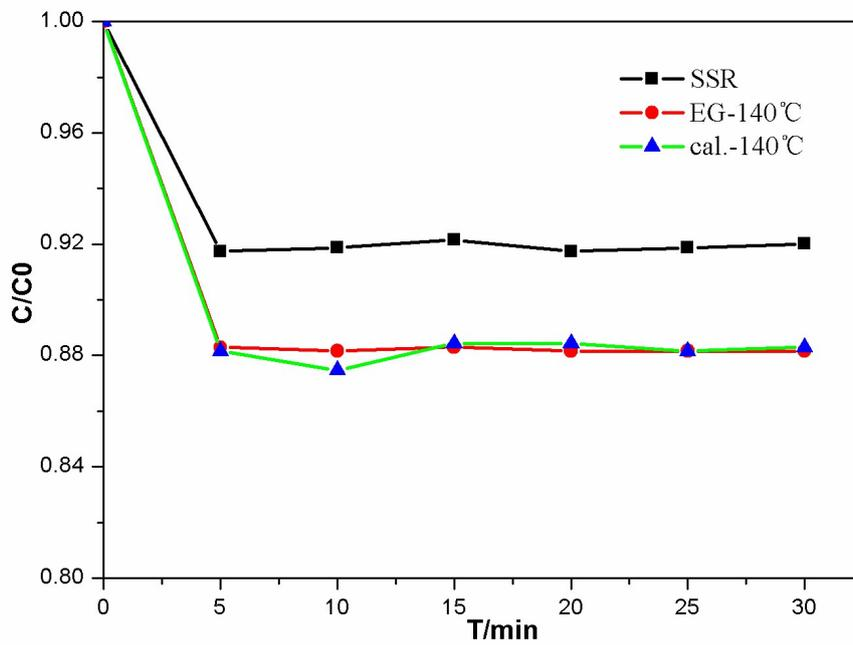
Fig. S2 The adsorption of SSR, EG-140°C, and cal.-140°C on the degradation of MB solution, in dark
