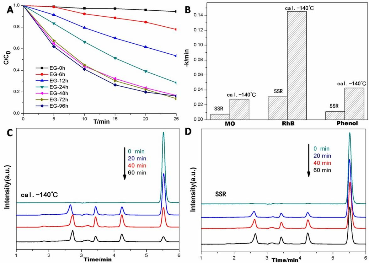
Fig. S4 (A) Degradation curves of MB ( $1 \times 10^{-5}$  mol/L) by  $\text{BiPO}_4$  prepared by different solvothermal time; (B) Apparent rate constants of degrading MO, RhB and phenol by SSR and cal.  $140^\circ\text{C}$ ; (C) and (D) are liquid chromatography of degrading phenol by cal.  $140^\circ\text{C}$  and SSR respectively.
