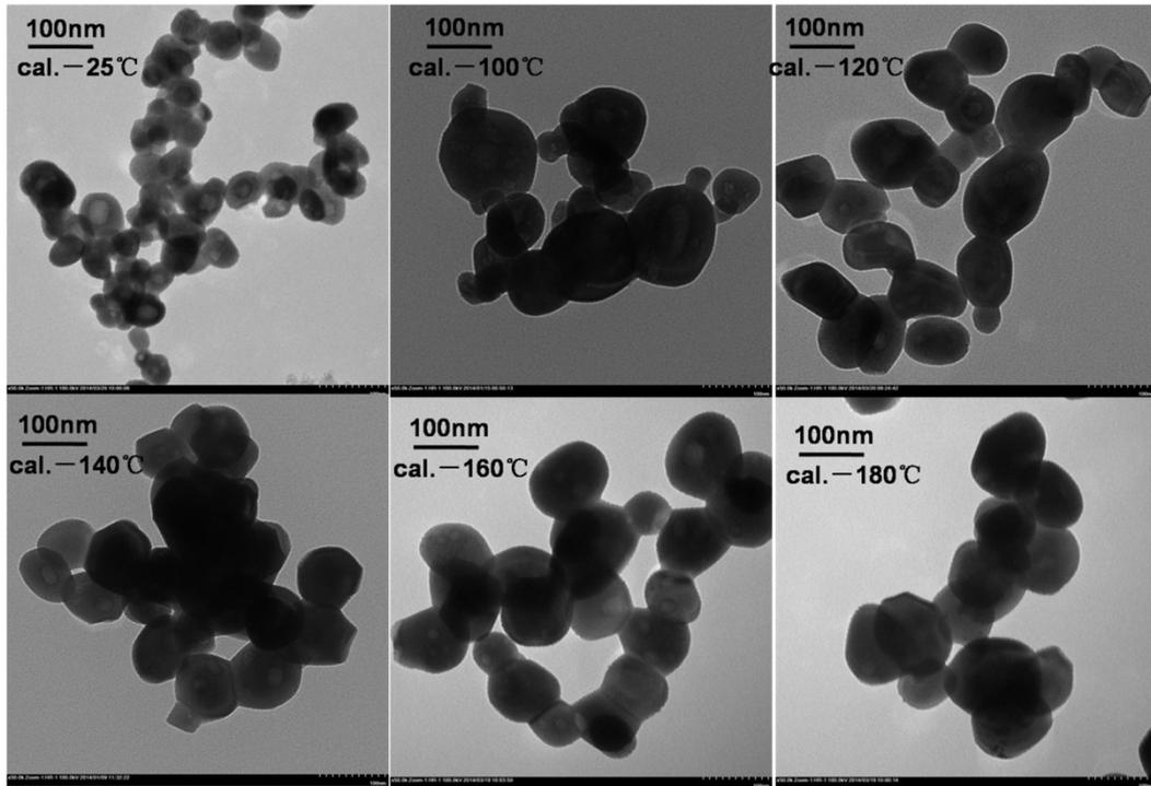
Fig. S1D TEM images of calcinated BiPO<sub>4</sub> synthesized at different solvothermal temperatures
