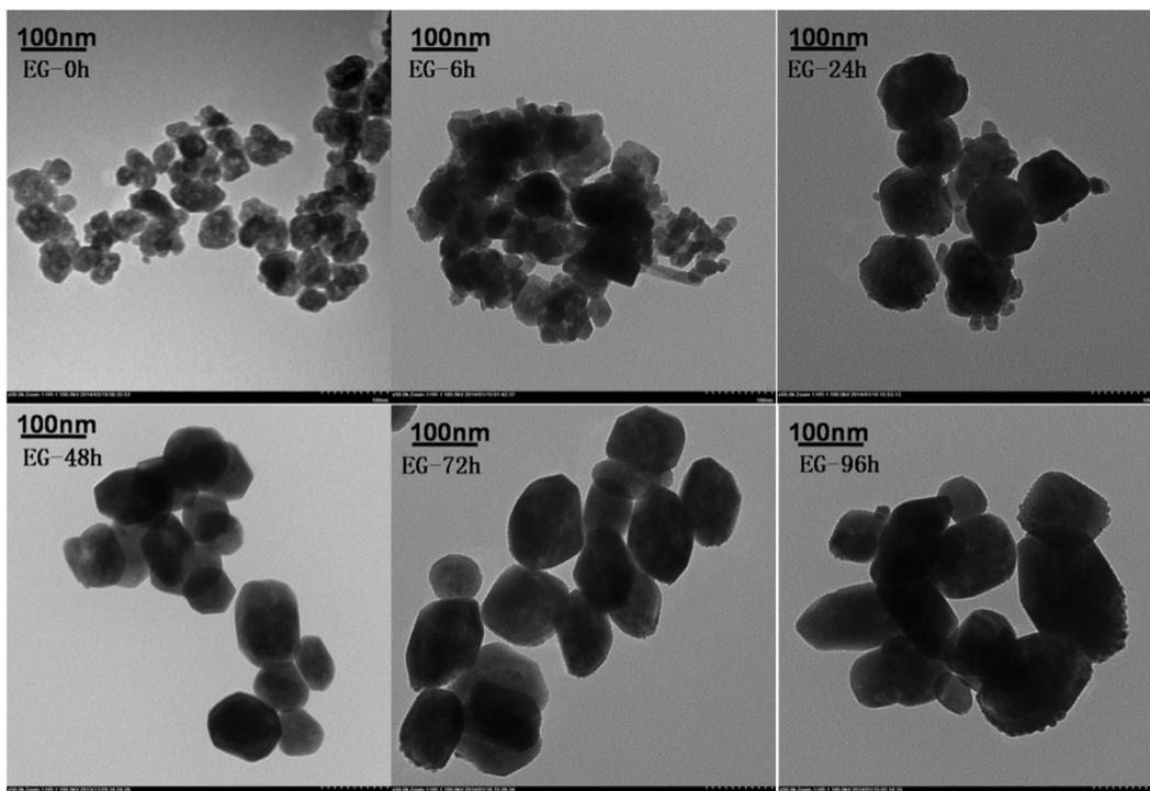
Fig. S1B TEM images of BiPO<sub>4</sub> synthesized at 140°C for different reaction time
