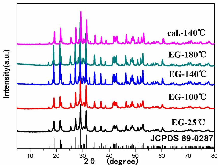
Fig. S1A XRD patterns of BiPO<sub>4</sub> synthesized at different reaction temperatures
