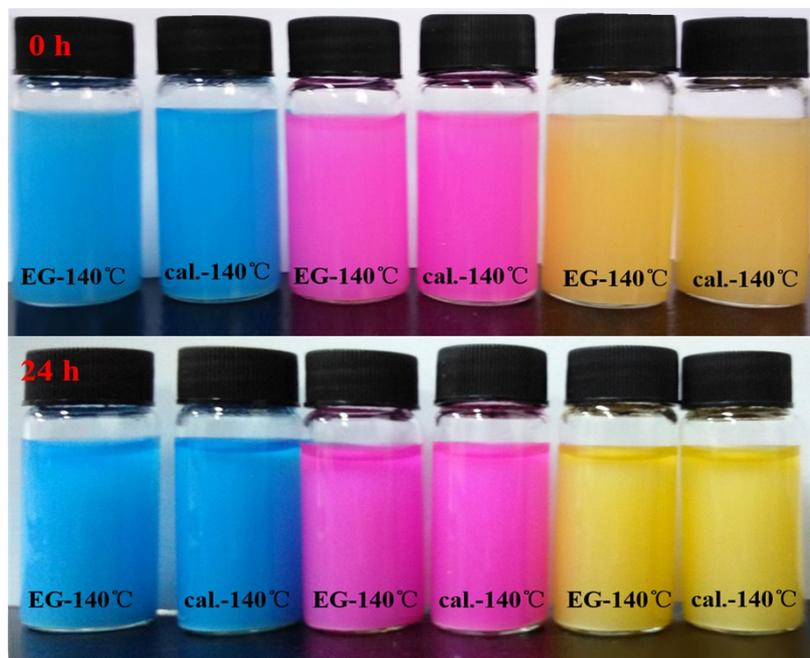
Fig. S3 Photos of EG-140°C and cal.-140°C dispersed in MB, RhB and MO  $2 \times 10^{-5}$  mol/L solutions stand for 0h (upper) and 24h (lower)
