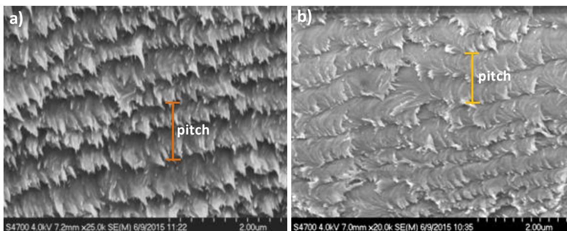
**Figure S3.** SEM images viewed perpendicular to fracture cross-sections of the GeO<sub>2</sub>/CNC composite films prepared using the water/DMF ratio of 1:1 (a) and 1:2 (b).
