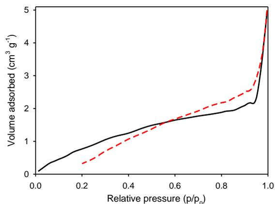
**Figure S7.** N<sub>2</sub> adsorption and desorption isotherms of chiral nematic GeO<sub>2</sub> films (**Ge-A**) obtained from calcination of the GeO<sub>2</sub>/CNC composite film under air. This material has very low surface area.
