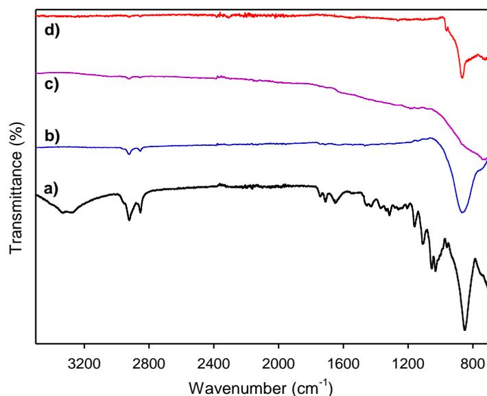
**Figure S4.** FTIR spectra of chiral nematic GeO<sub>2</sub>/CNC composite film GeO<sub>2</sub>/CNC (a) and the corresponding chiral nematic GeO<sub>2</sub> films **Ge-A** (b), mesoporous Ge/C composite film **Ge-H** (c) and GeO<sub>2</sub>/C composite film **Ge-N** (d).
