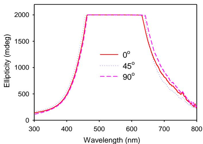
**Figure S2.** CD spectra of a GeO<sub>2</sub>/CNC composite film obtained by rotating the sample from 0° to 90°. No significant change is observed, indicating that the positive signal is not dominated by linear birefringence.
