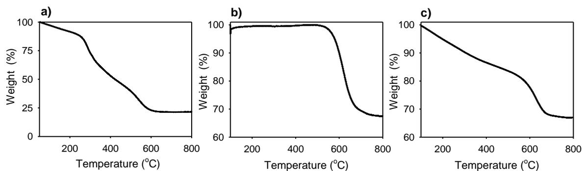
**Figure S5.** TGA curve of (a) the chiral nematic GeO<sub>2</sub>/CNC composite film and the corresponding chiral nematic mesoporous (b) Ge/C composite film **Ge-H** and (c) GeO<sub>2</sub>/C composite film **Ge-N**.
