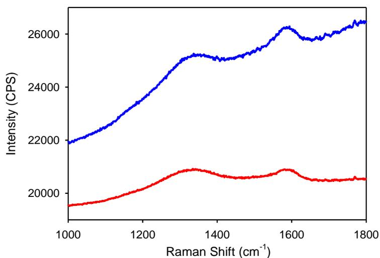
**Figure S8.** Raman spectra of chiral nematic mesoporous Ge/C film (**Ge-H**, blue line) and GeO<sub>2</sub>/C composite film (**Ge-N**, red line).
