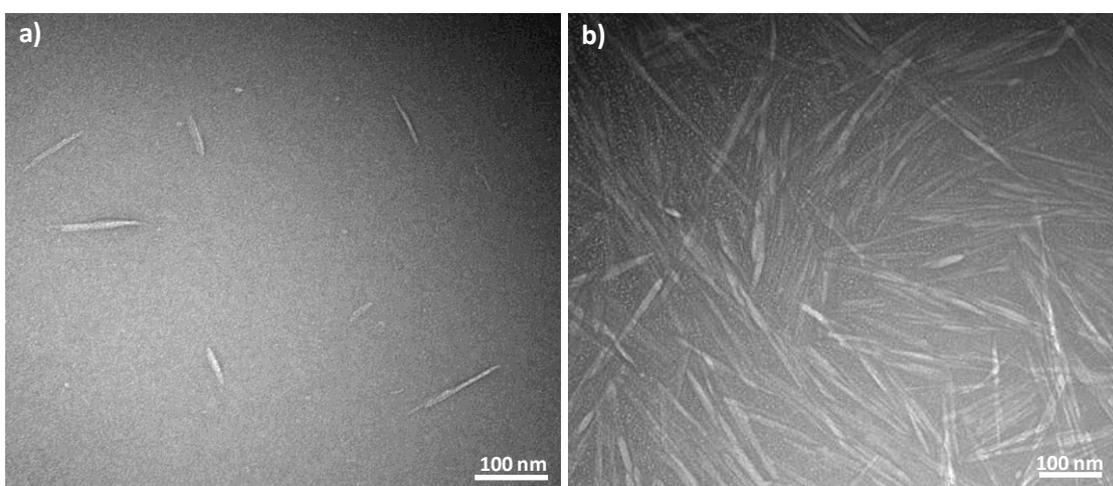
**Figure S1.** TEM images of the aqueous solution of CNCs (0.002 wt%).
