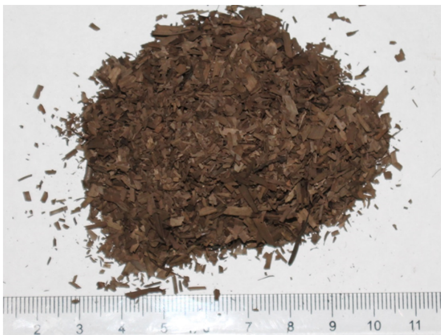
Figure S1. Optical photograph of HC-leached dead bamboo leaves (BLs).
