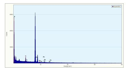
Figure S2 EDAX of Au-0.1NG-T composite to show the presence of all constituent elements including Au and nitrogen.
