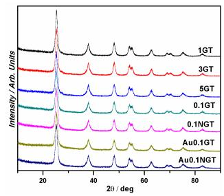
Figure S1 XRD pattern Au-RGO/NRGO-TiO<sub>2</sub> composites. Except anatase features, no other features could be observed.
