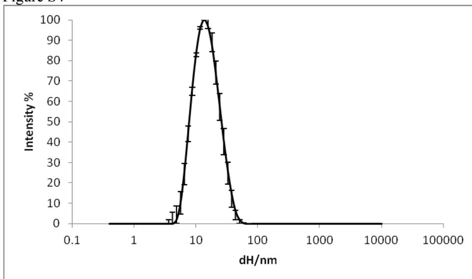
Figure S4. Intensity averaged hydrodynamic size distribution obtained fitting the DLS auto-correlation functions by cumulant analysis of Fe<sub>3</sub>O<sub>4</sub> NPs stabilized by oleic acid in toluene.
