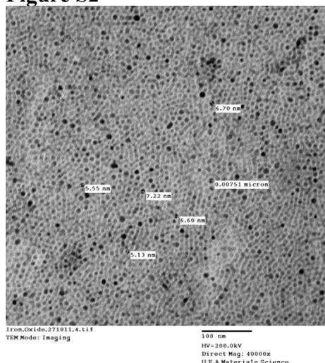
Figure S2. TEM image of Fe<sub>3</sub>O<sub>4</sub> NPs stabilized by oleic acid and dispersed in toluene. 1 drop of the dispersion was placed on the carbon film 300 mesh Cu(50)(Agar Scientific). The instrument was Joel 200EX with tungsten filament and acceleration voltage of 180kV to 200kV.
