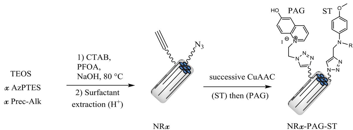
**Scheme S1:** Synthetic route for obtaining bifunctional nanorods from original precursors *via* CuAAC click reaction
