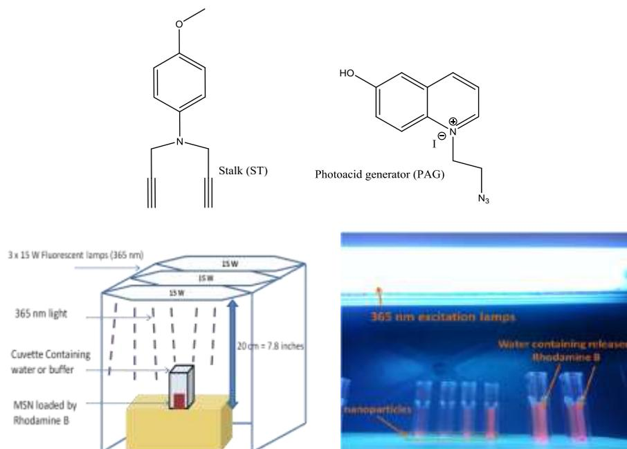
**Figure S7:** (Above) Molecular structure of the photoacid and the stalk and (below) light excitation setup.
