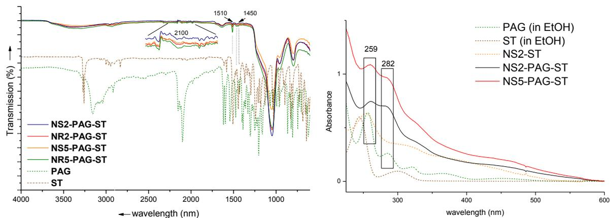
**Figure S9:** (left) FTIR spectra of bislicked nanoparticles: (blue) 2% and (orange) 5% nanospheres with (red) 2% and (green) 5% nanorods. Dashed lines correspond to the (green) AHQI (PAG) and (brown) Alk-anisidine (ST) precursors. Inset: zoom on  $N_3$  peak in the zone  $2050-2150\text{ cm}^{-1}$  (right) UV-vis spectra of the *clicked* nanospheres.
