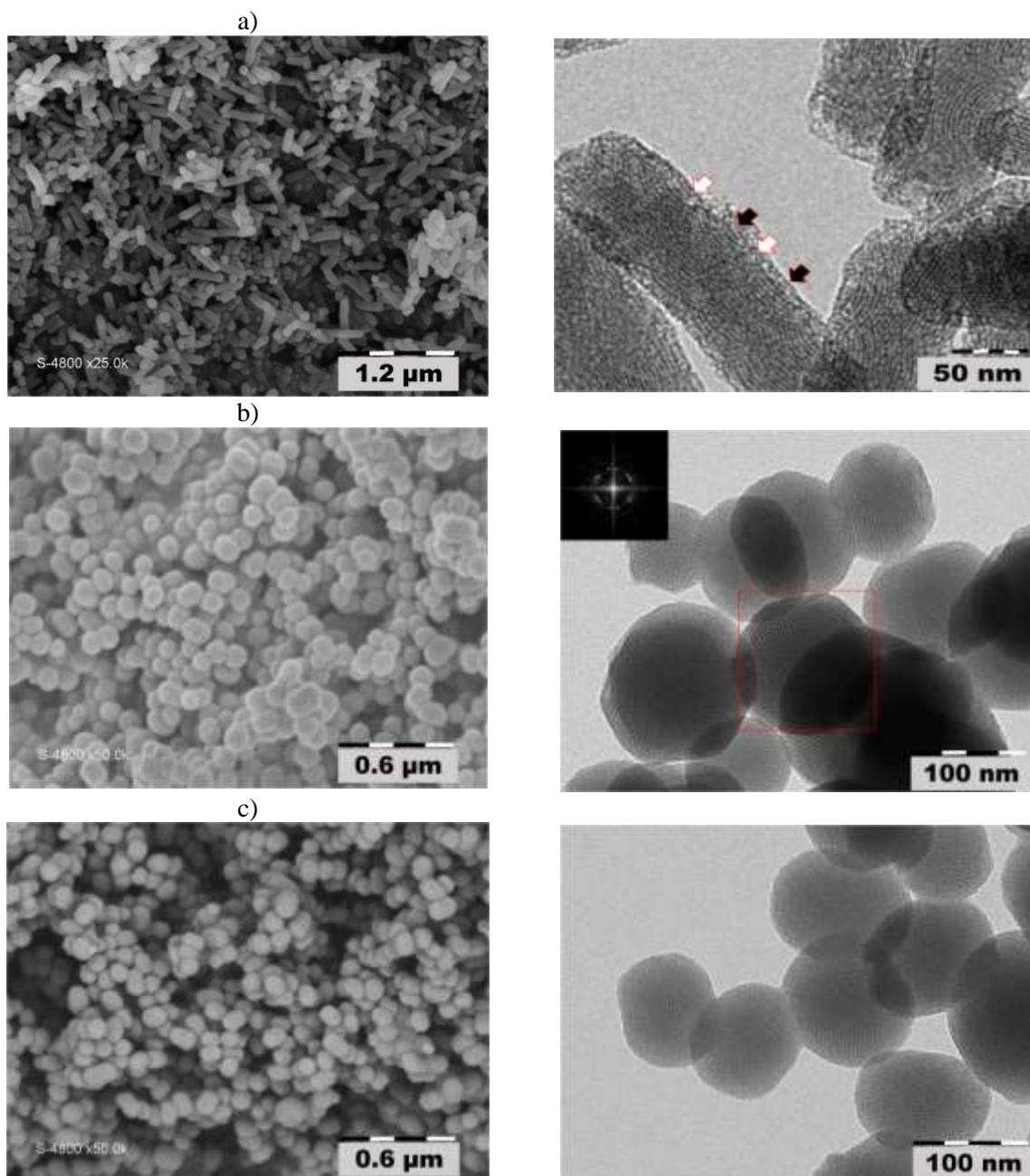
**Figure S2:** Images obtained by (left) SEM and (right) TEM of a) NR2 b) NS2 and c) NS5. SEM shows nanospheres with narrow sizes (100-150 nm). TEM shows ordered pore channels and the inset in b) is the FFT of the selected part of the image indicating a 2D-hexagonal structure.
