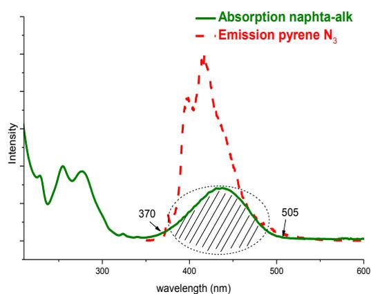
**Figure S4:** Spectral overlap between the emission of the donor and the excitation of the acceptor
