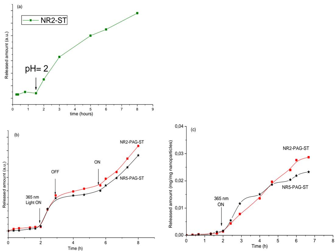
**Figure S13:** Release profiles of rhodamine B: (a) in pure water with bulk acidification for control NR2-ST; sequential on/off cycles (b) in pure water and (c) in Tris buffer. Red, black and green traces correspond to NR2-PAG-ST, NR5-PAG-ST and NR2-ST, respectively.
