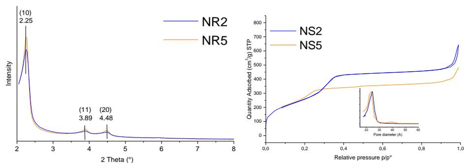
**Figure S3:** (left) X-ray diffractograms and (right) N<sub>2</sub> physisorption of parent bisclickable nanospheres. (inset: BJH plot)
