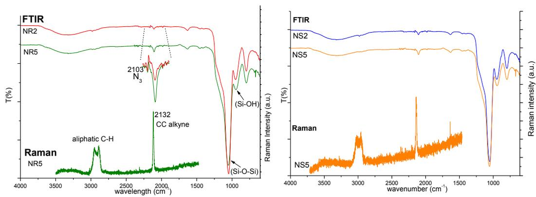
**Figure S1:** FTIR and Raman spectra of parent bisclickable (left) nanorods and (right) nanospheres
