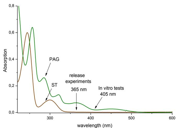
**Figure S12:** Absorption spectra of the photoacid PAG and the stalk ST with the used wavelength corresponding to release experiments with rhodamine B and in vitro tests with doxorubicin
