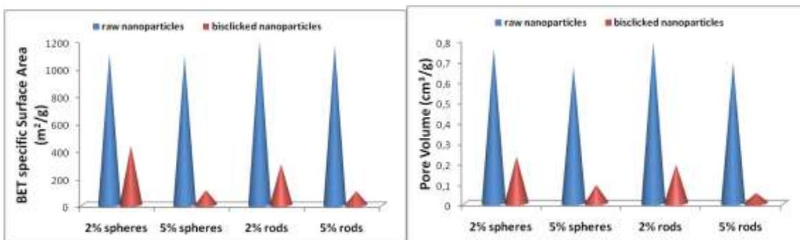
**Figure S11:** Evolution of the (left) specific surface area and (right) total pore volume in (blue cones) parent and (red cones) bislicked nanoparticles
