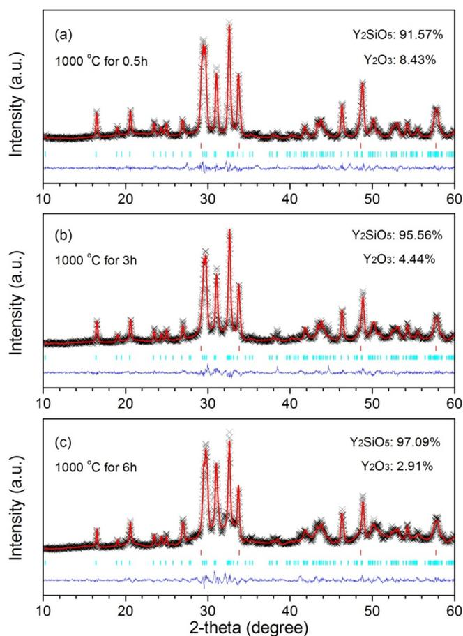
**Figure S1.** Refined XRD patterns of products sintering at 1000 °C for 0.5 h (a), 3 h (b) and 6 h (c). The refined percentage of  $Y_2O_3$  and  $Y_2SiO_5$  content is also shown here. Crosses: experimental; red solid line: calculated XRD patterns; blue solid line: difference. Two set of tick marks show the Bragg reflection positions of the phases  $Y_2O_3$  (red) and  $Y_2SiO_5$  (cyan).
