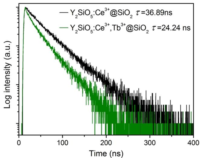
**Figure S6.** Decay curves of  $\text{Y}_2\text{SiO}_5:\text{Ce}^{3+}@\text{SiO}_2$  and  $\text{Y}_2\text{SiO}_5:\text{Ce}^{3+}, \text{Tb}^{3+}@\text{SiO}_2$  nanoparticles.
