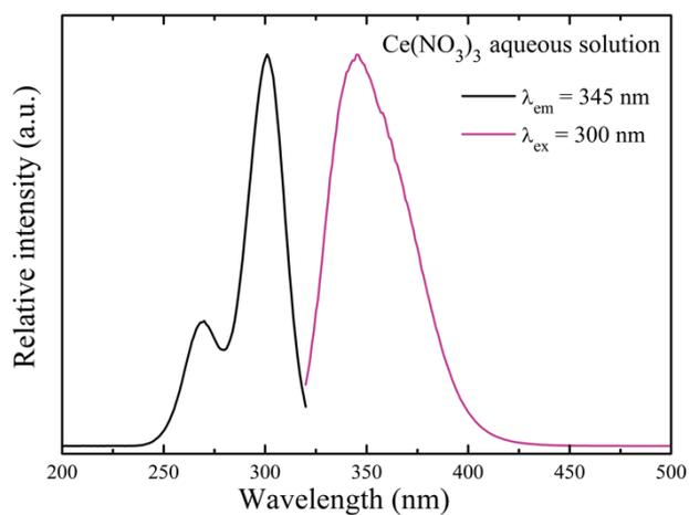
**Figure S5.** Photoluminescence excitation and emission spectra of  $\text{Ce}(\text{NO}_3)_3$  aqueous solution.
