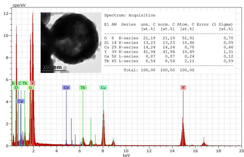
**Figure S4.** EDX spectrum of hollow  $\text{Y}_2\text{SiO}_5: 1\%\text{Ce}^{3+}, 9\%\text{Tb}^{3+}$  nanowalnuts, the inset shows the TEM image. The atomic ratios of Y, Ce and Tb is estimated to be 18.49: 0.24: 2.11, which is very closed to 90: 1: 9.
