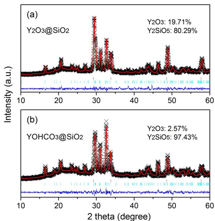
**Figure S3.** Refined XRD patterns of products from annealing  $\text{Y}_2\text{O}_3@\text{SiO}_2$  (a) and  $\text{YOxHCO}_3@\text{SiO}_2$  (b) core-shell nanostructures at 950 °C for 3 h.
