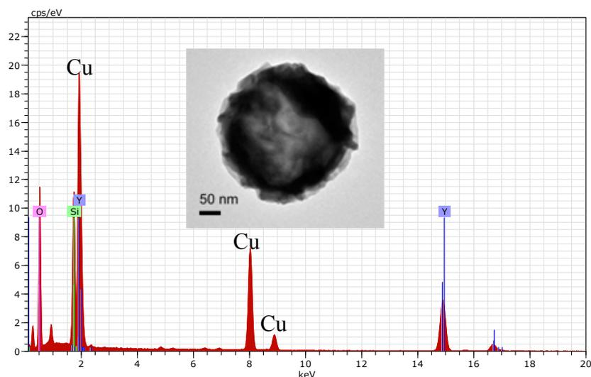
**Figure S2.** EDX spectrum of hollow  $\text{Y}_2\text{SiO}_5$  nanowalnuts, inset shows the TEM image. The atomic ratios of Y, Si and O is 3:2:5. Cu signal comes from the Cu support substrate.
