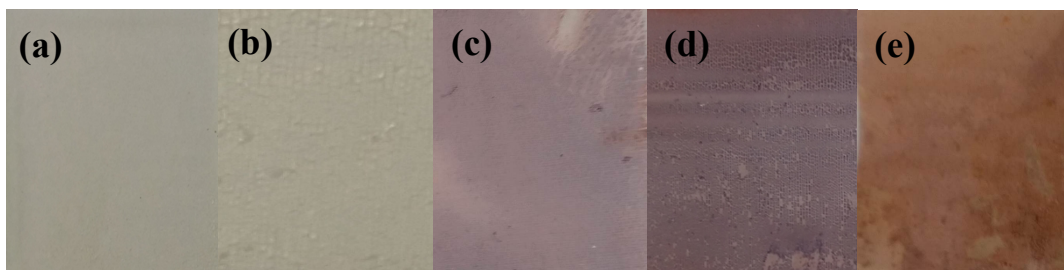
Fig. S1 (a-e) Photos of S1-S5 3DIO thin film on the glass substance. The photos were taken under normal indoor environment.
