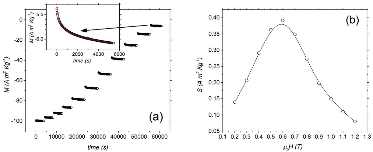
Figure S2. The time dependence of the magnetization reversal is reported in panel (a), with different field applied. For the 1.2 T field the experimental data (black circles) are reported both with the best fit (red line) using equation (1). The magnetic viscosity measured at each field is reported in panel (b).
