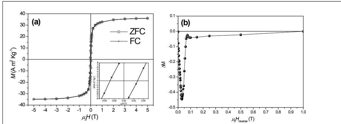
Figure S3: (a) Hysteresis loops recorded at 5 K in ZFC condition (big empty cycles) and cooling the samples under an applied field of 3T (small full circles); Inset: detail in the field range  $\pm 0.05$  T.
