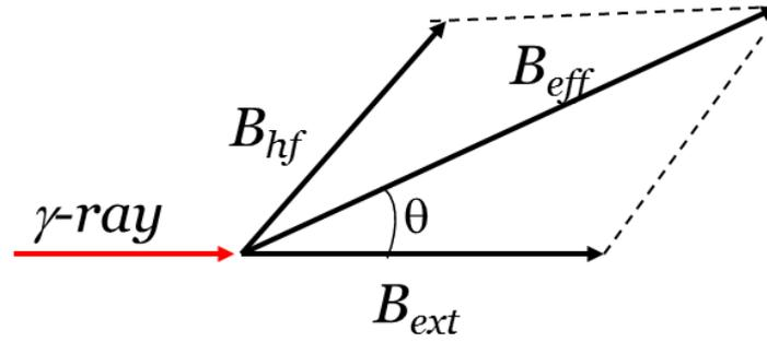
Figure S4. The setup for  $^{57}\text{Fe}$  Mössbauer spectroscopy and the relation between the effective field ( $B_{\text{eff}}$ ) and the external applied field ( $B_{\text{ext}}$ ) which differ by the average canting angle  $\theta$ .
