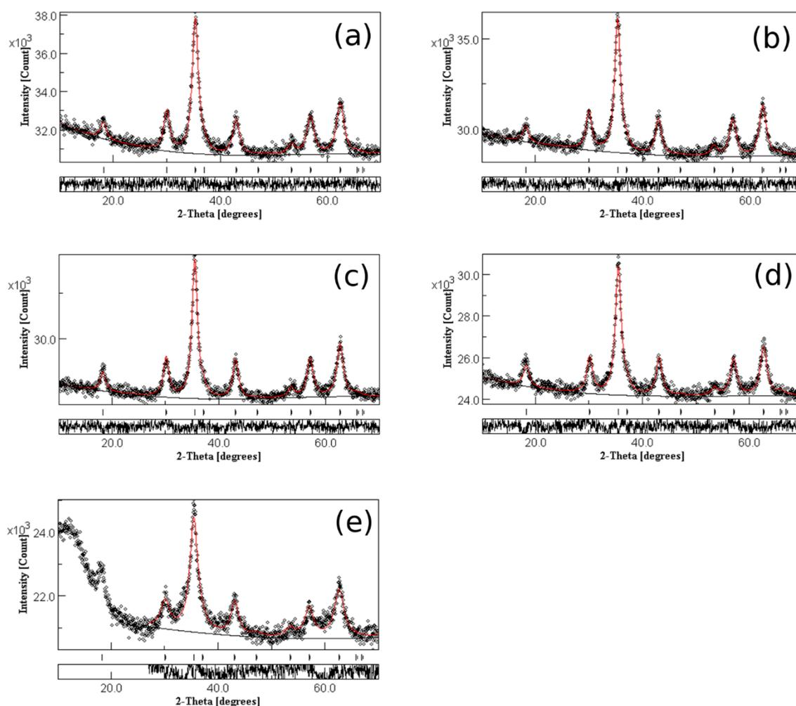
Figure S1. The XRD patterns and the respective fits from Rietveld refinement are reported for sample  $\text{Co}_{100}\text{-Ni}_0$  (a),  $\text{Co}_{75}\text{-Ni}_{25}$  (b),  $\text{Co}_{50}\text{-Ni}_{50}$  (c),  $\text{Co}_{25}\text{-Ni}_{75}$  (d) and  $\text{Co}_0\text{-Ni}_{100}$ . The experimental data are represented as open circles, the background as a black line and the fit as a red line.
