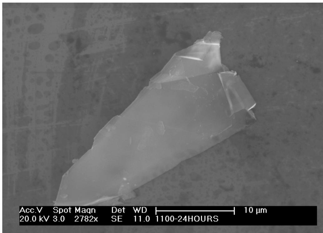
Figure S1: SEM image of the exfoliated graphane after 2 hours of electrolysis
