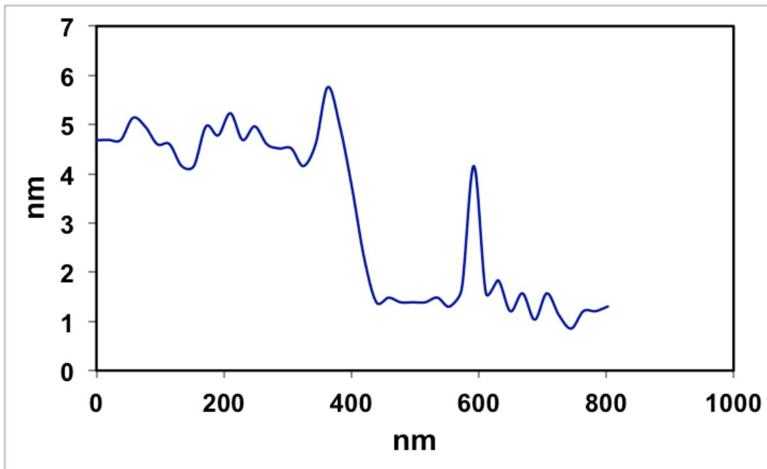
Figure S5: AFM image and height profile across the line giving clear evidence of the exfoliation to multilayer graphene after 3 hours of the electrolysis. In average, the thickness of the flakes gets thinner by increasing the electrolysis time as can be concluded from comparing Figure S5 and Figure 7 in the manuscript.
