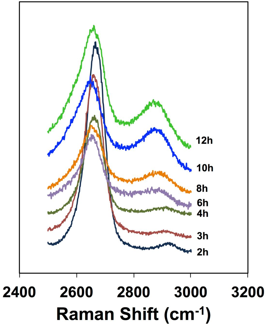
Figure S6: Raman spectra recorded using the 633 nm laser, showing the development of the G+D band as a function of the process duration.
