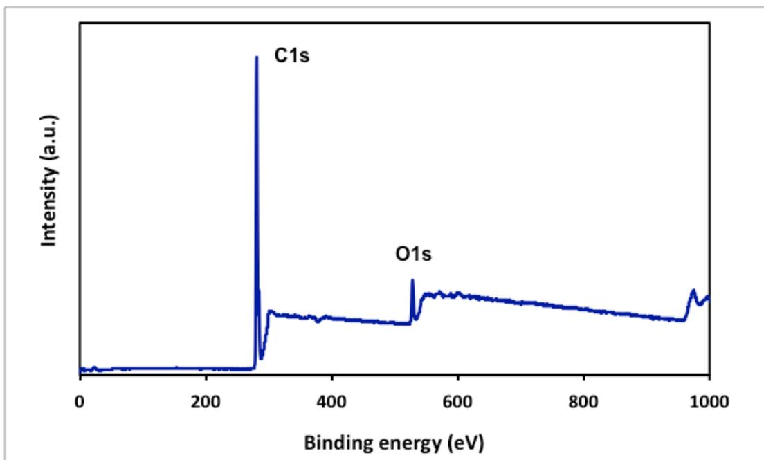
Figure S7: Wide scan XPS for the sample hydrogenated for 12 hours at 2.5 V in urea-choline chloride eutectic mixture. Showing almost no oxygen content.
