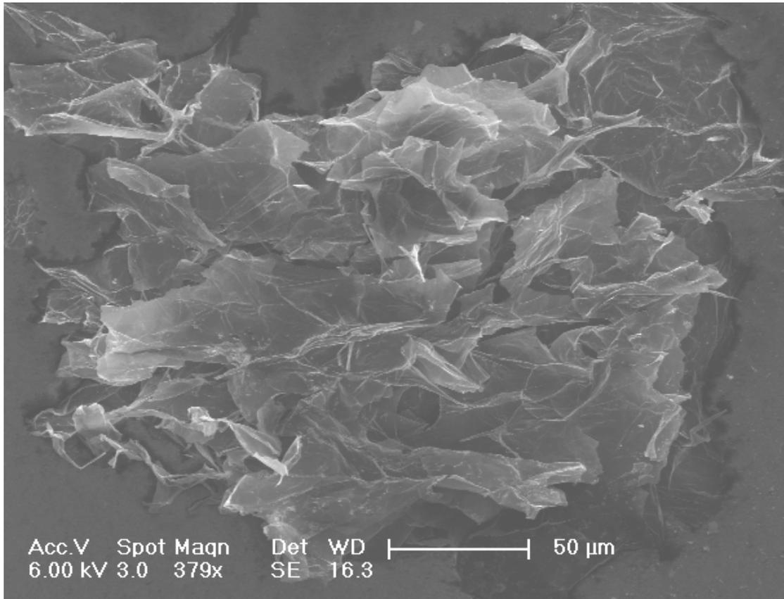
Figure S2: after 6 hours of electrolysis the flakes tend to agglomerate together in a porous structure
