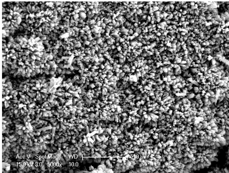
Figure 5. SEM image of the \text{Ti}^{+3} - \text{TiO}_2 .
