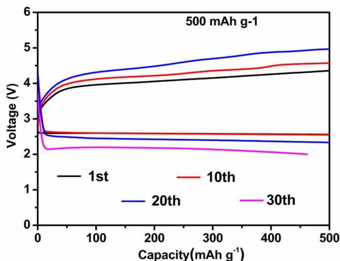
Fig. S11. Cyclic performance of the VX-72 carbon electrode at 0.16 mA cm<sup>-2</sup> with limited capacity of 500 mAh g<sup>-1</sup>.
