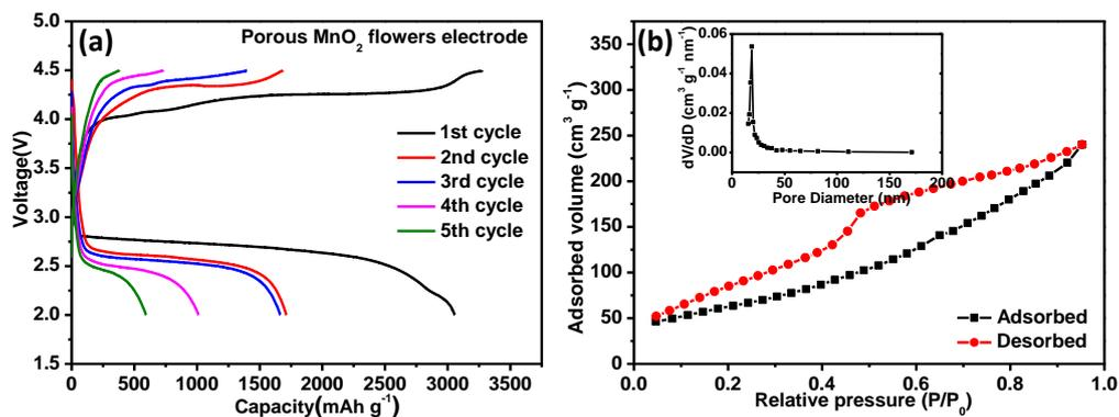
Fig. S10. (a) Discharge-charge curves of Li-O<sub>2</sub> batteries with hierarchical porous  $\delta$ -MnO<sub>2</sub> nanoboxes electrode at 0.16 mA cm<sup>-2</sup>; (b) Nitrogen adsorption-desorption isotherms and pore size distribution (inset) of the flower-like  $\delta$ -MnO<sub>2</sub>. The BET surface area is about 229.6 m<sup>2</sup> g<sup>-1</sup> and the pore volume is 0.340 cm<sup>3</sup> g<sup>-1</sup>
