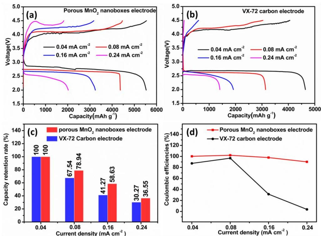
**Fig. S6.** First discharge-charge curves of Li-O<sub>2</sub> batteries with (a) hierarchical porous  $\delta$ -MnO<sub>2</sub> nanoboxes and (b) VX-72 carbon electrodes at various current densities; (c) Discharge capacity retention of Li-O<sub>2</sub> battery cells with different electrodes at various current densities; (d) Coulombic efficiency of Li-O<sub>2</sub> batteries with different electrodes at various current density.
