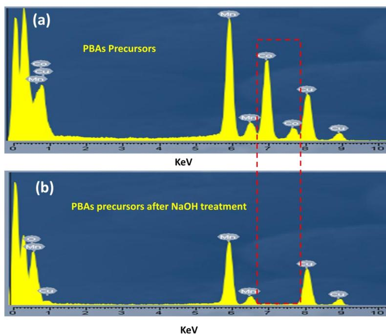
**Fig. S3.** EDX spectra of the PBAs precursors (a) before and (b) after the NaOH treatment.
