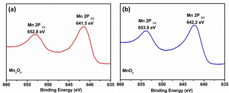
**Fig. S4.** XPS survey of (a) porous Mn<sub>3</sub>O<sub>4</sub> nanoboxes and (b) hierarchical porous δ-MnO<sub>2</sub> nanoboxes.
