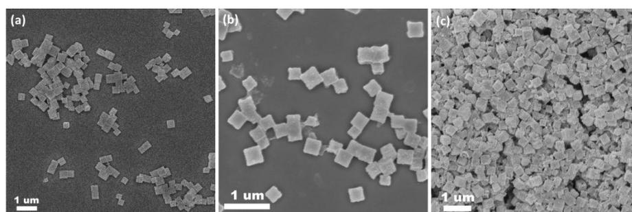
**Fig. S1.** SEM images of the obtained (a) nanocube-like PBAs precursors, (b) porous  $\text{Mn}_3\text{O}_4$  nanoboxes and (c) hierarchical porous  $\delta\text{-MnO}_2$  nanoboxes.
