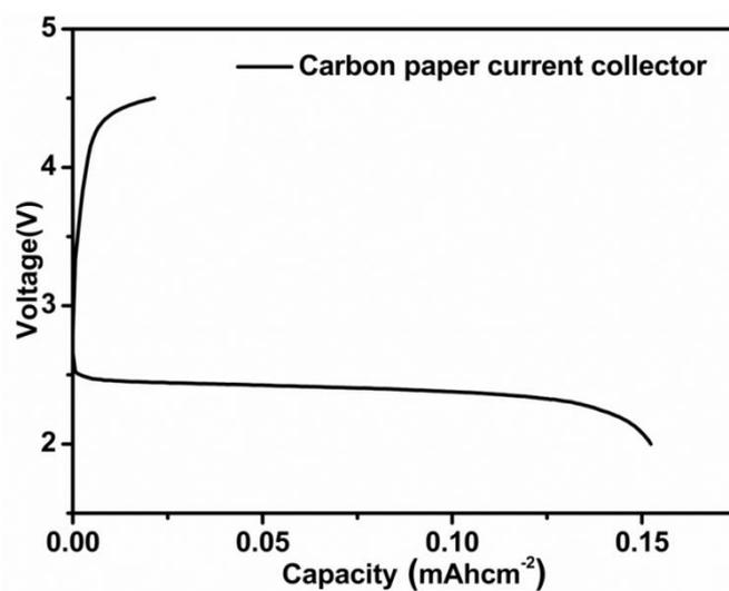
**Fig. S5.** Discharge-charge curves of Li-O<sub>2</sub> batteries with blank carbon paper current collector.
