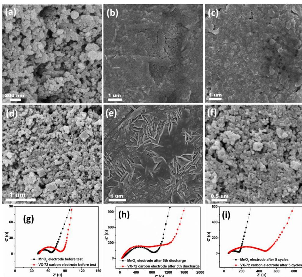
Fig. S9. SEM images of the VX-72 carbon electrode (a, b, c) and hierarchical porous  $\delta$ -MnO<sub>2</sub> nanoboxes electrode (d, e, f), before test (a, d), after 5<sup>th</sup> discharge (b, e) and after 5<sup>th</sup> charge (c, f); (g), (h), (i) electrochemical impedance spectra of Li–O<sub>2</sub> batteries with the hierarchical porous  $\delta$ -MnO<sub>2</sub> nanoboxes and VX-72 carbon electrodes at different discharge–charge states.
