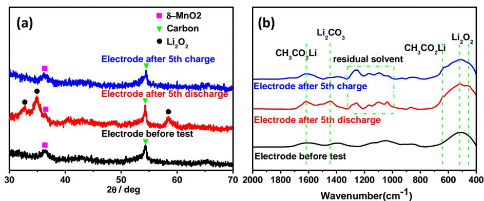
Fig. S8. (a) XRD pattern and (b) FTIR spectrum of the electrode at different states.
