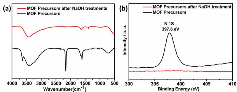
**Fig. S2.** (a) FT-IR and (b) N 1s XPS spectra of the PBAs precursor before (black) and after (red) NaOH treatment.
