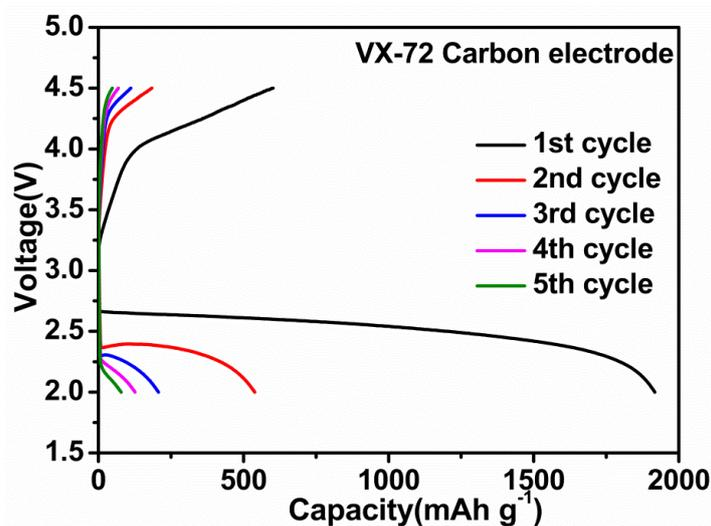
**Fig. S7.** Discharge-charge curves of Li-O<sub>2</sub> batteries with VX-72 carbon electrode at 0.16 mA cm<sup>-2</sup>.
