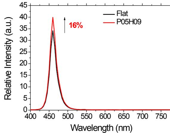
**Fig. S2** Emitted spectra from the LED without packaging phosphor in the absence and presence of the inverted pyramid structure on the surface of the PDMS encapsulation layer.
