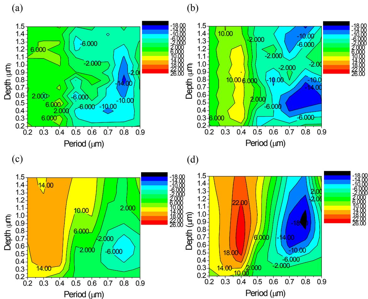
**Fig. S1** Contour diagrams of the simulated light extraction efficiency enhancements at a wavelength of 455 nm for (a) nanorods, (b) inverted rods, (c) pyramids, and (d) inverted pyramids having periods ranging from 200 to 900 nm and depths ranging from 200 to 1500 nm.
