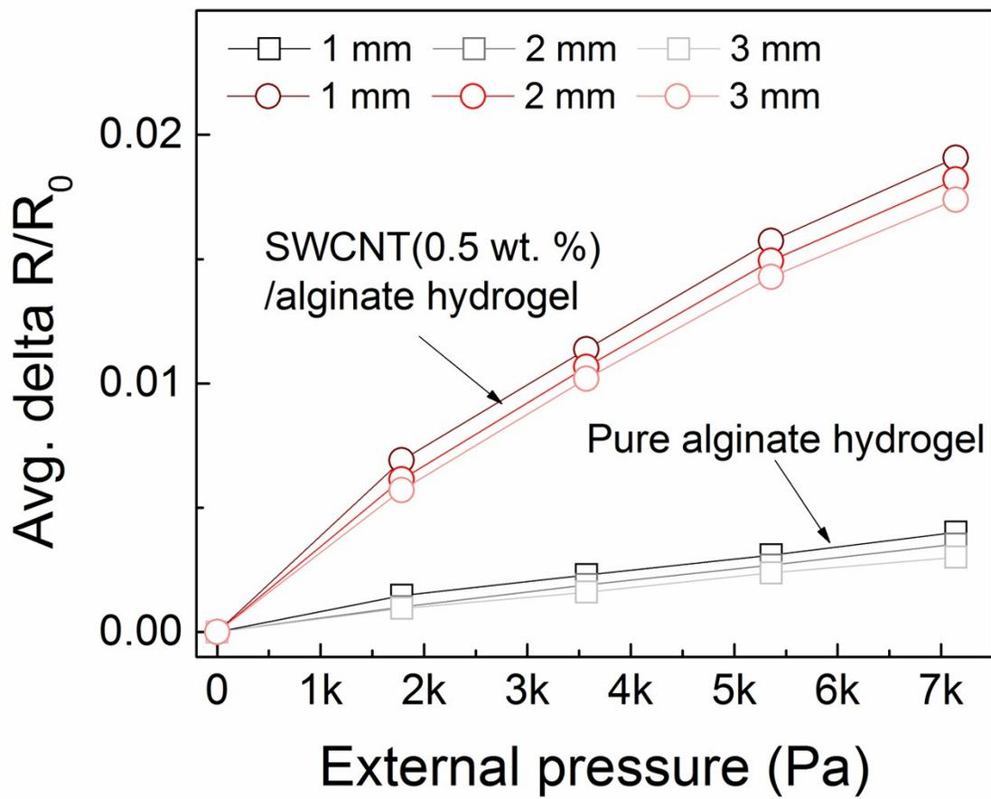
Fig. S3 Total resistance variation as a function of external loading with different alginate cylinder lengths (1 mm, 2 mm, 3 mm). Gold-coated wafer served as the electrodes; the cylinder sample had a diameter of 3 mm.
