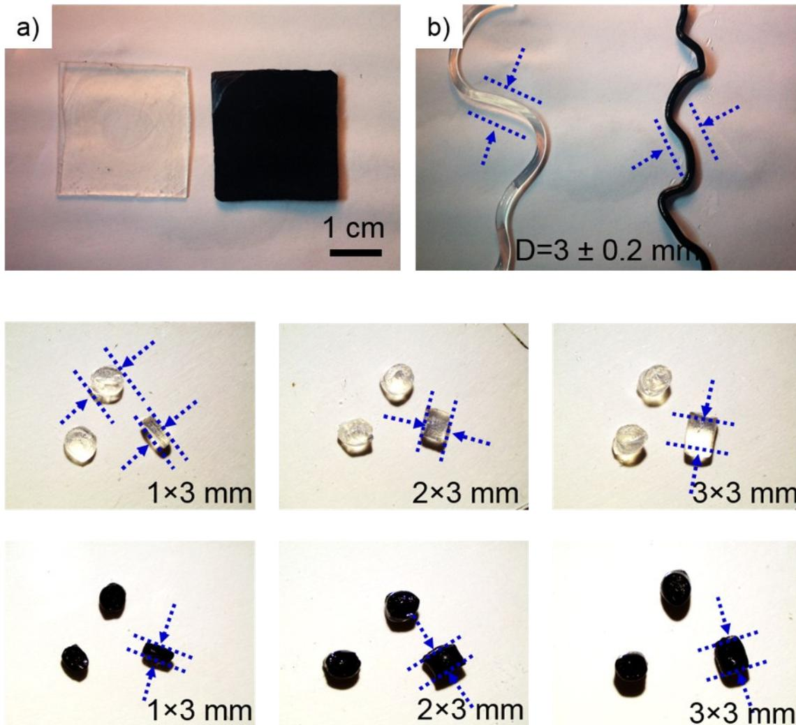
Fig. S1 Alginates-based hydrogels with different geometries. a) An alginates hydrogel film, b) a hydrogel thread made of cylinders  $3 \pm 0.2$  mm in diameter, c) and d) hydrogel cylinders of different lengths cut from the hydrogel thread. Transparent samples are alginates hydrogels, while black samples are SWCNT/alginates hydrogels with a SWCNT concentration of 0.5 wt. %.
