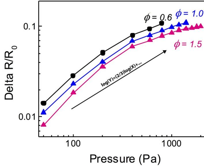
Fig. S6 Change in resistance as a function of pressure in log-log scale.
