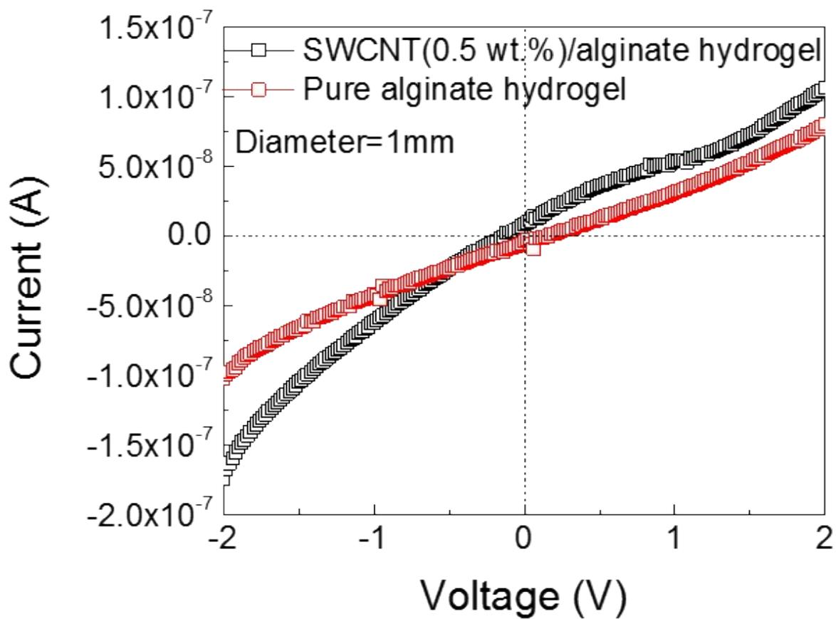
Fig. S2 I-V curves of the as-prepared pressure sensor with pure alginate sphere and SWCNT (0.5 wt. %)/alginate sphere (sensing sphere diameter is 1 mm).
