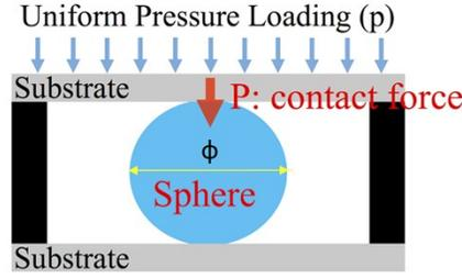
Fig. S4 A schematic of the system.  $p$  is the external applied pressure and  $P$  is the contact force at the sphere/electrode interface.
