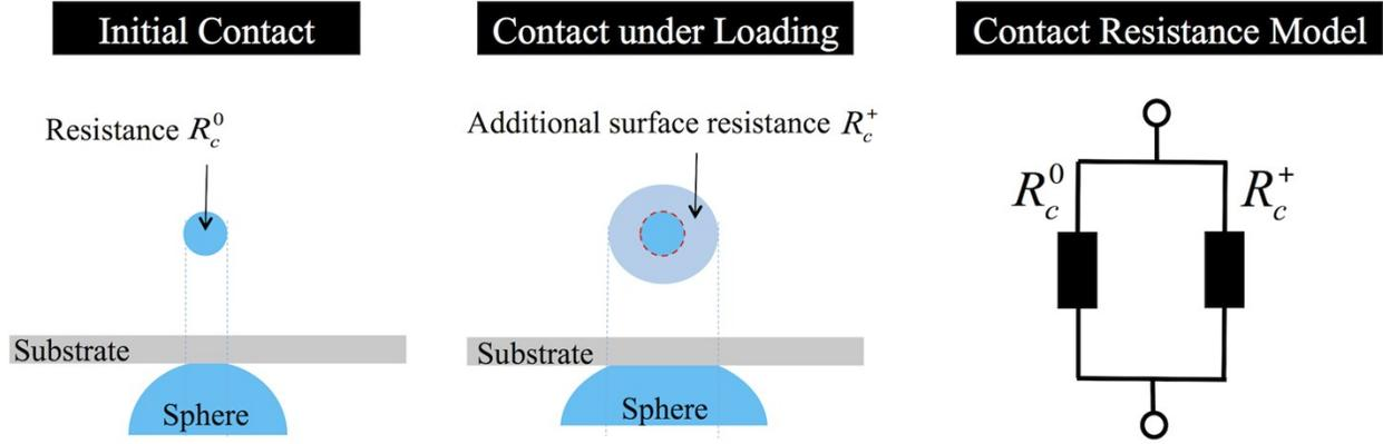
Fig. S5 Decomposition of the contact resistance.
