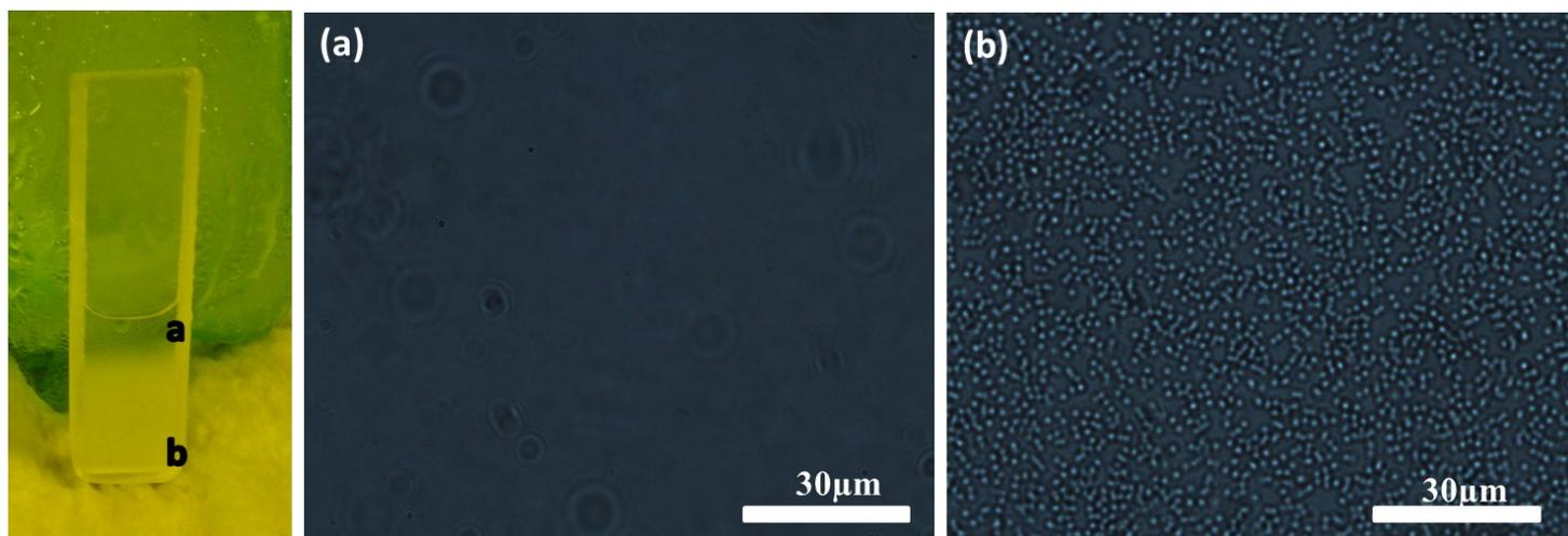
Fig. S4. Optical microscope images of the dispersion in (a) upper solution and (b) bottom solution. It can be seen from the image that after precipitation, most of the SiO<sub>2</sub> micro-beads resides in the bottom where the solution looks opaque. On the other hand, the upper part is free of the SiO<sub>2</sub> micro-beads and looks transparent.
