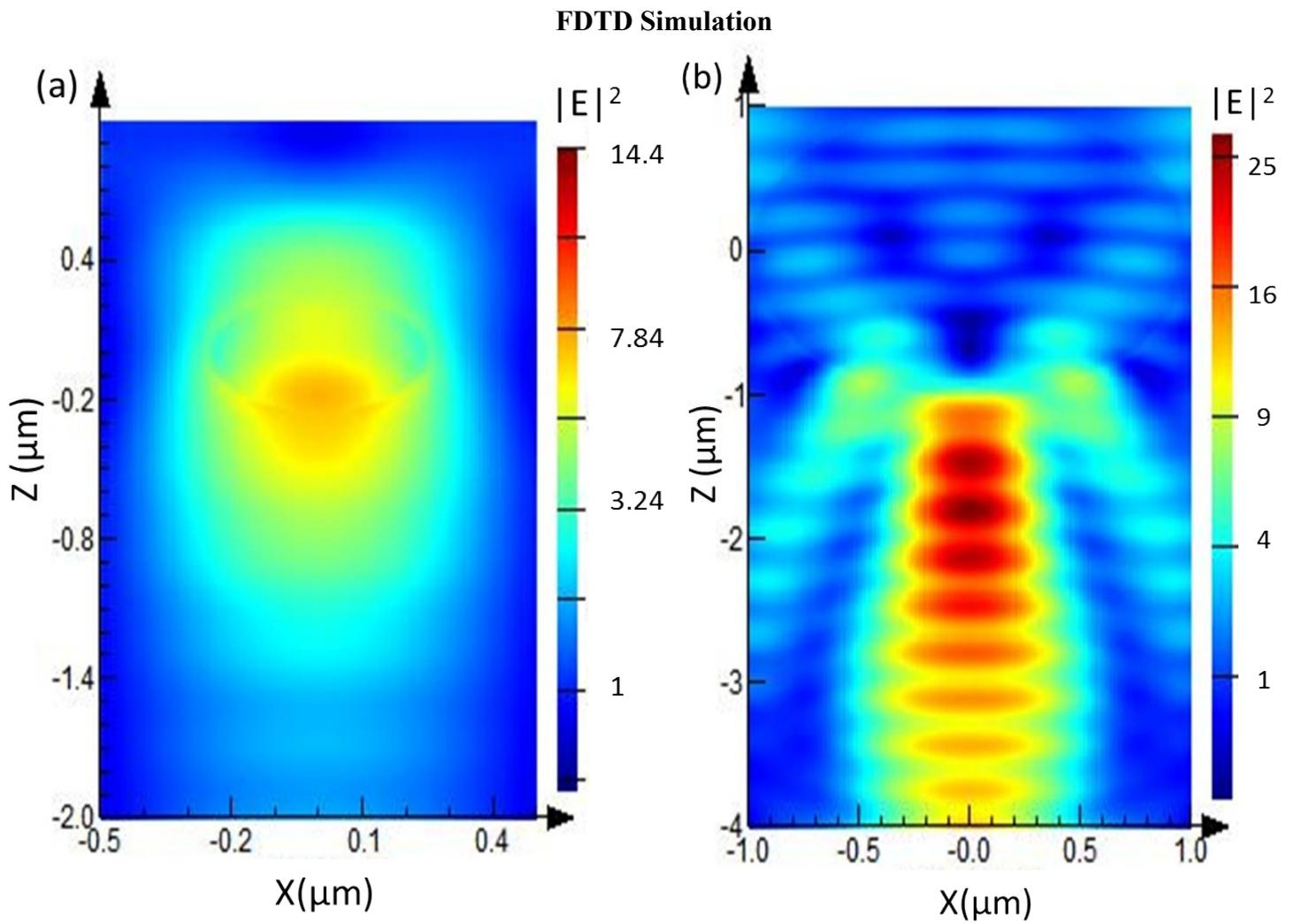
Fig. S2. FDTD simulation results for  $\text{SiO}_2$  micro-bead with (a) 500 nm and (b)  $2\mu\text{m}$  diameters in frozen matrix (ice)
