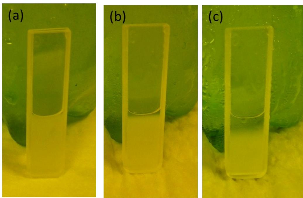
Fig. S3. Optical image for the SiO<sub>2</sub> micro-bead dispersion at the precipitation time of (a) 4 minutes, (b) 10 minutes, and (c) 60 minutes
