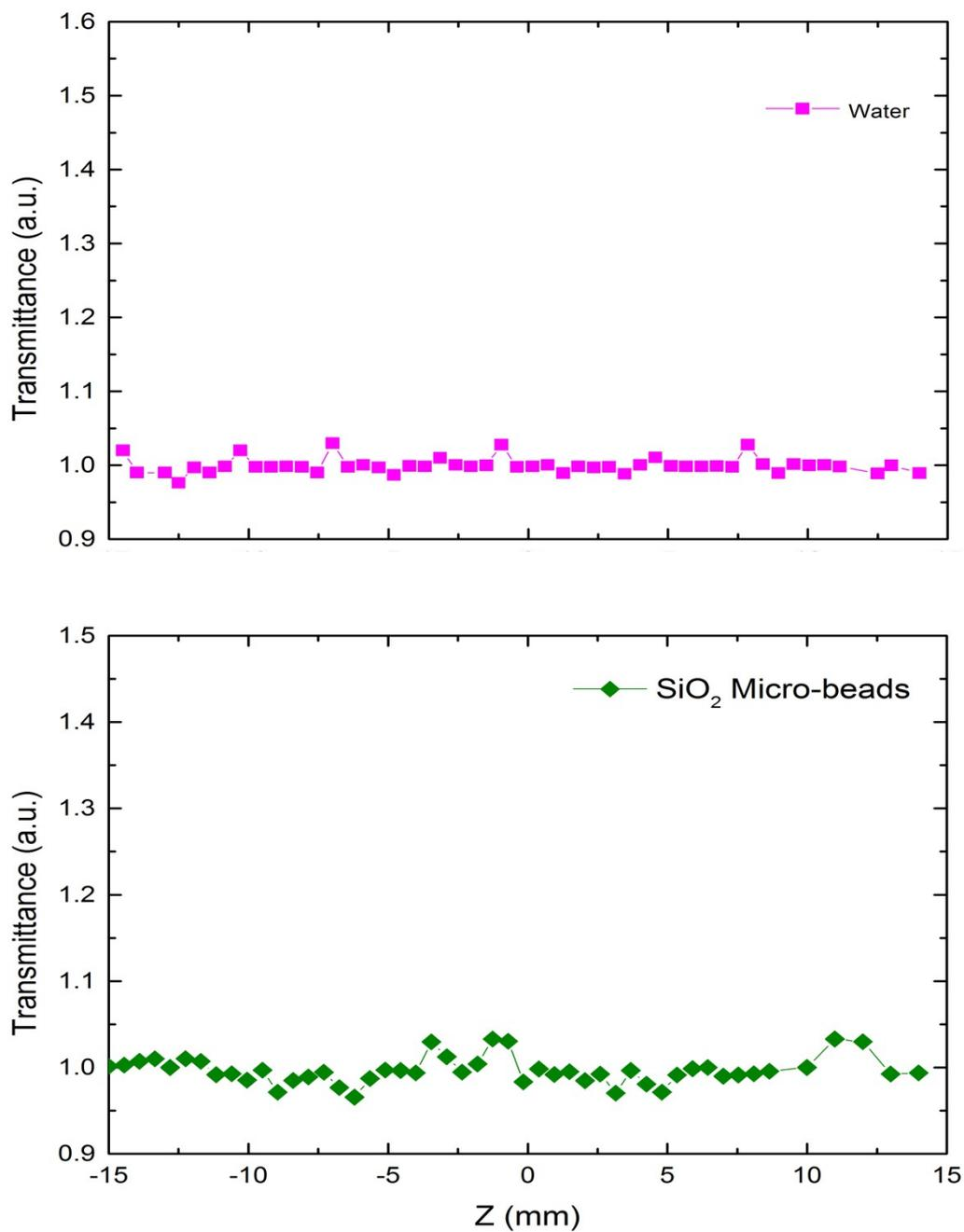
Fig. S5. Open aperture Z-scan results for the (a) water and (b) SiO<sub>2</sub> micro-beads
