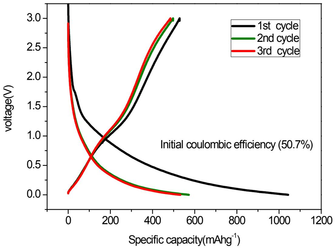
**Figure S7** Charge-discharge curves of pristine GNS.
