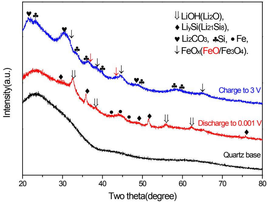
**Figure S4** XRD of the hybrid anodes after 2<sup>nd</sup> cycles. The anodes were composed of 75% hybrids, 15% acetylene black, and 10% PVDF. After 2<sup>nd</sup> charged to 3V or discharged to 0.001V, the anodes were removed from batteries and dried in the Ar gas glove box, finally placed on quartz glass for XRD testing.
