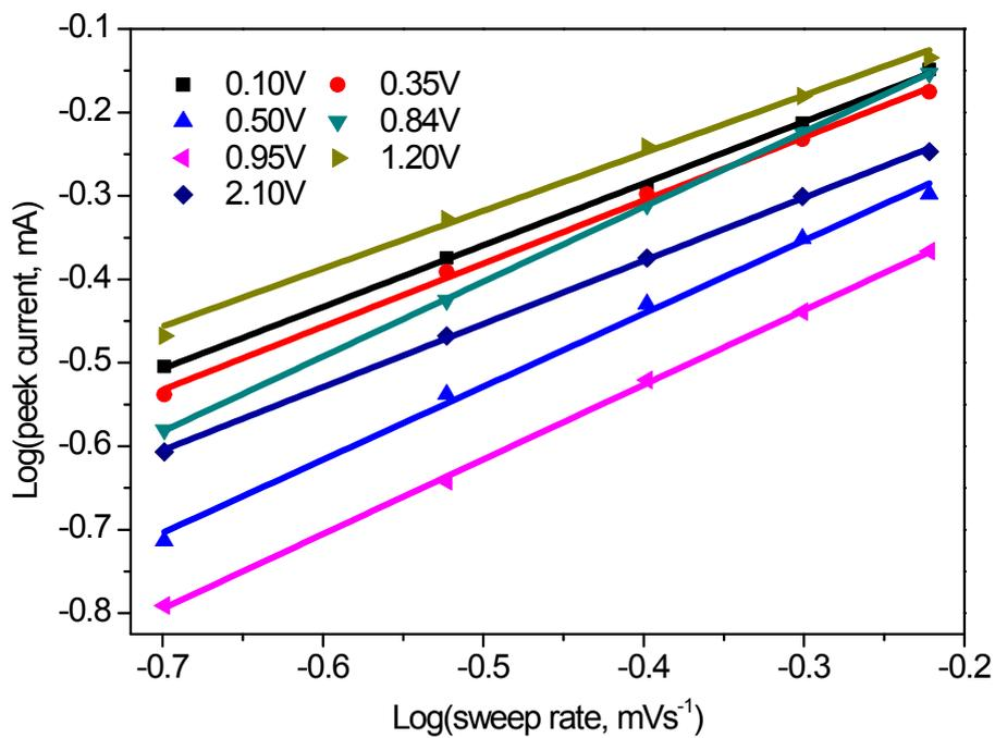
**Figure S5** Slope of the peak current versus the potential scan rate in a logarithm scale at different anodic and cathodic peaks position.
