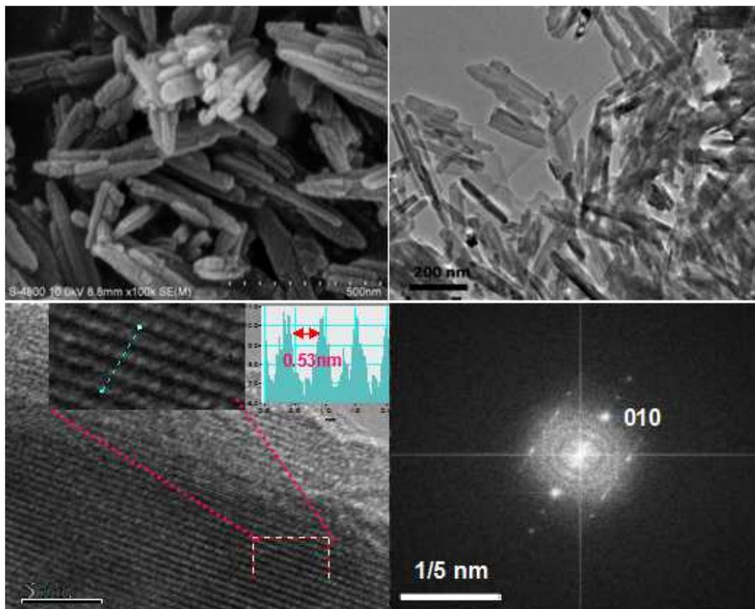
**Figure S1** SEM and TEM images of pristine LFSNR obtained at hydrothermal process.
