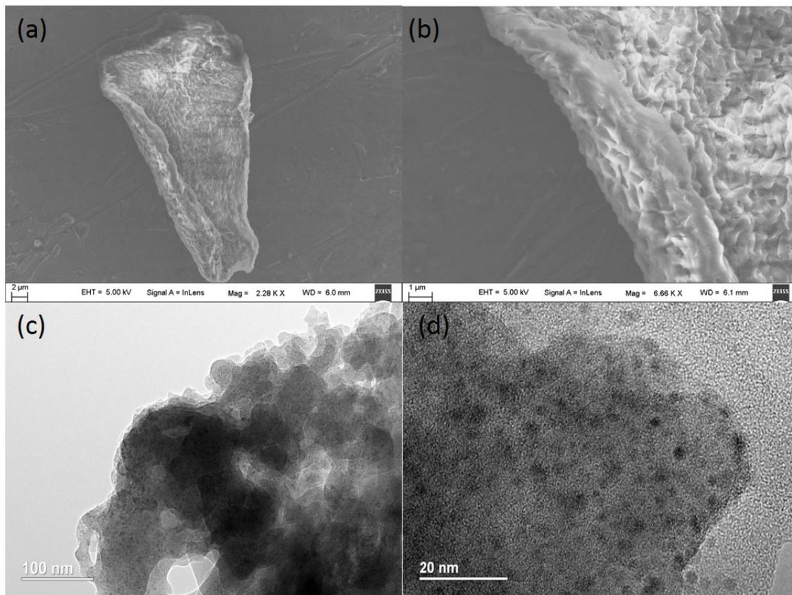
Figure S10 (a, b) SEM and (c, d) HRTEM images of the nanocomposites after 100 cycles.
