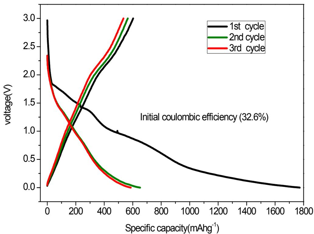
**Figure S8** Charge-discharge curves of pristine LFSNR.
