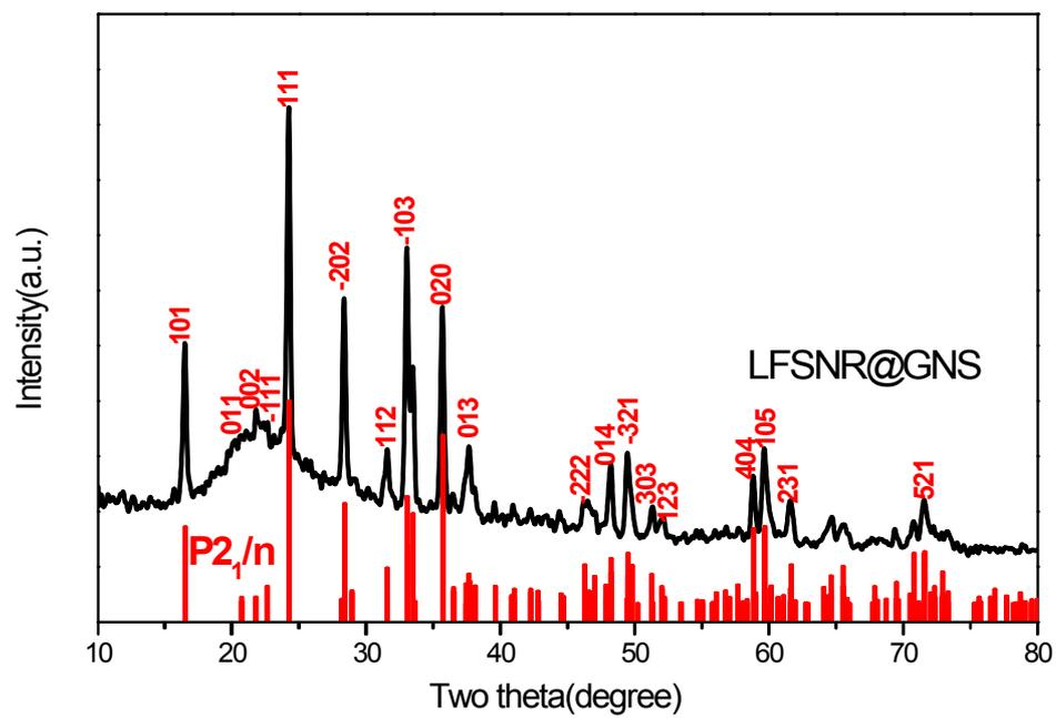
**Figure S3** XRD of the LFSNR@GNS hybrid.
