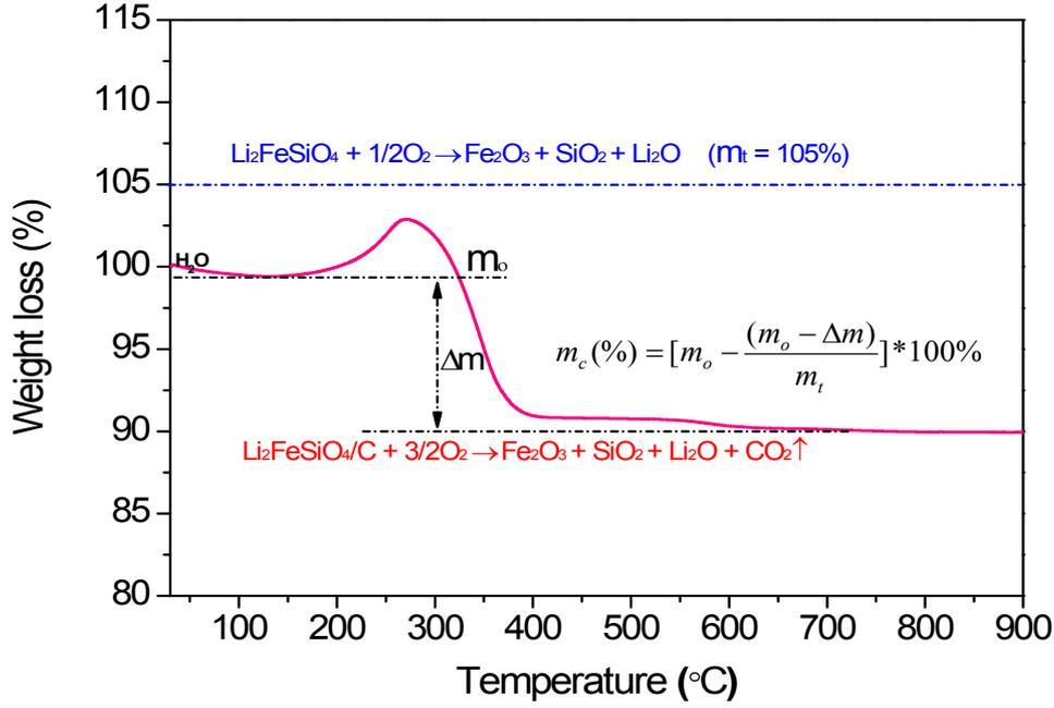
**Figure S6** TG curve of the LFSNR@GNS. The amount of carbon released from the sample was measured using TG method (Fig. S5) within a temperature range of room temperature to 900 °C under O<sub>2</sub> flow. The oxidation of samples under O<sub>2</sub> can be carried out on the basis of the reactions (S1) and (S1):
