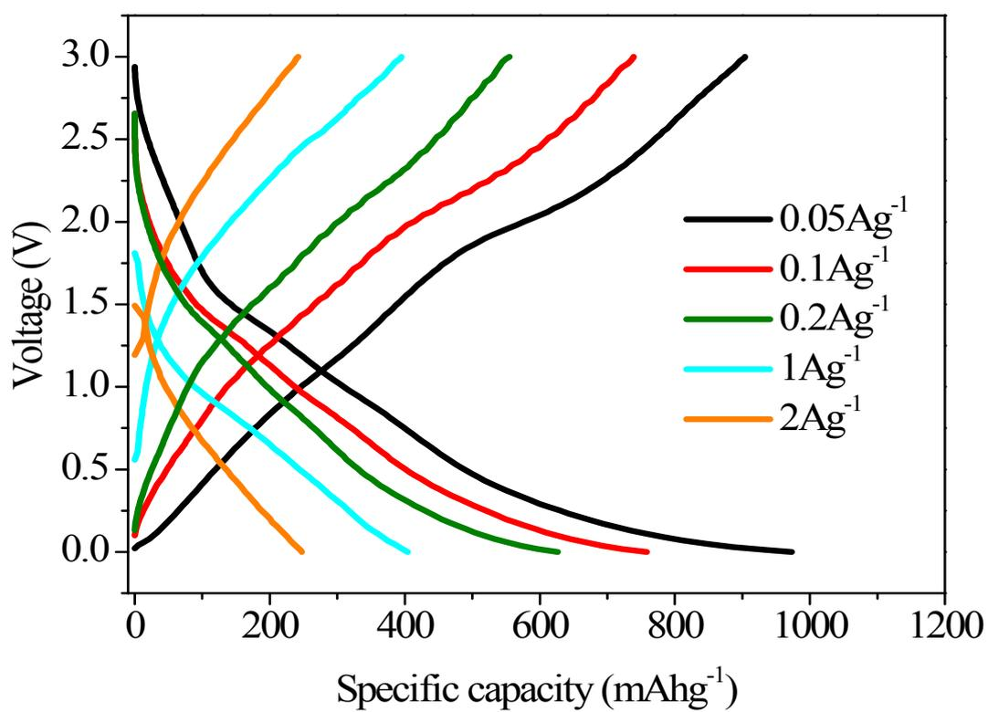
**Figure S9** Typical charge-discharge curves at various current densities between 0.001-3 V for the hybrid.
