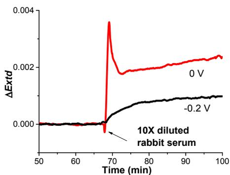
**Fig. S5.** Real-time monitored  $\Delta Ext_d$  upon the injection of 10× diluted rabbit serum on the peptide-modified AuNH array under bias of 0 V and -0.2V.
