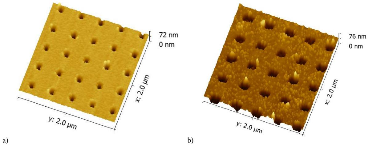
**Fig. S2.** AFM imaging of the AuNH array a) before and b) after 30-min incubation of 3 µg/ml cTnI in PBS buffer under -0.2 V bias applied on the sensor chip.
