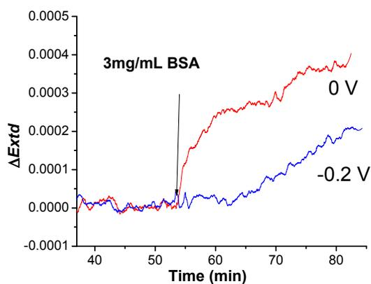
**Fig. S4.** Real-time monitored LSPR response ( $\Delta Ext_d$ ) to the incubation of 3 mg/ml BSA on the peptide-modified AuNH array under 0 V and -0.2V.
