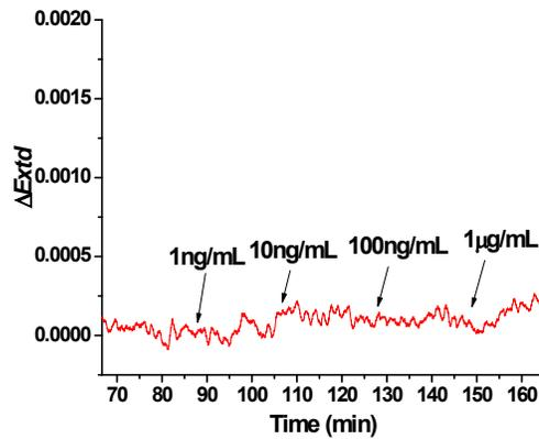
**Fig. S3.** LSPR response ( $\Delta Ext_d$ ) of the AuNH array modified by CALNN under no bias, after the injection of cTnI at the concentration of 1ng/mL, 10ng/mL 100ng/mL and 1µg/mL.
