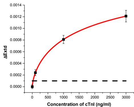
**Fig. S6.** Calibration curve for the detection of cTnI in 10× diluted rabbit serum. Dash line shows the noise level ( $3\sigma$ ).
