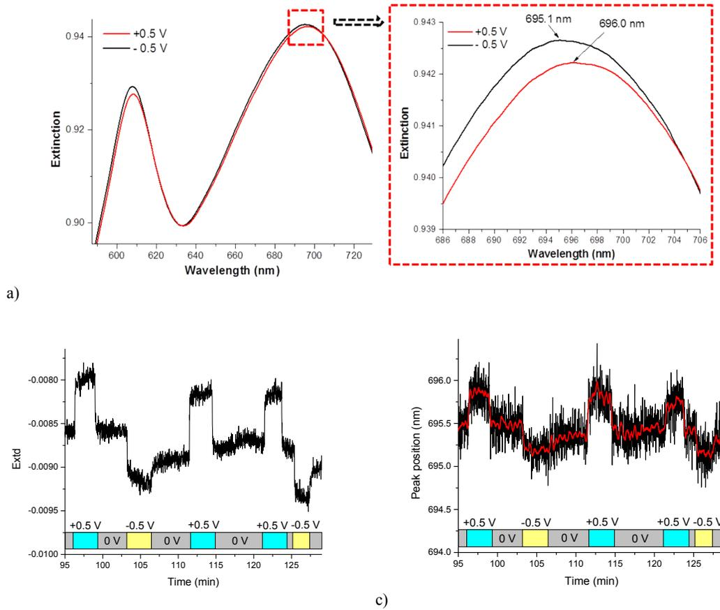
**Fig. S1.** a) Extinction spectra of the AuNH array applied with -0.5 V and +0.5 V biases. The time dependent b) extinction difference (ExtD) and c) peak position changes upon applying different biases on the sensor surface.
