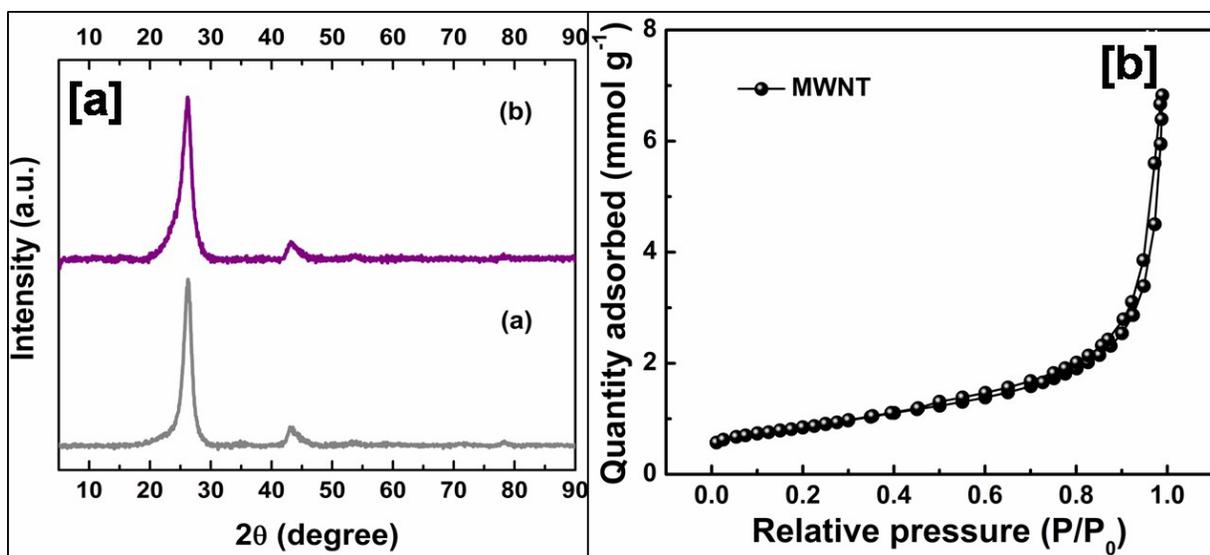
Fig. S3. [a] X-ray diffraction patterns of exfoliated multiwalled carbon nanotubes oxidized at (a) 10% and (b) 25% amount of  $\text{KMnO}_4$ . [b] Nitrogen adsorption-desorption isotherm for purified multiwalled carbon nanotubes giving SSA as  $\sim 66 \text{ m}^2 \text{ g}^{-1}$ .
