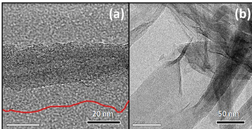
Fig. S4. TEM images of multiwalled carbon nanotubes exfoliated (a) least and (b) most amount of  $\text{KMnO}_4$ .
