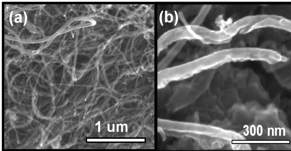
Fig. S5: Scanning electron microscopy images of (a) MWNT and (b) PENT.
