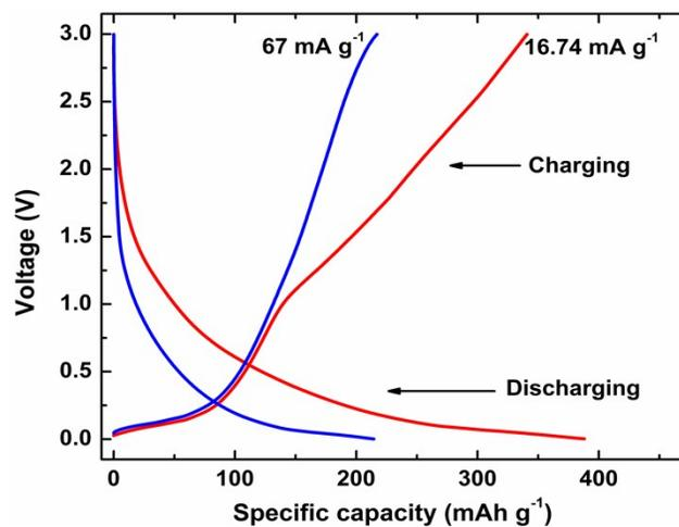
Fig. S1. Charge-discharge profile for multiwalled carbon nanotubes (MWNT).
