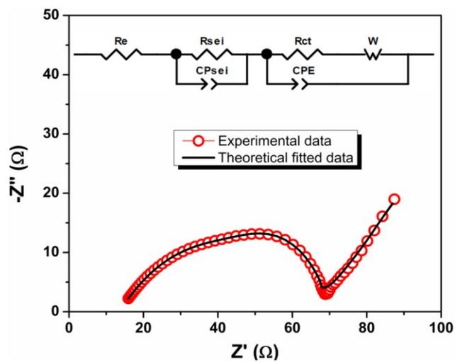
Fig. S2. Impedance spectra study from 100 kHz to 0.01 mHz with a sine wave of amplitude 5 mV.
