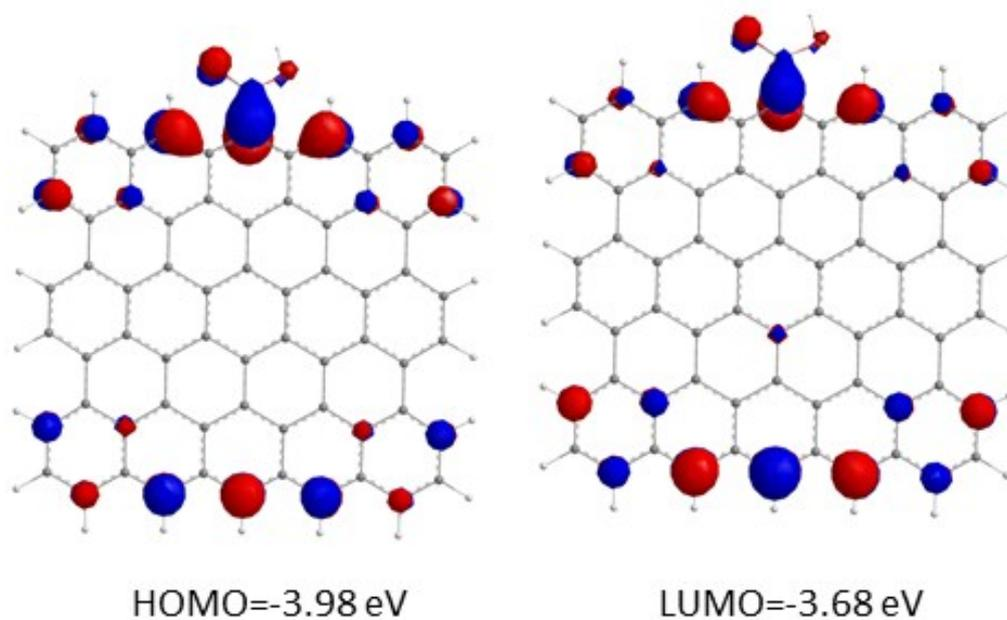
**Figure S8.** Frontier molecular orbitals (Isocontour 0.035) of model structure of GO with COOH group connected to the zig-zag edges. As can be seen the strongest localization of both HOMO and LUMO is calculated on the COOH defect of graphene sheet indicating the most reactive place in molecule.
