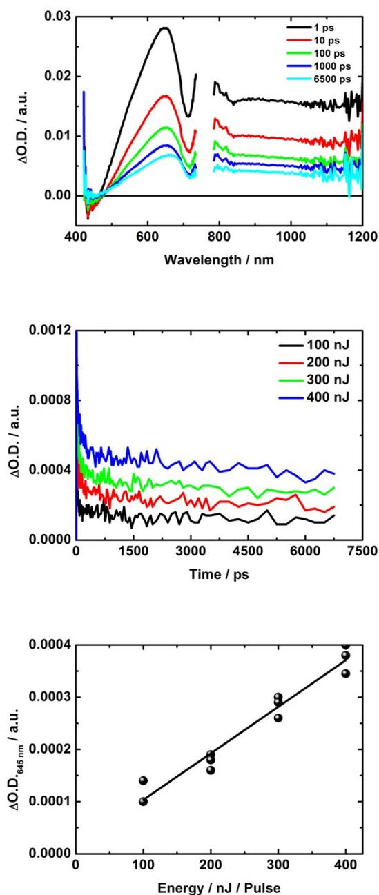
**Figure S6.** Upper part: Transient absorption spectra of CT-GO (0.2 mg / ml) in water upon fs-laser photolysis (256 nm / 400 nJ) with several time delays. Middle part: Corresponding time absorption profiles at 645 nm at different excitation energies ranging from 100 to 400 nJ / pulse) Lower part: Plot of the transient absorption obtained for the time delays 6250, 6500 and 6750 ps vs. the excitation energy. The black line represents the linear fit.
