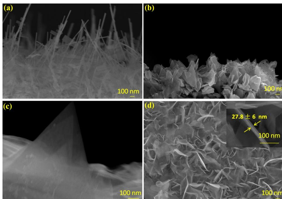
Fig. S1. SEM images side view for (a) WO<sub>3</sub> (b) rGO/ WS<sub>2</sub>, (c) magnified for rGO/ WS<sub>2</sub> and (d) top view for rGO/ WS<sub>2</sub>
