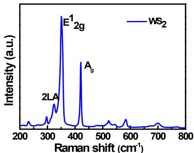
Fig. S4. Raman spectra of WS<sub>2</sub>.
