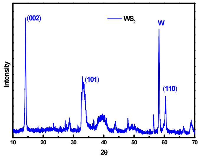
Fig. S3. XRD pattern of  $\text{WS}_2$
