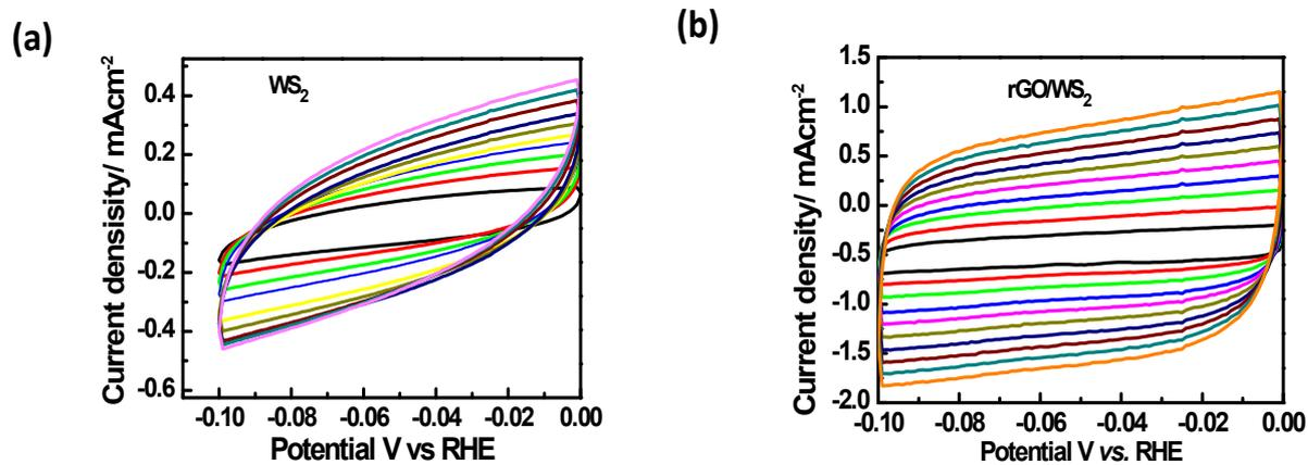
**Fig. S5** Voltammograms at various scan rates for estimation of  $C_{dl}$  of WS<sub>2</sub> (a) and rGO/WS<sub>2</sub>(b)
