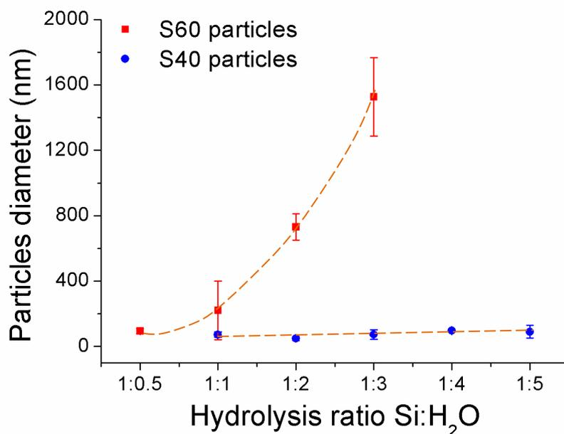
Figure S4. Comparison between the particles size of S40 and S60 particles prepared with different hydrolysis ratios.
