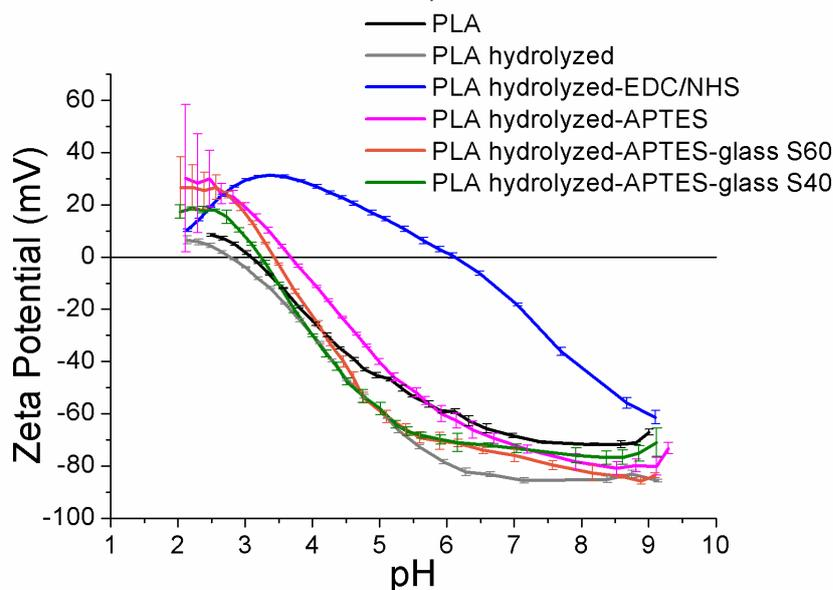
Figure S1. pH dependence of the zeta potential of the fibrous layer after the different surface treatments applied to perform the coating.
