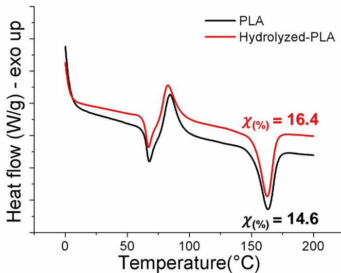
**Figure S10.** DSC thermograms of PLA and hydrolyzed-PLA fibers ( $\chi$ : percentage of crystallinity).
