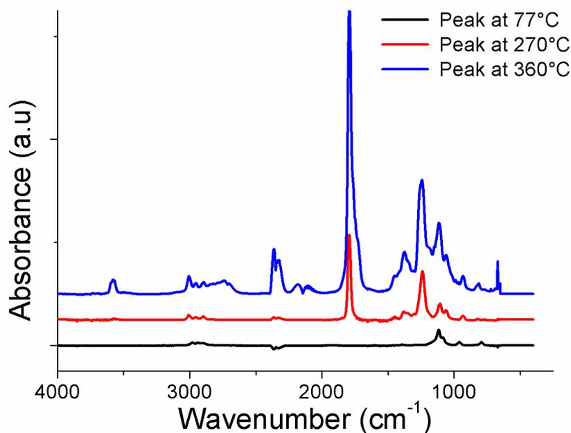
**Figure S6.** FTIR spectra of compounds vaporizing during the thermal degradation of PLA fibers coated with glass S60 at 77°C, 270°C and 360°C.
