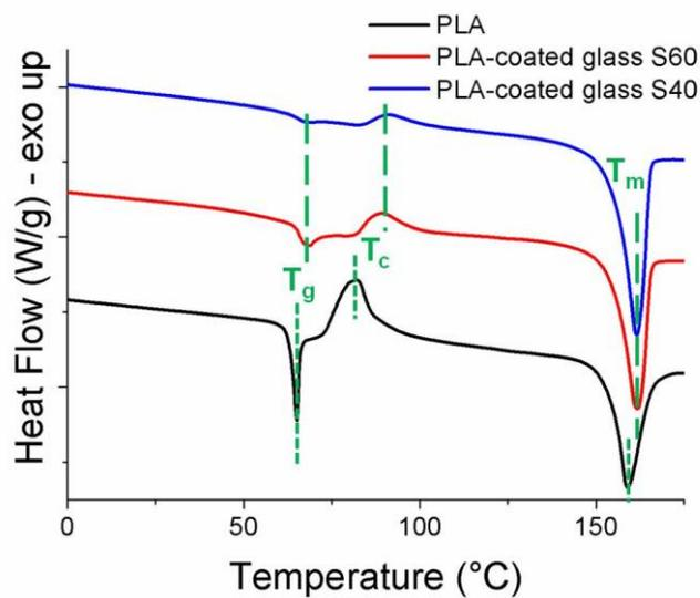
**Figure S8.** DSC thermograms of PLA and hybrid coated fibers.
