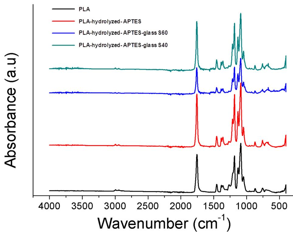
Figure S3. Full FTIR spectra obtained for the PLA fibers, hydrolyzed and APTES functionalized fibers, and coated fibers (S40 and S60).
