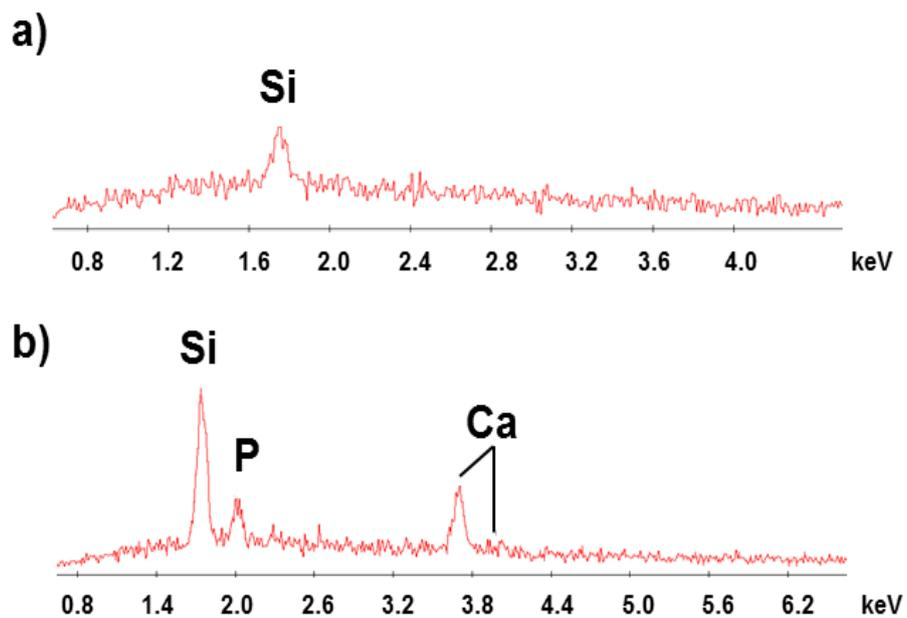
Figure S2. EDS spectra related to (a) APTES functionalized fibers and (b) coated fibers.
