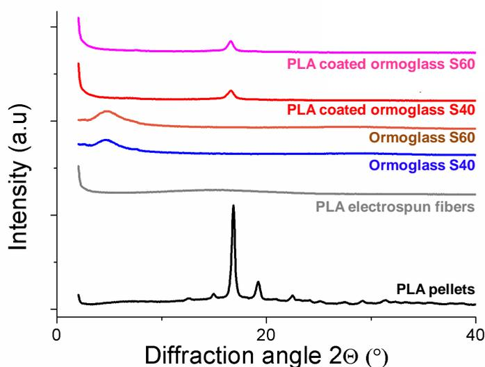
**Figure S9.** X-ray diffraction spectra of PLA pellets (pellets dissolved to obtain the polymeric solution for electrospinning – raw material), PLA electrospun fibers, S40 and S60 ormoglasses, and PLA fibers coated with both ormoglass compositions.
