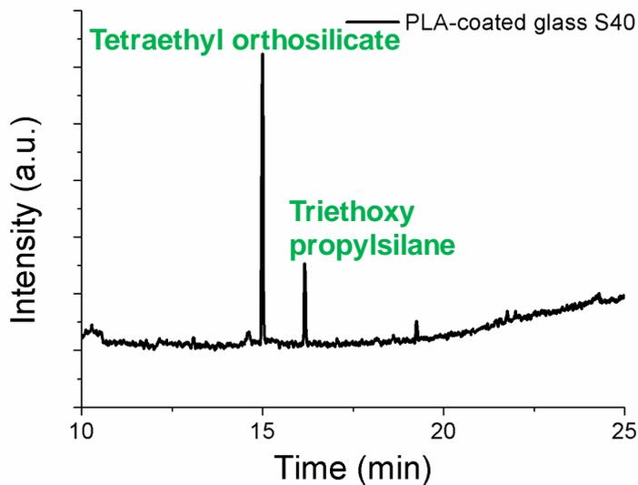
**Figure S7.** Gas chromatography pattern of fibers coated with S40 ormoglass, showing the presence of TEOS.
