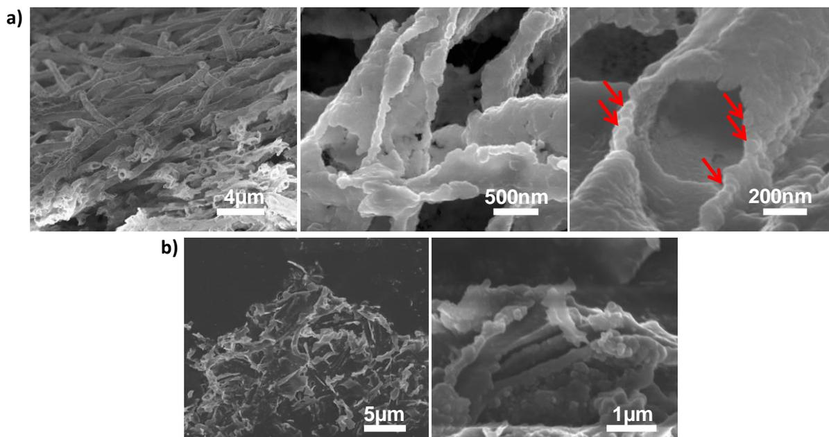
**Figure S5.** Morphology of (a) PLA fibers coated with the S60 ormoglass composition showing the particles monolayer (arrows) and the thickness of the coating after thermal treatment, and morphology of (b) PLA fibers coated with the S40 ormoglass composition showing the fragility and collapsing of the sample after thermal treatment.
