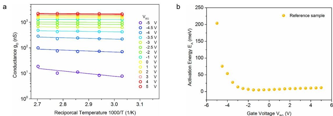
**Fig. S10.** (a) Arrhenius plot of the two-terminal conductance at various gate voltages. (b) The extracted activation energy data from (a). This reference sample was made by using PDMS transfer method and has the same device structure with Fig. 1a in Manuscript.
