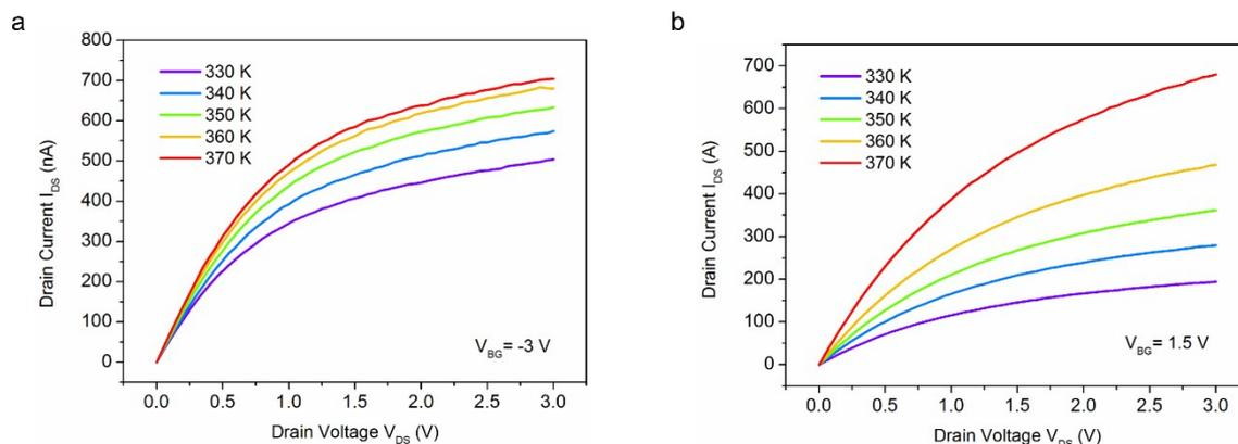
**Fig. S9.** Temperature-dependent transport characteristics for extraction activation energy. (a)  $I_{DS}$ - $V_{DS}$  curves for the bridge-channel FET at temperature range from 330 K to 370 K with near threshold voltage gate bias ( $V_{BG} = -3$  V). (b)  $I_{DS}$ - $V_{DS}$  curves for  $\text{SiO}_2$ -supported FET under the same condition ( $V_{BG} = 1.5$  V).
