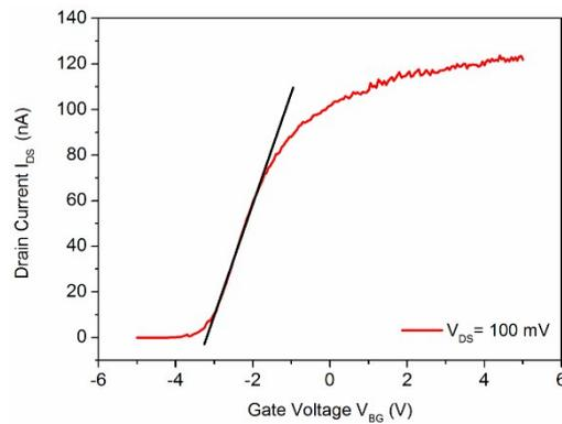
**Fig. S5.** Threshold voltage determination at low drain voltage ( $V_{DS} = 100$  mV) for the bridge-channel FET by using the linear extrapolation method.
