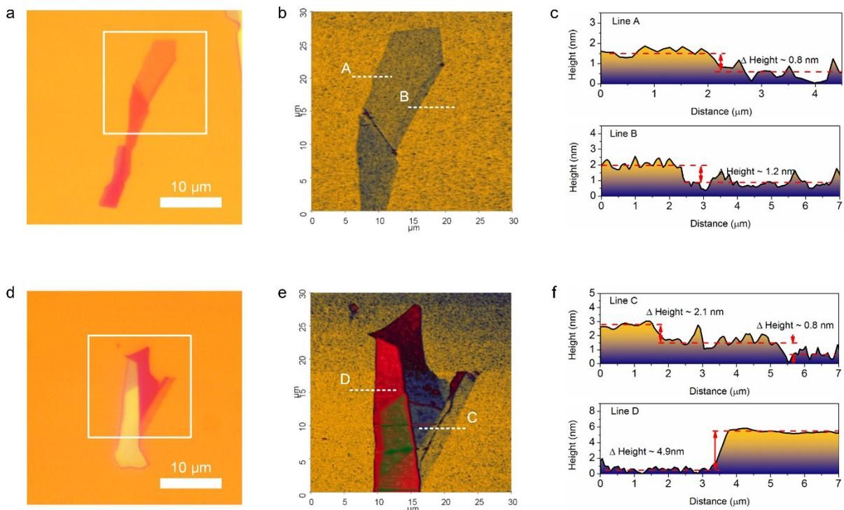
**Fig. S1.** (a) Optical image of MoS<sub>2</sub> flake deposited on 280-nm-SiO<sub>2</sub>/Si substrate. (b) AFM image of the selected area (white box). (c) The corresponding height profiles along the line A (top) and B (bottom). (d)-(f) are optical image, AFM image, and cross-section profile, respectively.
