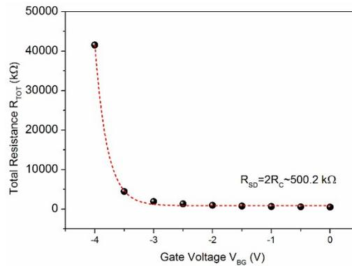
**Fig. S6.** The total resistance,  $R_{TOT}$  as function of gate voltage  $V_{BG}$ .
