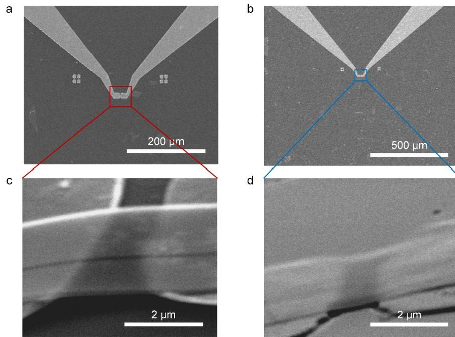
**Fig. S4.** (a)-(b) SEM images of two MoS<sub>2</sub> transistors with bridge-channel and corresponding magnified SEM images of the selected area (c)-(d).
