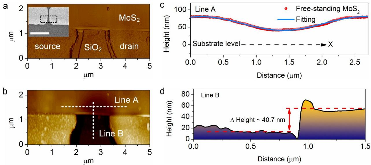
**Fig. S3** (a) phase image and (b) AFM topography of the selected area of a device corresponding to the highlighted area in inset of (a) (Inset: low magnification SEM image. Scale bar is  $10 \mu\text{m}$ ). The dashed lines labeled by A and B are perpendicular to each other. The corresponding height profile of the line A and B are given in (c) and (d). Note that the y-axis of (c) and (d) is in nanometer unit.
