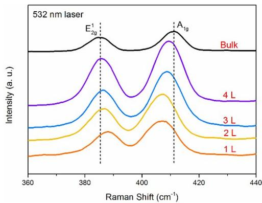
**Fig. S2.** Raman spectra of various thicknesses (one- to four-layer and bulk) of exfoliated MoS<sub>2</sub> using 532nm laser.
