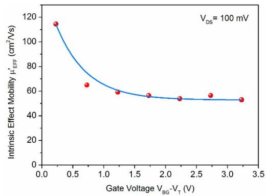
**Fig. S7.** Intrinsic effective mobility as function of  $(V_{BG}-V_T)$  extracted from Equation 1 in Manuscript. The intrinsic effective mobility of the bridge-channel transistor under low drain bias ( $V_{DS}= 100 \text{ mV}$ ) to make FET operating at linear regime.
