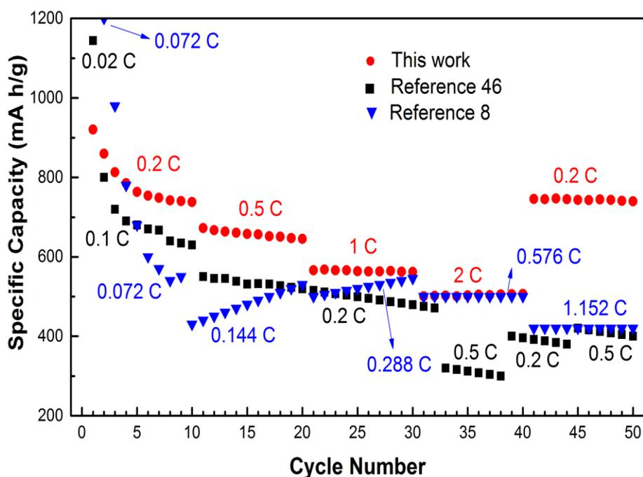
**Figure S5.** Rate capacity comparison between this work and other references. Black squares and blue triangles correspond to Reference 46 and Reference 8, respectively, whereas the red dots are this work's results.
