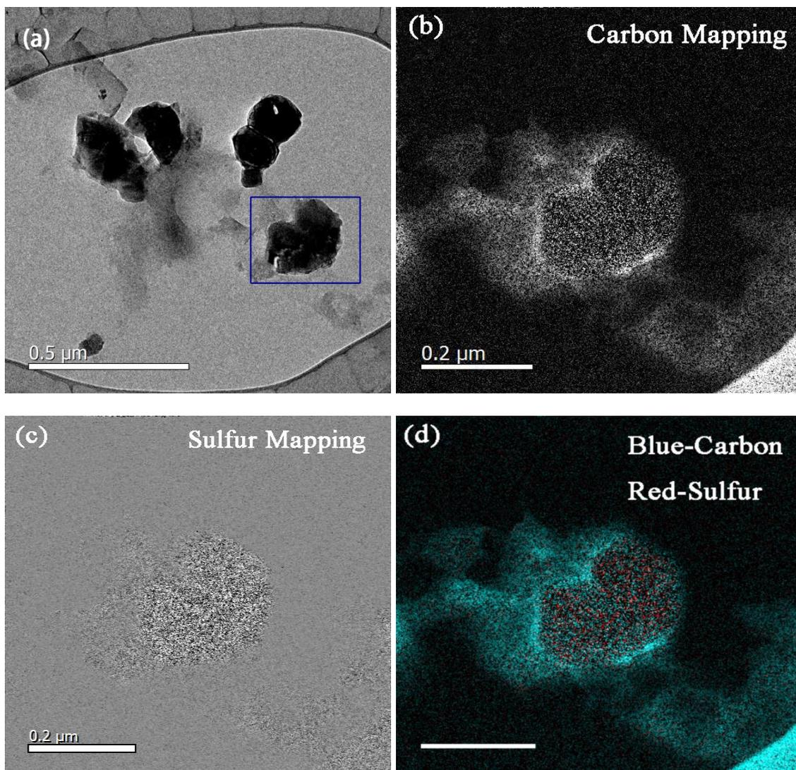
**Figure S2.** (a) FETEM image of nanoLi<sub>2</sub>S@C; the nanoparticle within blue circle is used for EFTEM elemental mapping, (b) Carbon mapping, (c) Sulfur mapping, (d) Combined elemental mapping, Scale bar: 200 nm.
