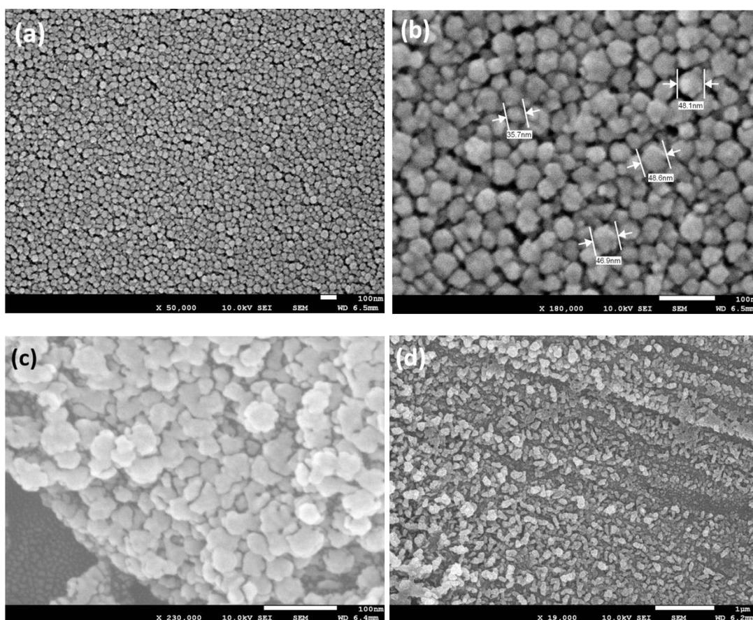
**Figure S1.** (a-b) FESEM images of polystyrene (PS) dispersed in aqueous solution from Nanocs, (c) FESEM image of PS after freeze-drying, (d) FESEM image of nanoLi<sub>2</sub>S@C.
