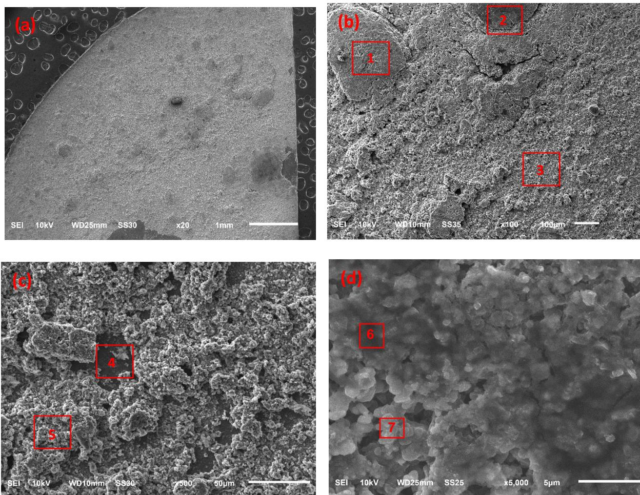
**Figure S4.** SEM images of a nanoLi<sub>2</sub>S@C-based cathode after 200 charge/discharge cycles at 0.2 C with different magnifications. The red boxes with numbers in (b), (c) and (d) show the locations where EDS data were collected.
