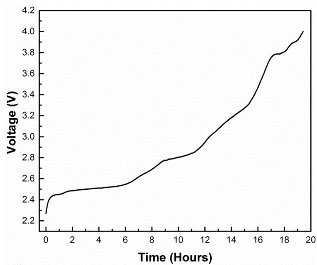
**Figure S3.** First charge profile for activation of  $\text{Li}_2\text{S}$ .
