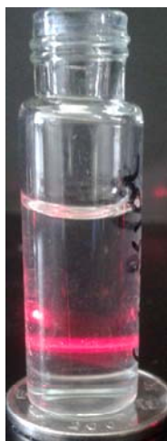
Figure S6. Tyndall effect of the 4-fold diluted incubation mixture of 1 at 1 wt% after 12 h incubation with 300 U/mL alkali phosphatase at 37 °C and pH 8.5 excited by laser light.
