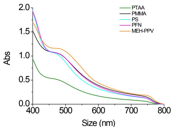
**Figure S5.** UV-vis spectra of MAPbI<sub>3</sub>:polymer mixtures thin films.
