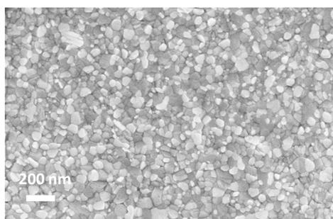
**Figure S6.** SEM image of MAPbI<sub>3</sub> film deposited on PEDOT:PSS.
