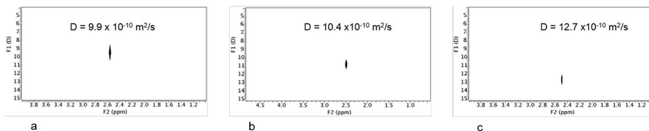
**Figure S1.** Expansion of DOSY maps (600 MHz, THF/DMF/DMSO 3:3:1:1, 298 K) of  $P_3$  at different concentration: 184 mM (a), 10 mM (b) and 2 mM (c).
