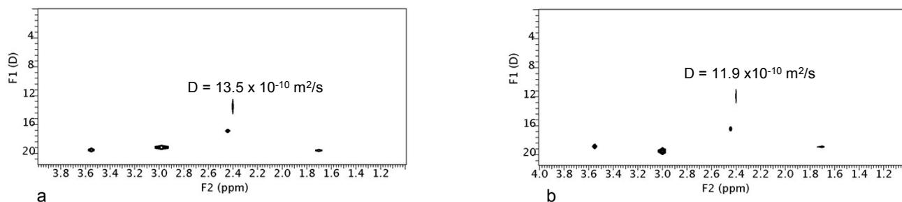
**Figure S3.** Expansion of DOSY maps (600 MHz, THF/DMSO 5:2, 298 K) of (a) MAPbI<sub>3</sub> (2 mM) and (b) of MAPbI<sub>3</sub> in the presence of MEH-PPV (molar ratio MAPbI<sub>3</sub>/MEH-PPV 176:1).
