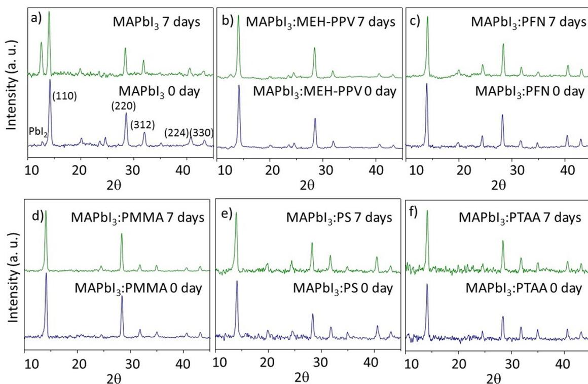
**Figure S4.** X-Ray diffraction pattern of (a) MAPbI<sub>3</sub> and MAPbI<sub>3</sub>:polymer (b) MEH-PPV, (c) PFN, (d) PMMA, (e) PS, (f) PTAA thin films, which were exposed to ambient air.
