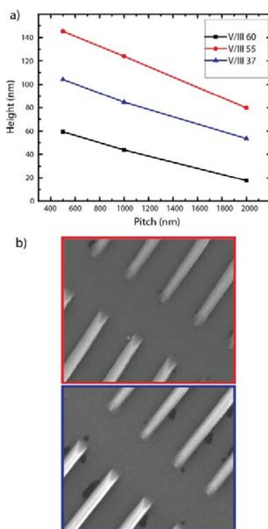
**Figure 1:** a) Pitch Dependency of the GaAs nanomembrane height in function of V/III ratio which is controlled via changing Arsenic BEP (Beam Equivalent Pressure) by keeping Gallium (Ga) growth rate fixed at 0.3 Å/s b) SEM images of the samples grown under the conditions specified above, the colour of the frame is matched to the colour of the data line.
