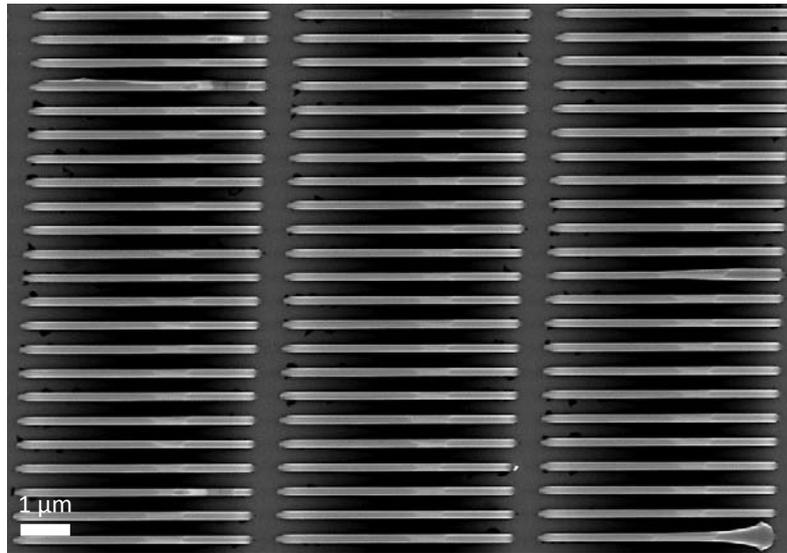
**Figure 6:** Part of a 1mmx1mm size pattern. Nanoscale membranes are grown at 640 °C and 17 of V/III.
