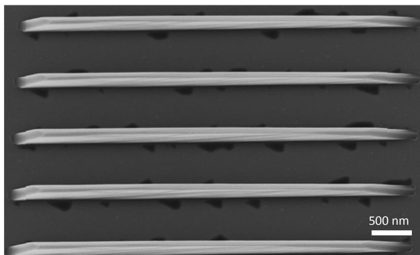
**Figure 3:** Twin defects formed at the side facets of the GaAs nanoscale membranes grown at 660 °C
