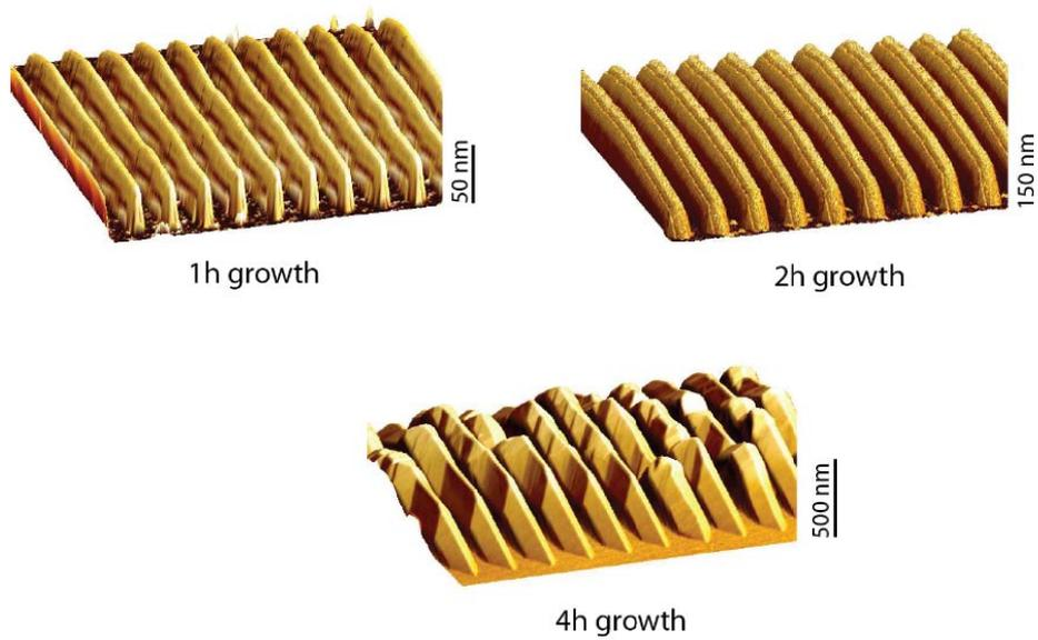
**Figure 2:** Time series of samples grown with 0.3 A/s Ga rate and 60 of V/III ratio.
