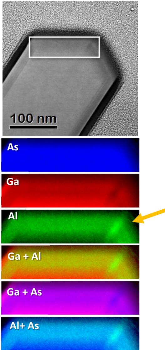
**Figure 4:** EELS mapping at the top part of the membranes along the [112] direction.
