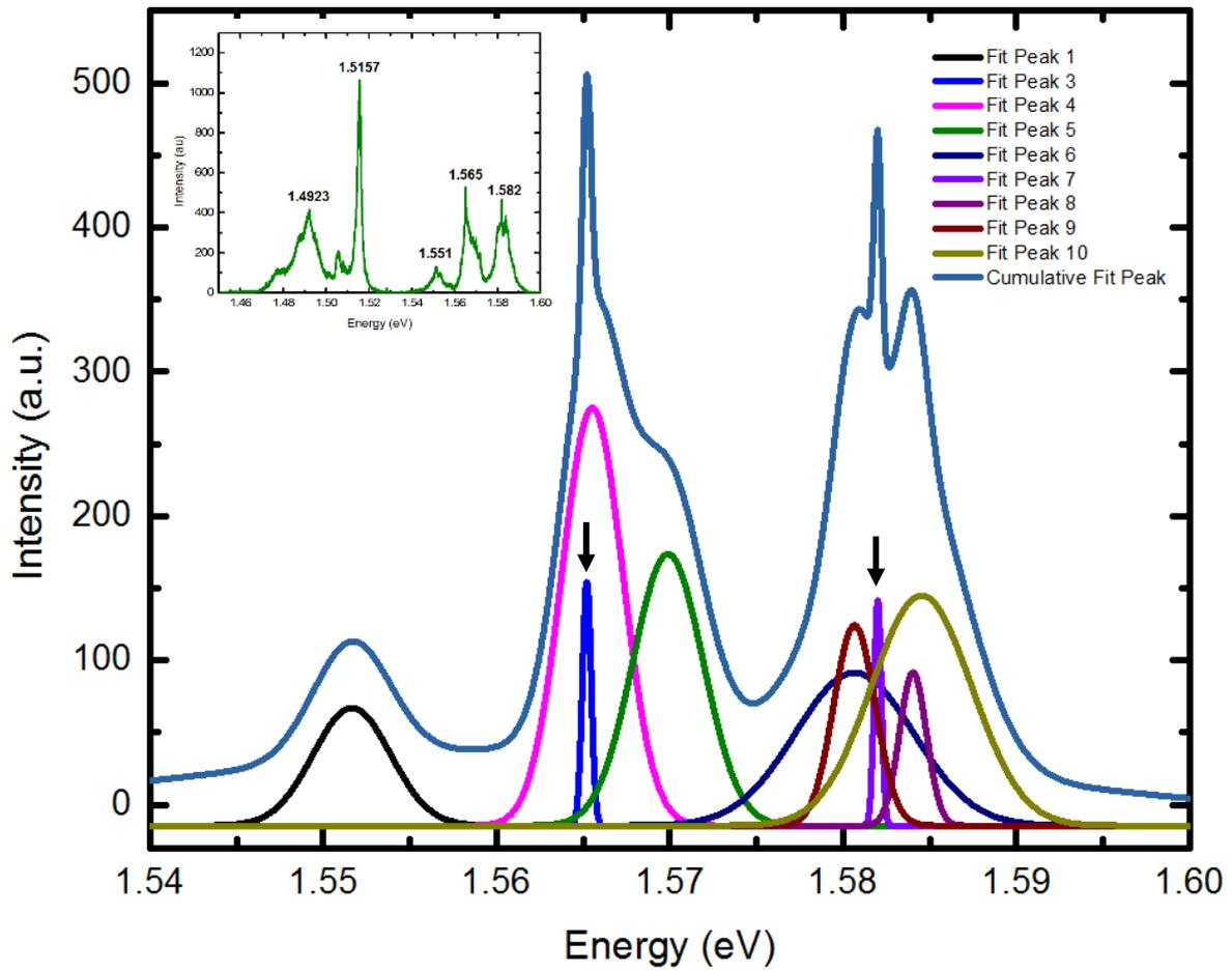
**Figure 5:** 1.54 eV-1.60 eV section of a PL spectrum of a GaAs nanoscale membrane with 8 nm (nominal) of GaAs QW sandwiched between 20 nm (nominal) of AlGaAs layers. Full spectrum is shown in the inset
