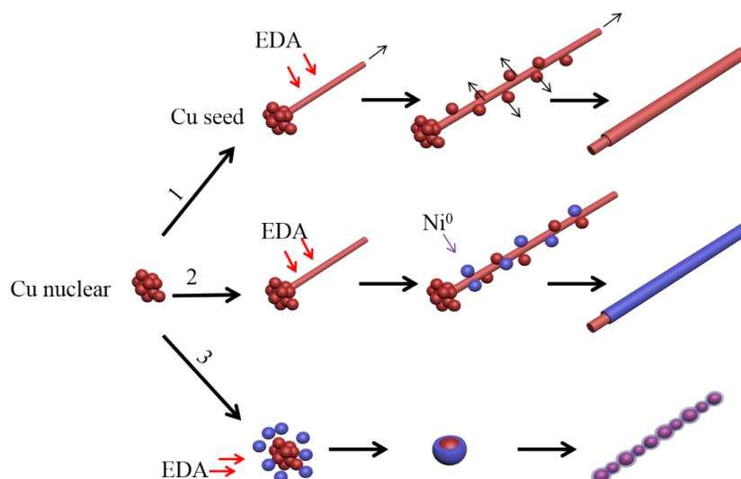
**Fig. S3** Schematic of neat Cu and Cu-Ni NW growth process.
