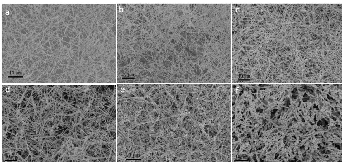
**Fig. S1** SEM images of Cu-Ni NWs with Cu/Ni molar ratio of (a) 3.5:1, (b) 2.1:1, (c) 1.6:1, (d) 1:1.4, (e) 1:2 and (f) 1:3.3.
