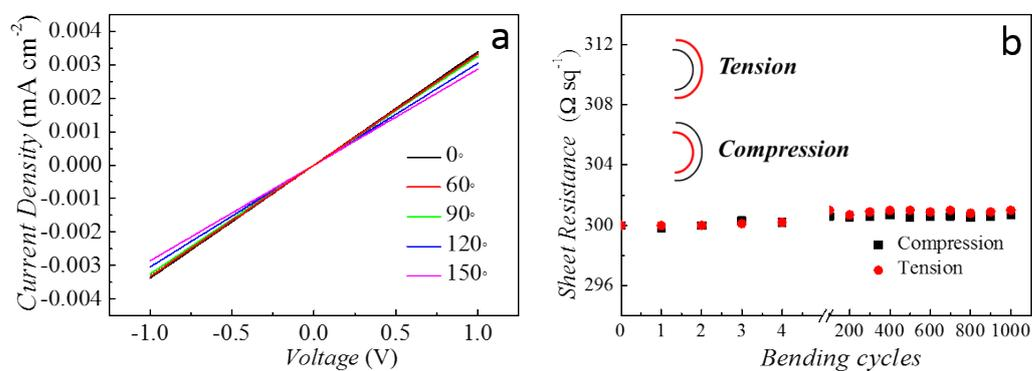
**Fig. S5** Flexibility tests of Cu-Ni(1:1) TCFs. (a) I-V curves measured at 0-150° bending angles; (b) Resistance changing under continuous bending.
