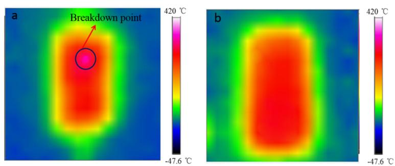
**Fig. S7** Infrared thermal images of (a) Cu NW and (b) Cu-Ni NW heaters operated at 12 V.
