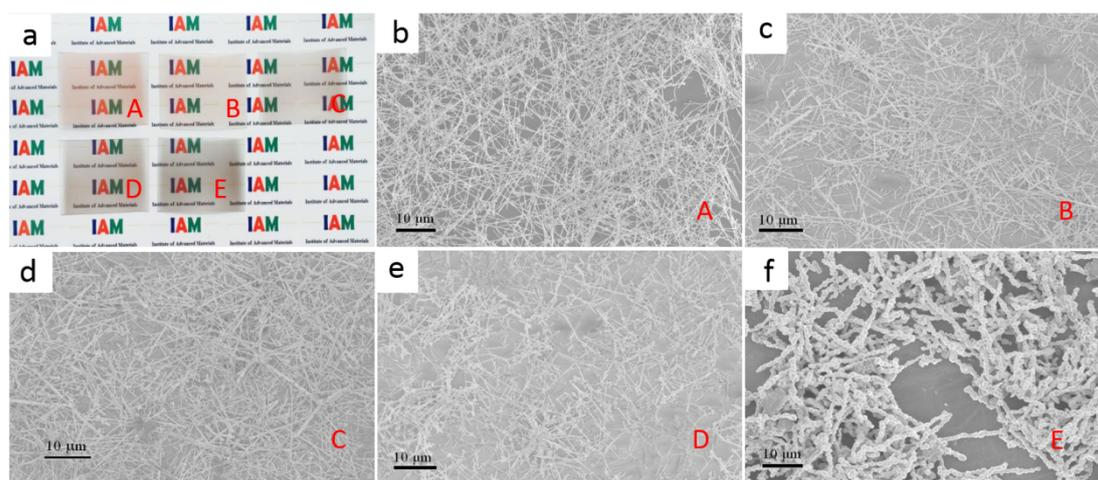
**Fig. S6** (a) Photograph of Cu-Ni TCFs prepared using different Cu-Ni NWs. SEM images of (b) Cu-Ni(3.5:1), (c) Cu-Ni(2.1:1), (d) Cu-Ni(1:1), (e) Cu-Ni(1:2) and (f) Cu-Ni(1:3.3) TCFs.
