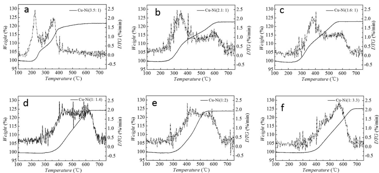
**Fig. S4** TG and DTG curves of (a) Cu-Ni(3.5:1), (b) Cu-Ni(2.1:1), (c) Cu-Ni(1.6:1), (d) Cu-Ni(1:1.4), (e) Cu-Ni(1:2), and (f) Cu-Ni(1:3.3) NWs.
