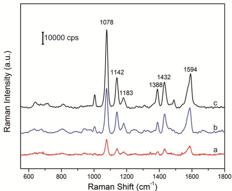
**Figure S2.** SERS spectra of  $10^{-5}$  M PATP absorbed on  $\text{Fe}_3\text{O}_4@\text{Ag}$  microspheres prepared at following concentrations of  $\text{AgNO}_3$ : a- 0.05 mM, b- 0.1 mM, and c- 0.2 mM.
