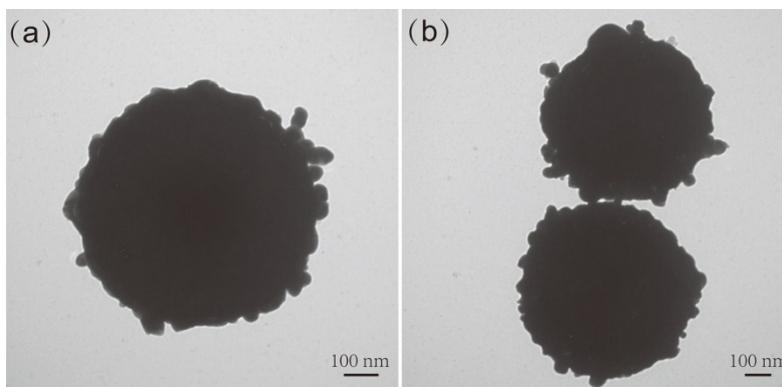
**Figure S6.** TEM images of (a)  $\text{Fe}_3\text{O}_4@Ag\text{-PEI-60nm Au@Ag}$  CSSM, (b) 70nm Au@Ag CSSM. Sparse satellites were observed on the surface of  $\text{Fe}_3\text{O}_4@Ag$  microspheres, suggesting the Au@Ag NPs larger than 55 nm could not assemble uniformly.
