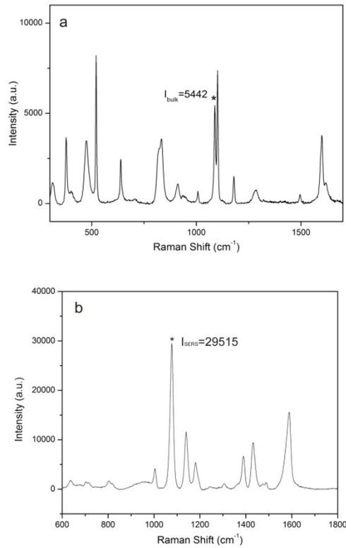
**Figure S7** (a) Raman spectrum of pure PATP. (b) SERS spectrum of PATP with a concentration of  $10^{-9}$ M.
