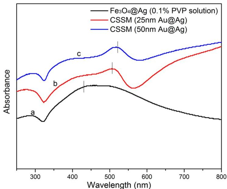
**Figure S5.** UV-vis spectra of a-  $\text{Fe}_3\text{O}_4@Ag$  microspheres in 0.1% PVP water solution, b- CSSM (25nm Au@Ag) and c- CSSM (50nm Au@Ag) in water solution.
