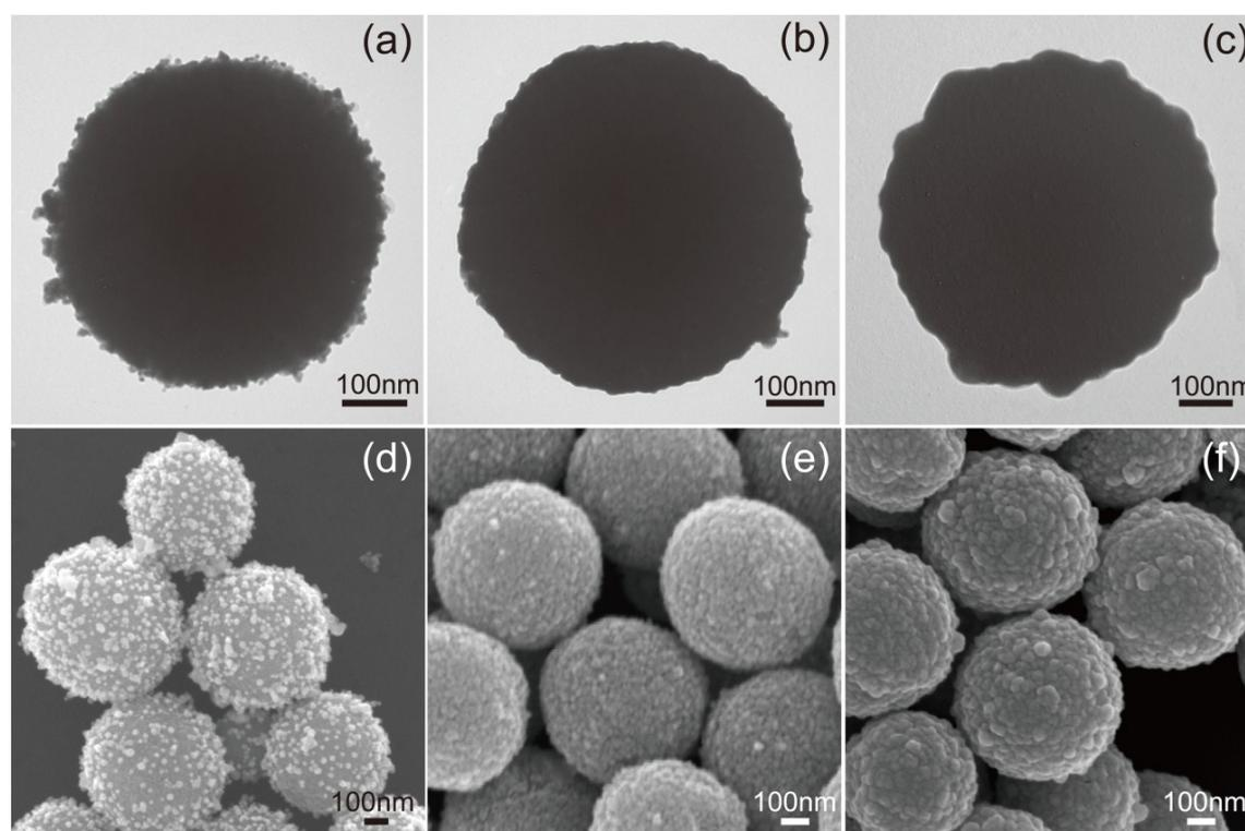
**Figure S1.** TEM images of  $\text{Fe}_3\text{O}_4@Ag$  microspheres synthesized with different concentration of  $\text{AgNO}_3$ : (a) 0.05 mM, (b) 0.1 mM, (c) 0.2 mM and their corresponding SEM images (d), (e), and (f), respectively.
