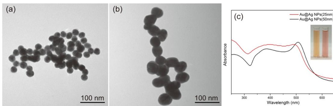
**Figure S4.** Characterization of the synthesized Au@Ag NPs. (a) TEM images of 25nm Au@Ag NPs, (b) TEM images of 50 nm Au@Ag NPs and (c) UV-visible spectra of the two Au@Ag NRs. The inset shows the photograph of 25nm Au@Ag NRs (right) and 50 nm Au@Ag NRs (left).
