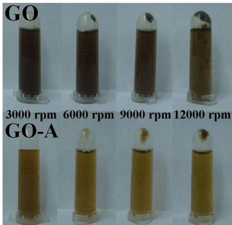
**Fig. S3.** The colloidal dispersions of GO and GO-A with the concentration of *ca.*  $0.75 \text{ mg mL}^{-1}$  centrifuged at 3000, 6000, 9000 and 12000 rpm for 8 min, respectively.
