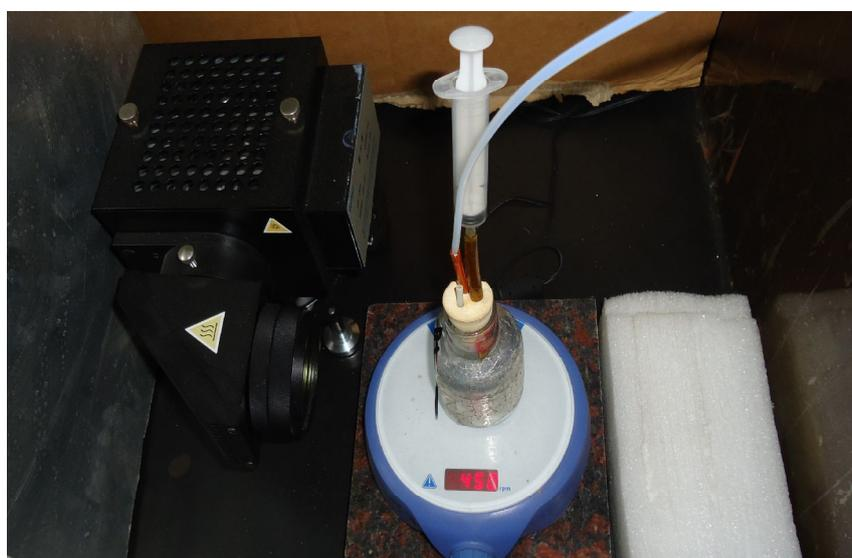
**Fig. S18.** Photograph of the experimental setup for photocatalytic anaerobic reduction of nitroaromatic compounds.
