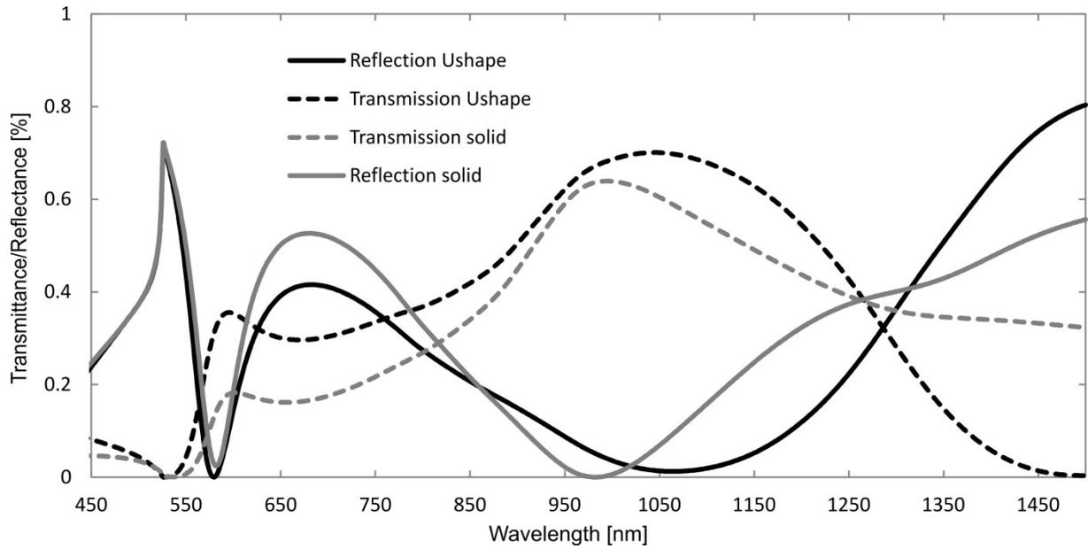
Figure S3: Comparison of the optical properties of U-shaped wires and solid aluminum wires (missing the backside groove)
