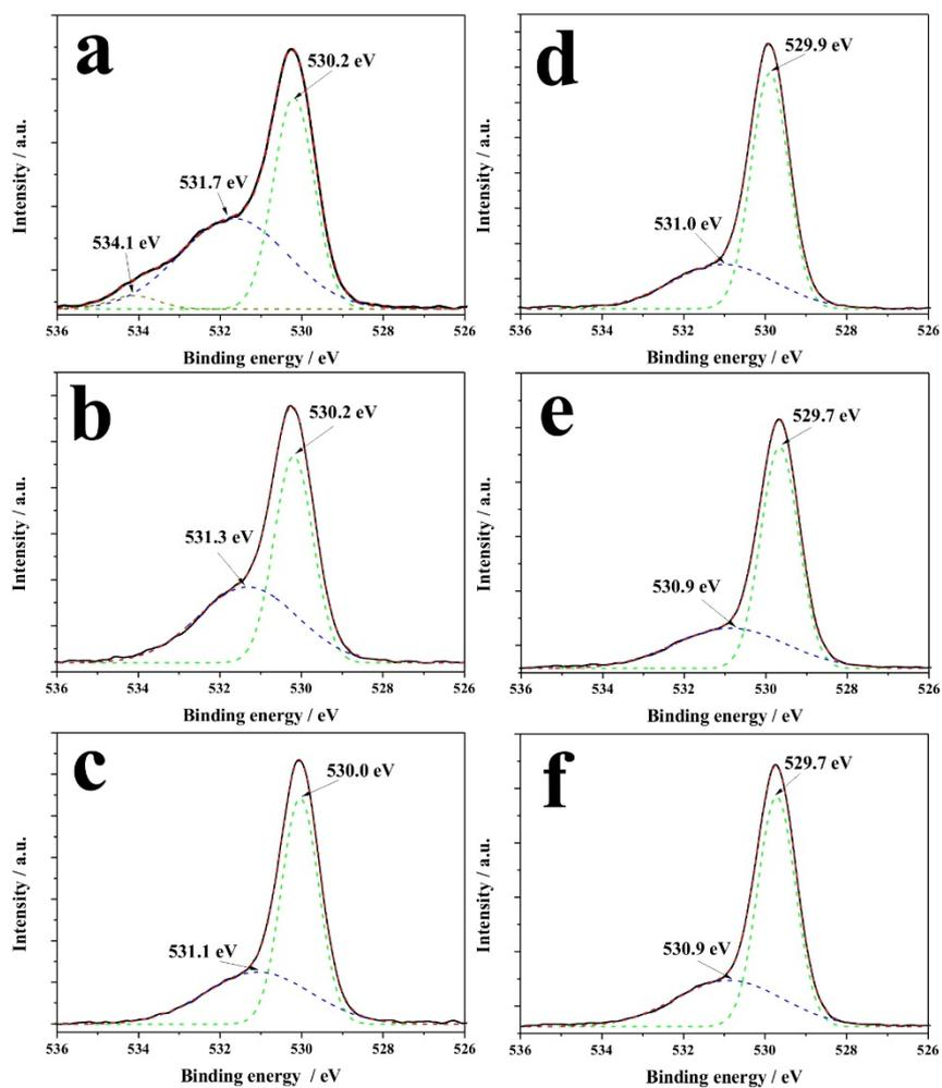
**Fig. S6** XPS core level of O 1s after annealing at different temperatures: (a) no annealing, (b) 200 °C, (c) 300 °C, (d) 400 °C, (e) 500 °C, (f) 600 °C.
