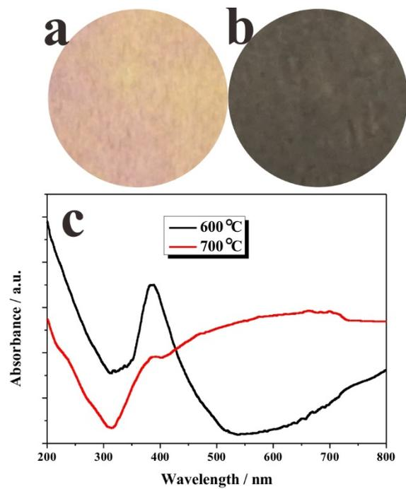
**Fig. S3** Digital photos of patterned titanium foils annealed at (a) 600 °C and (b) 700 °C and (c) UV-vis diffuse reflectance absorption spectra.
