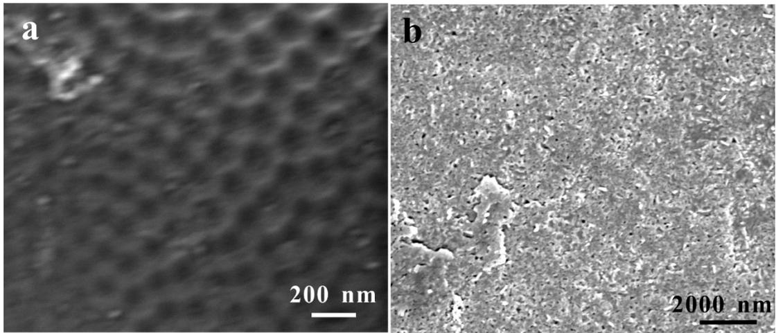
**Fig. S2** SEM image of patterned titanium foil annealed at (a) 600 °C and (b) 700 °C.
