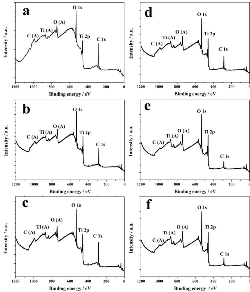
**Fig. S5** XPS survey of TOPCs after annealing at different temperatures: (a) no annealing, (b) 200 °C, (c) 300 °C, (d) 400 °C, (e) 500 °C, (f) 600 °C.
