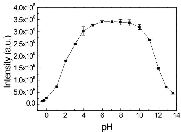
**Fig. S8** Effect of pH on the fluorescence intensity of hydrothermal-prepared HCDs.
