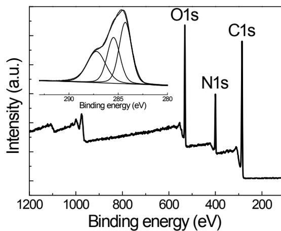
**Fig. S7** XPS analysis of HCDs prepared by hydrothermal method.
