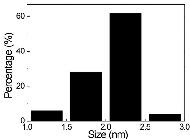
**Fig. S1** The size distribution of CDs obtained by counting the average size of 50 nanoparticles from the TEM image.
