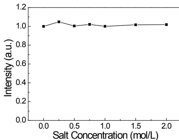
**Fig. S5** The influence of ionic strengths on the fluorescence intensity of CDs. The ionic strengths were controlled by various the concentrations of NaCl (from 0 to 2.0 M).
