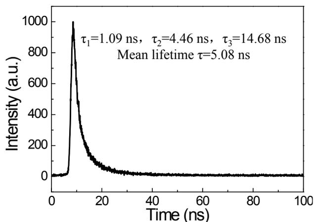
**Fig. S4** The time-resolved fluorescence decay curve of CDs at the wavelength of 360 nm.
