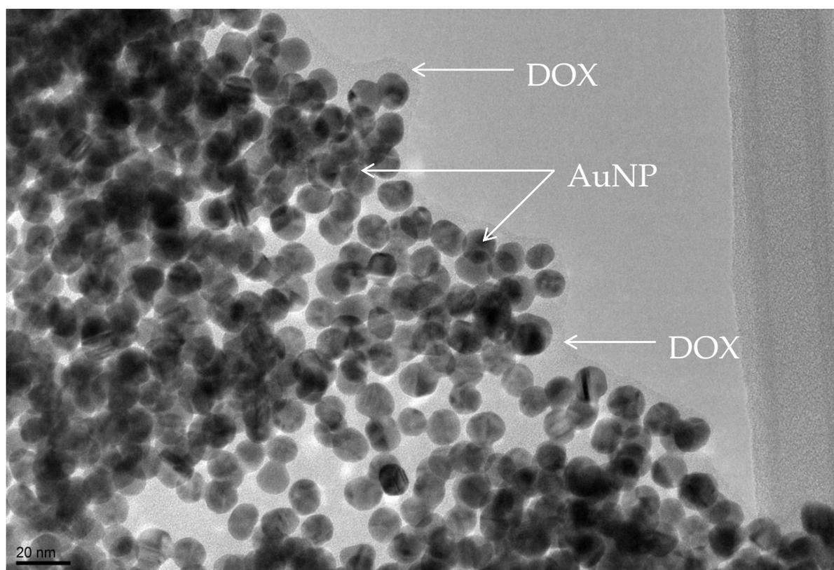
**Figure S3.** TEM micrograph of DOX-AuNP conjugates. DOX:AuNP molar concentration ratio = 307:1 (Scale bar: 20 nm).
