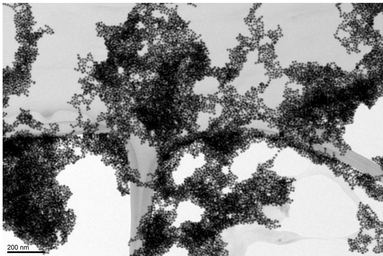
**Figure S4.** Figure S4. TEM micrograph of DOX-AuNP conjugates. DOX:AuNP molar concentration ratio = 307:1 (Scale bar: 200 nm).
