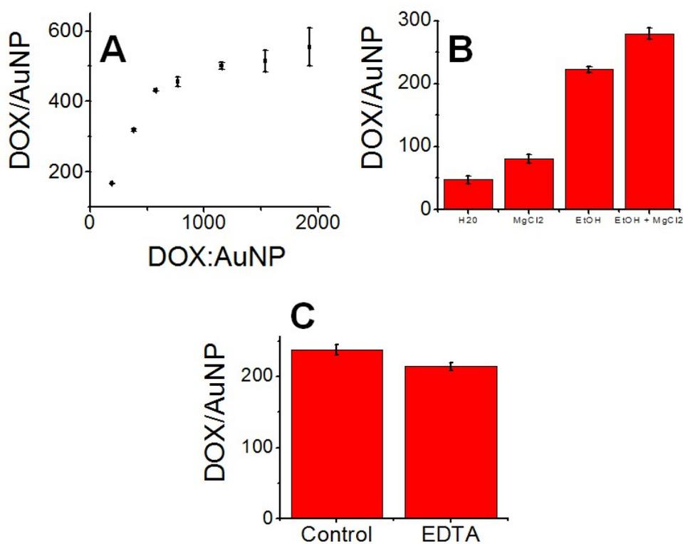
Figure S7. (A) Original DOX-AuNP loading isotherm including standard error bars. (B) Desorption of DOX from AuNP surface after treatment with  $\text{MgCl}_2$  ([62.5 mM]), EtOH (31.25% v/v) and EtOH- $\text{MgCl}_2$ . DOX:AuNP ratio = 317:1. (C) Adsorption of DOX to AuNP surface after EDTA ([3.84  $\mu\text{M}$ ]) treatment of AuNP. DOX:AuNP ratio = 308:1.
