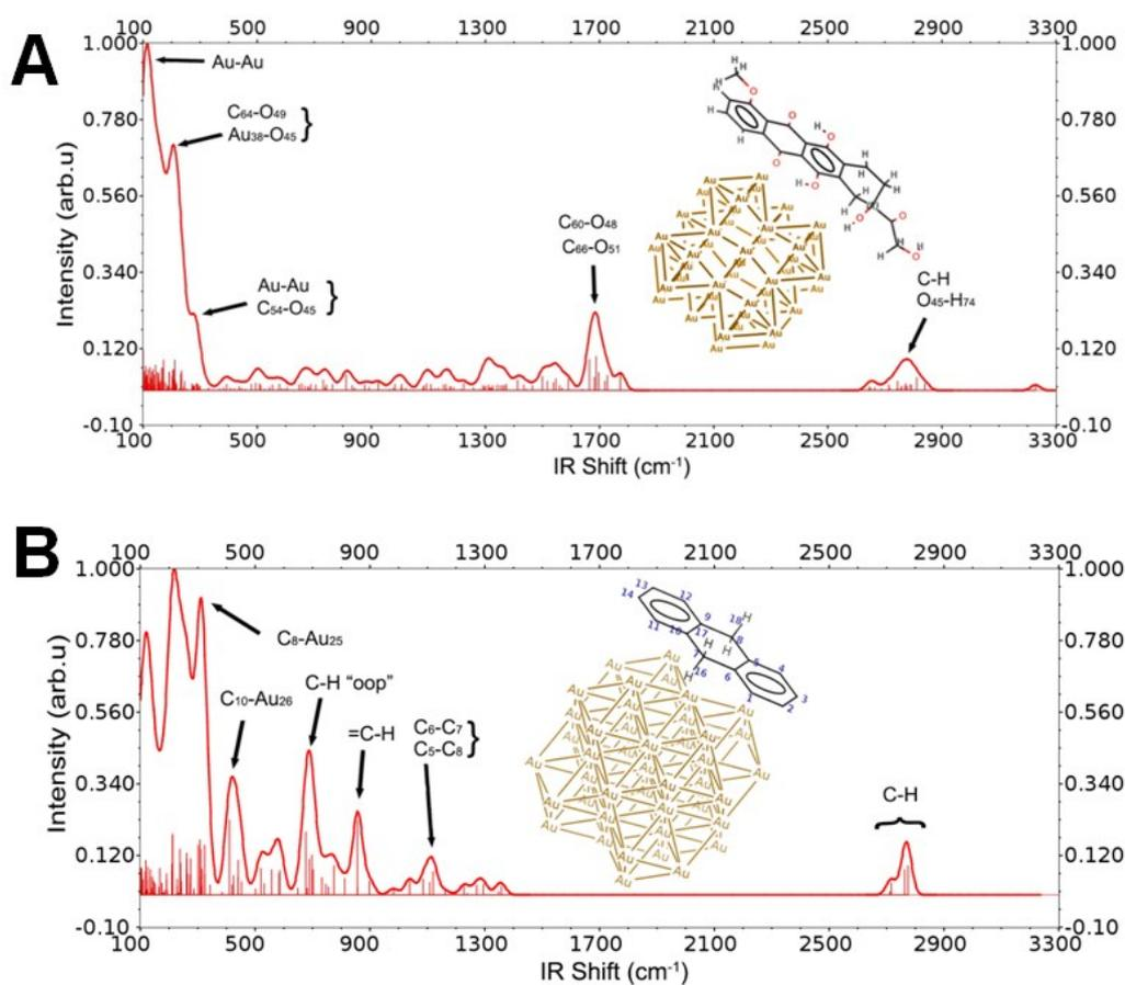
**Figure S10.** (A) Modelling of IR spectrum of DOX without ring 1 connected to amine moiety with a 0.5 nm AuNP. (B) Modelling of IR spectrum of the DOX-like anthracene with 0.5 nm AuNP.
