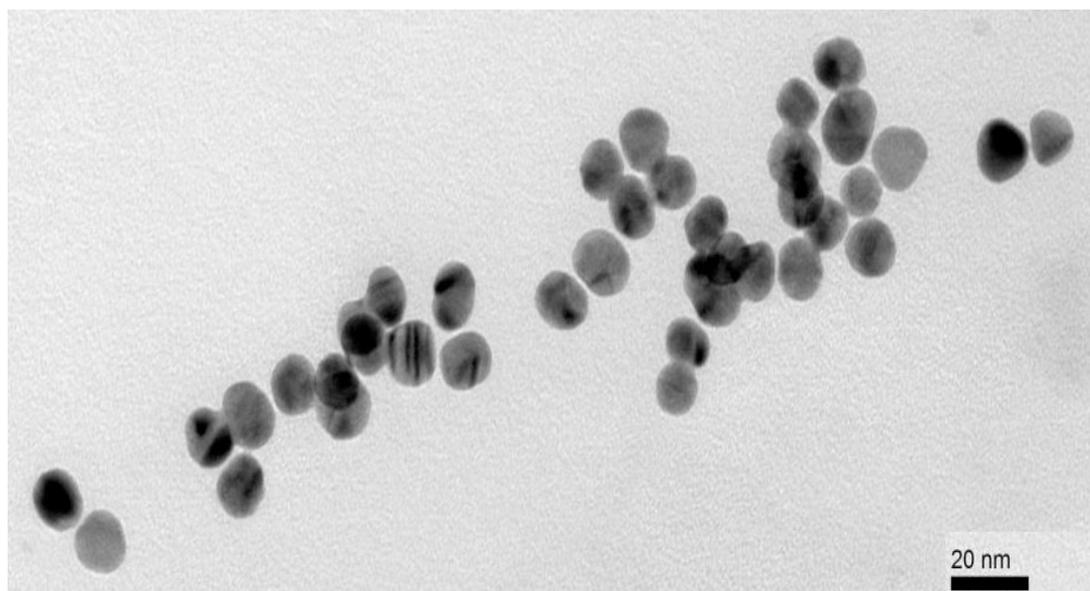
**Figure S2.** TEM micrograph of ~13 nm citrate-capped AuNP used in this work (Scale bar: 20 nm).
