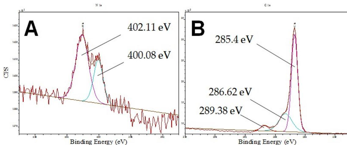
Figure S8. XPS N 1s (A) and C 1s (B) deconvoluted spectra for DOX-AuNP conjugate solutions.
