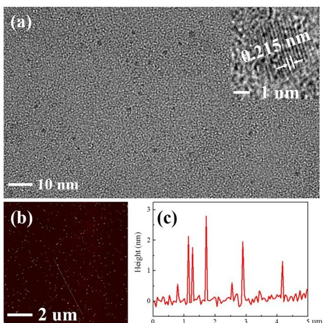
**Fig. S3** A typical TEM image (a) and AFM image (b) of the BN QDs prepared by the sonication and solvothermal treatment of the bulk BN flakes in DMSO, and the height profile of the as-prepared BN QDs (c). Inset of (a): the HRTEM image of the BN QDs.
