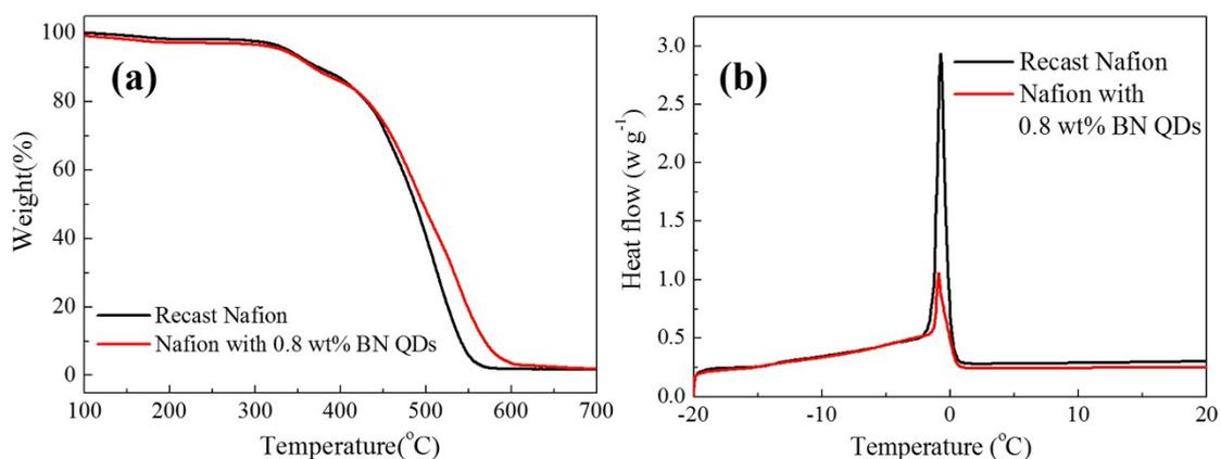
**Fig. S9** TGA (a) and DSC (b) curves of the recast Nafion and 0.8 wt% BN QDs/Nafion.
