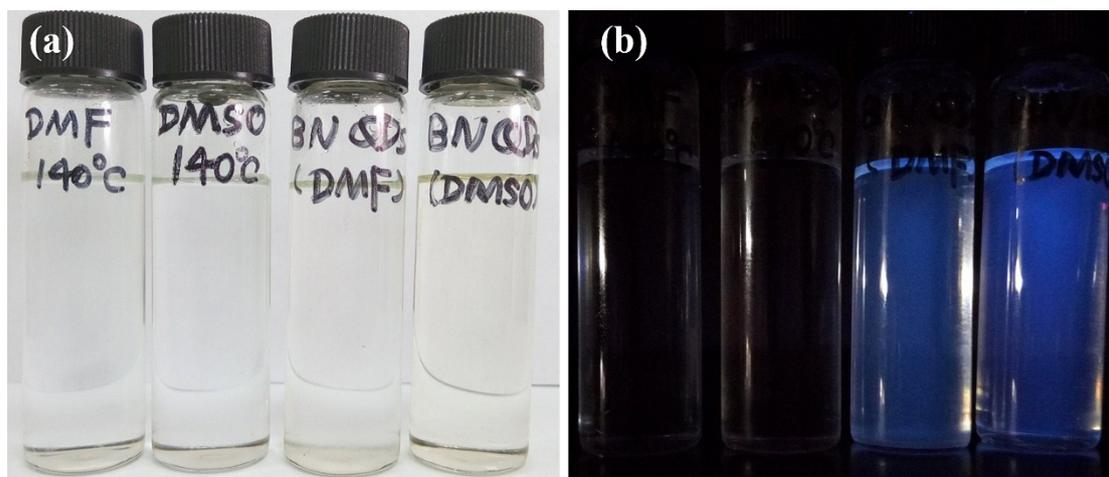
**Fig. S4** Typical digital photographs of DMF, DMSO, DMF with the addition of BN raw materials and DMSO with the addition of BN raw materials in natural light (a) and under 365 nm UV radiation (b) after the same sonication-solvothermal process.
