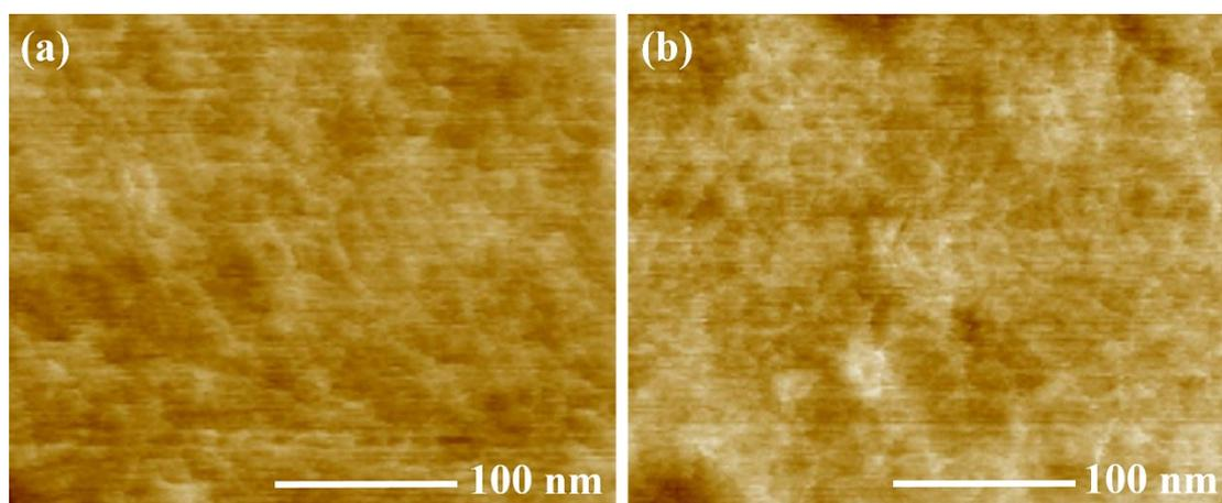
**Fig. S10** Typical AFM images of recast Nafion (a) and the Nafion membrane with 0.8 wt% BN QDs (b).
