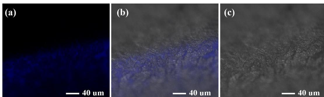
**Fig. S8** (a) The CLSM image of labeled Nafion membrane with 0.8 wt% BN QDs, (b) the overlapped image of the darkfield image and brightfield image, (c) the corresponding brightfield image.
