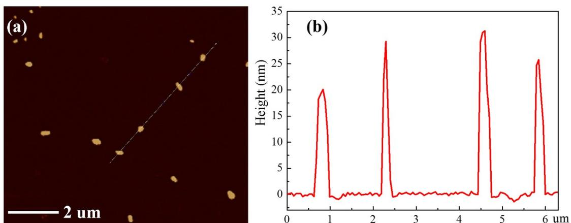
**Fig. S2** AFM images of BN nanosheets prepared by the sonication treatment of bulk BN flakes in DMF for 8 h.
