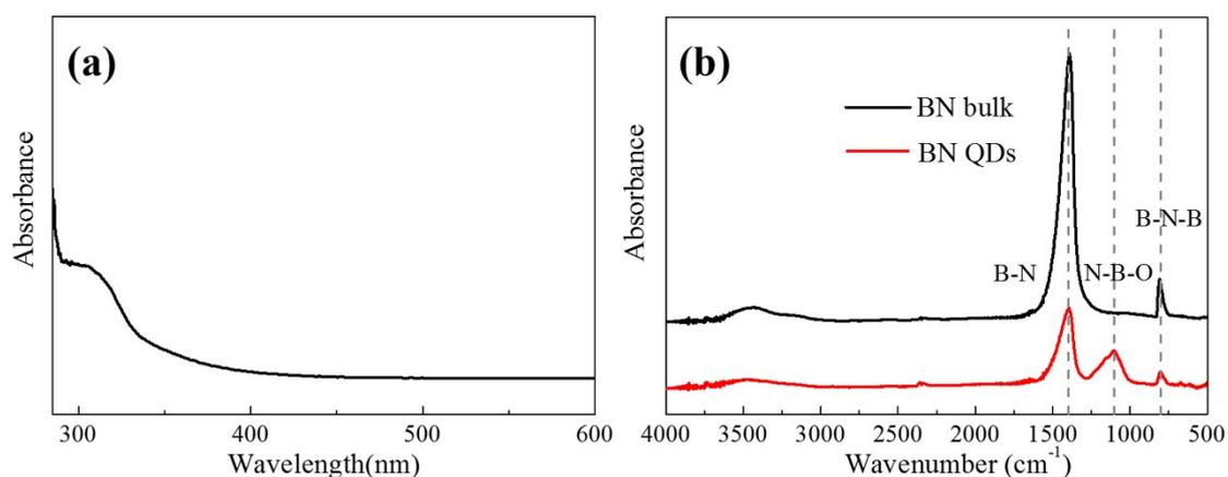
**Fig. S5** UV-vis spectrum of the BN QDs and FTIR spectra of the bulk BN flakes and BN QDs.
