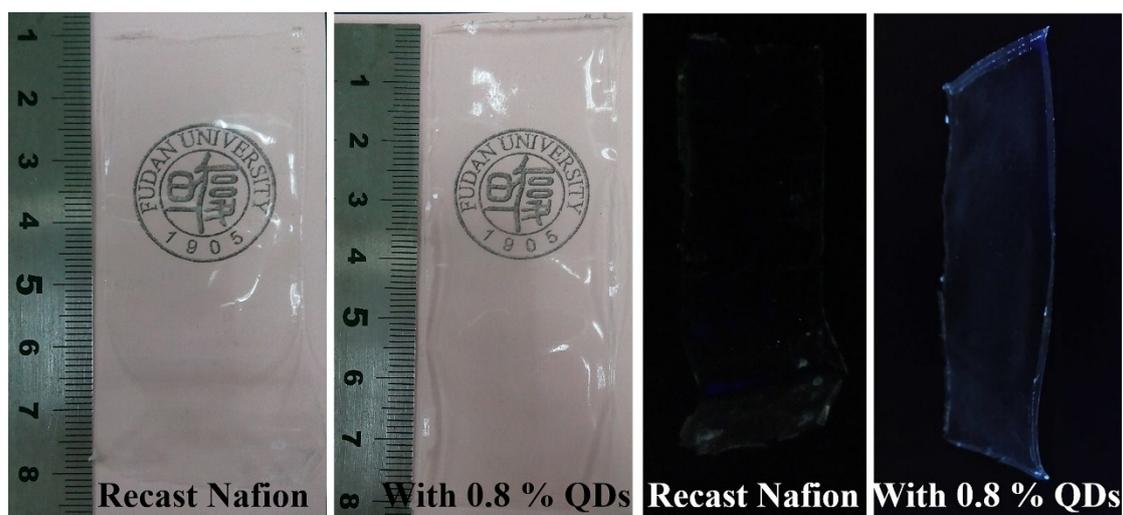
**Fig. S7** Digital photographs of the as-prepared PEMs under visible light (left) and under 365 nm UV irradiation (right).
