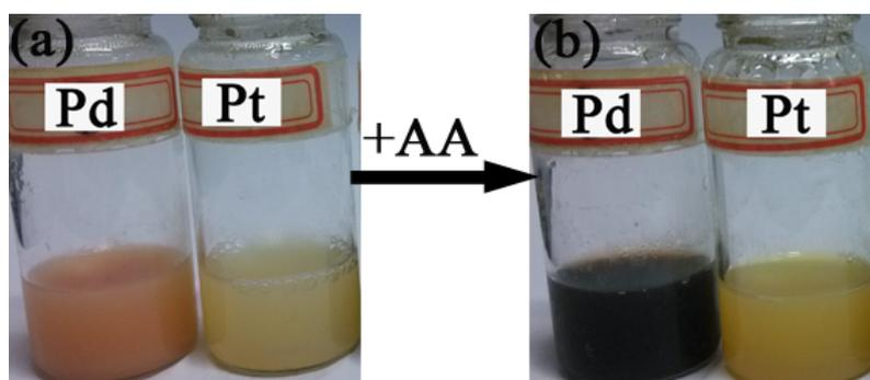
**Figure S4.** Photographs of CPC aqueous solutions containing Pd and Pt precursors respectively followed by the introduction of 80 mM NaBr before (a), after (b) the addition of reducing agent AA for 5 min at 90 °C.
