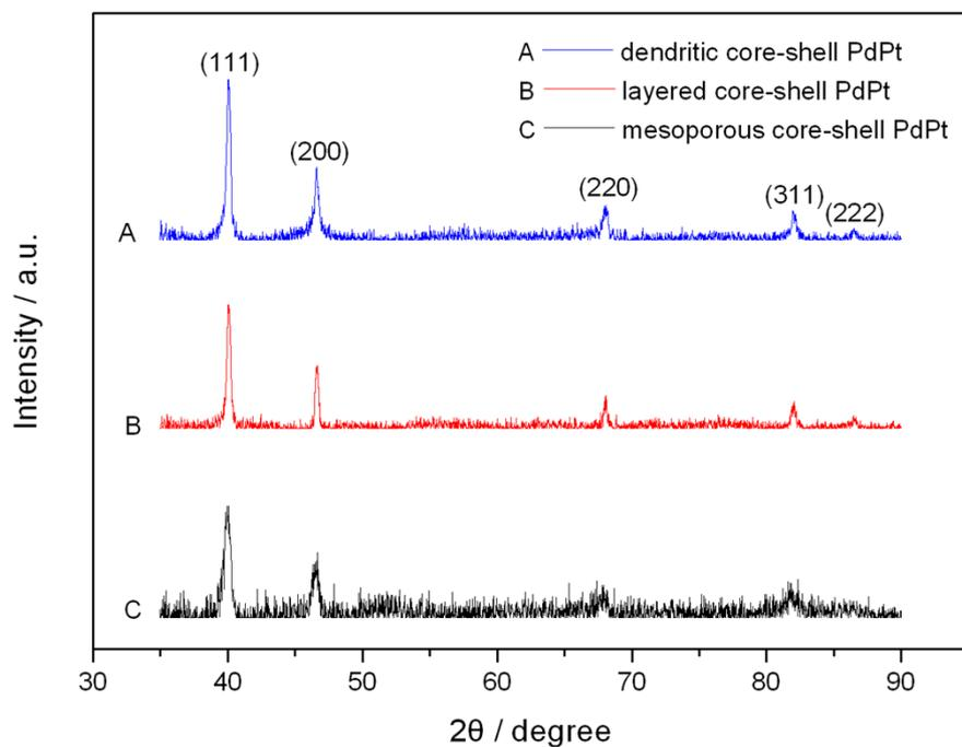
**Figure S2.** Powder XRD pattern of dendritic core-shell (A), layered core-shell (B) and mesoporous core-shell (C) PdPt bimetallic nanoparticles.
