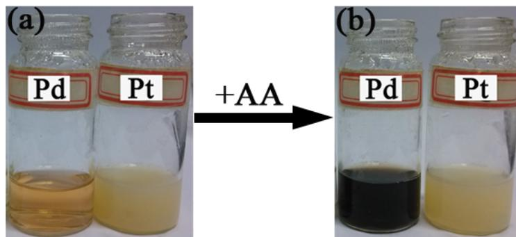
**Figure S1.** Photographs of CPC aqueous solutions containing Pd and Pt precursors respectively before (a), and after (b) the addition of reducing agent AA at 90 °C.
