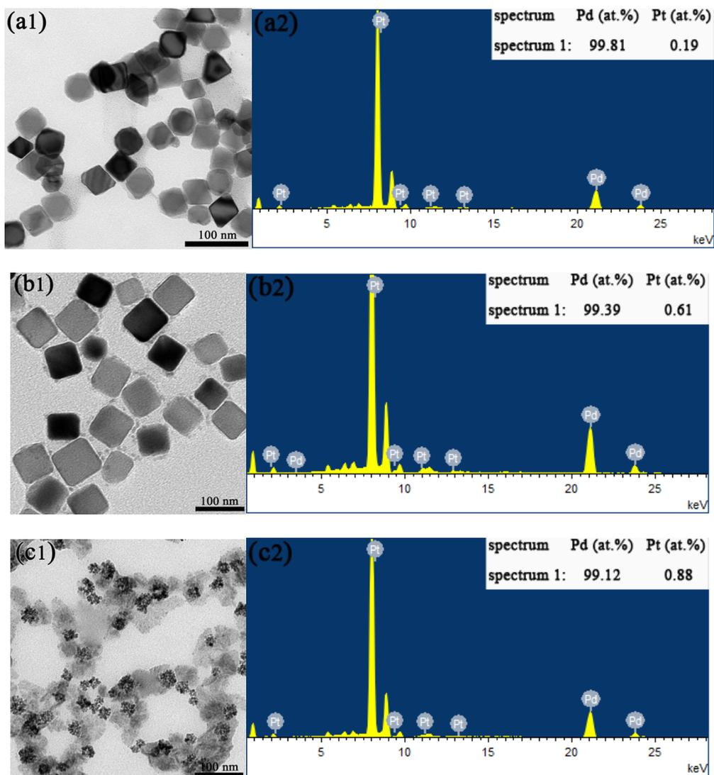
**Figure S6.** TEM image and the corresponding EDS results of dendritic core-shell (a1, a2), layered core-shell (b1, b2) and mesoporous core-shell (c1,c2) PdPt bimetallic nanoparticles for 1 min reaction time (All the strong peak located at 8 keV is actually the position of Cu element from copper grid with carbon support film loading the samples for TEM test, and the peak is too strong to weaken the signal of Pd around 3 keV.).
