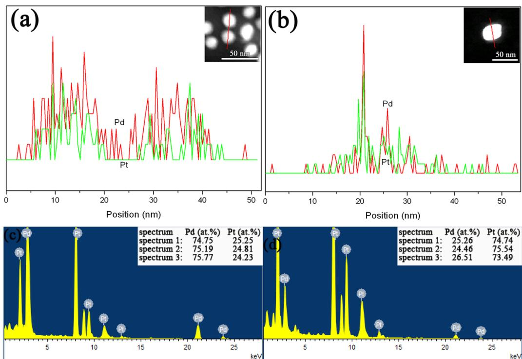
**Figure S8.** EDX line scan (a, b), EDS (c, d) results of layered (a, c) and mesoporous (b, d) PdPt bimetallic nanoparticles corresponding to Figure 5b3 and Figure 5c3, respectively.
