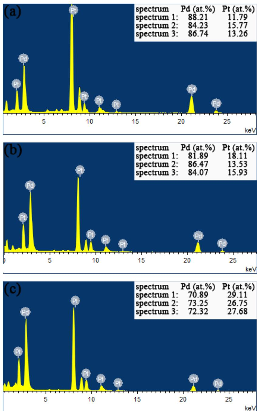
**Figure S3.** EDS results of dendritic core-shell (a), layered core-shell (b) and mesoporous core-shell (c) PdPt bimetallic nanoparticles.
