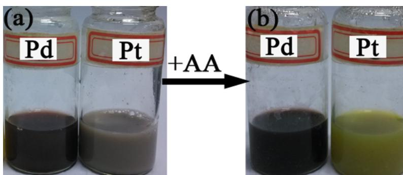
**Figure S5.** Photographs of CPC aqueous solutions containing Pd and Pt precursors respectively in the presence of 80 mM NaI before (a), and after (b) the addition of reducing agent AA for 10 min at 90 °C.
