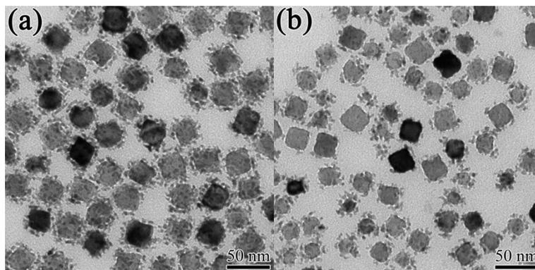
**Figure S9.** TEM images (a–b) of dendritic core-shell PdPt bimetallic nanoparticles without the involvement of any additional halide ions in the case of (a) the precursors of Pd and Pt simultaneously present in the mixture solution for one-step method, (b) Pd nanocubes premade as seeds followed by the addition of Pt precursors for two-step method.
