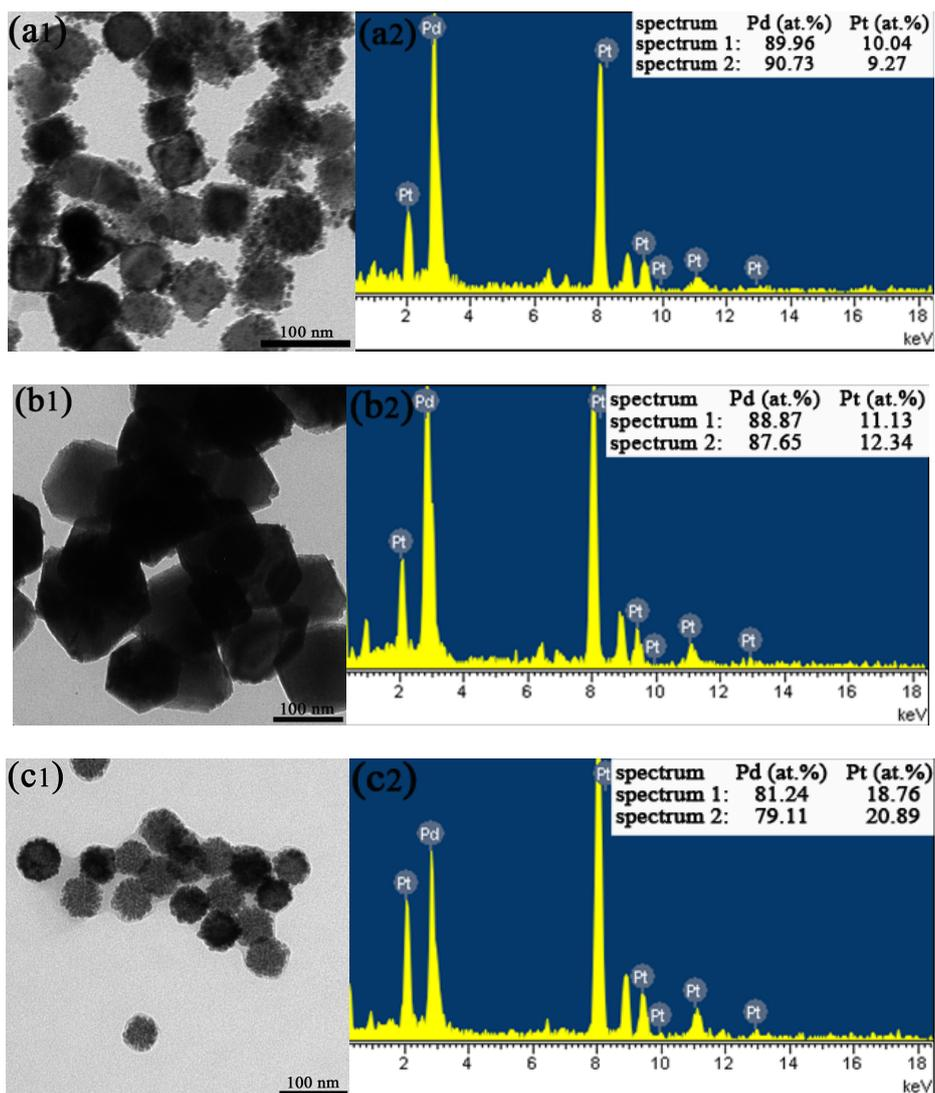
**Figure S7.** TEM image and the corresponding EDS results of dendritic core-shell (a1, a2), layered core-shell (b1, b2) and mesoporous core-shell (c1,c2) PdPt bimetallic nanoparticles for 40 min reaction time.
