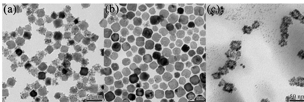
**Figure S10.** TEM images (a–c) of PdPt bimetallic nanoparticles synthesized with pre-made Pd nanocubes as seeds, followed by the addition of Pt precursors and the introduction of various halides: (a) 80 mM NaCl; (b) 80 mM NaBr; (c) 80 mM NaI.
