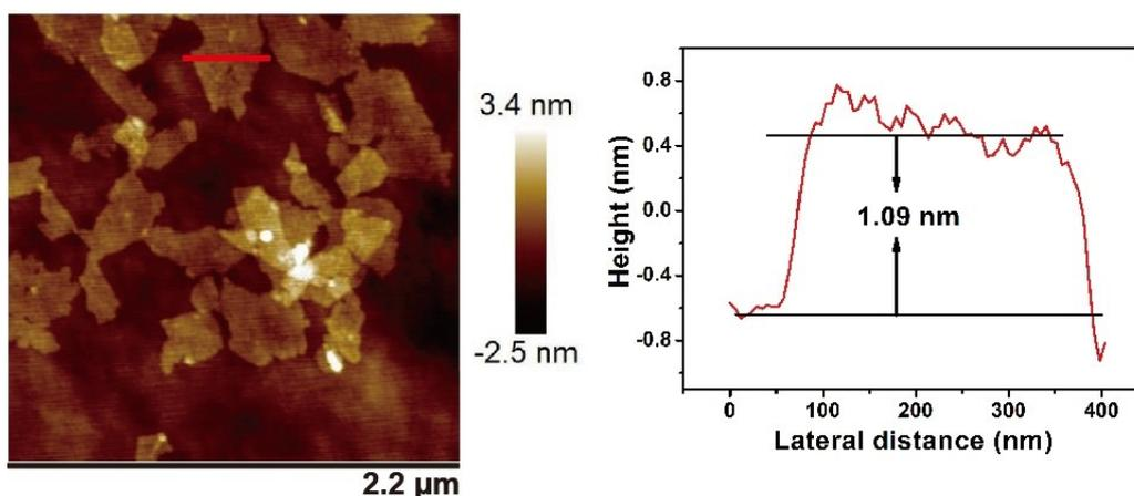
**Fig. S2.** AFM image of MoS<sub>2</sub> nanosheets.
