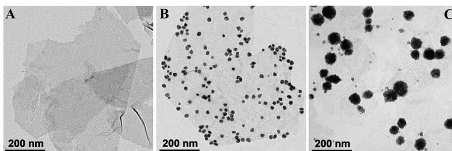
**Fig. S1.** TEM images of (A) MoS<sub>2</sub>, (B) Au/MoS<sub>2</sub> and (C) Pt/MoS<sub>2</sub>.
