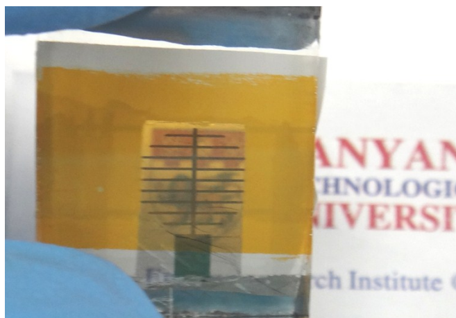
Figure S8. Photo of semi-transparent MAPbBr 3 /CNT solar cell with gold finger electrode.
