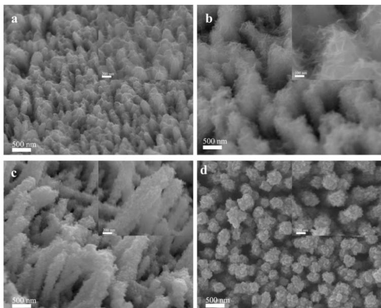
**Figure S5.** SEM images of samples obtained after different reaction temperature. (a) 20 °C, (b) 70 °C, (c) 80 °C, and (d) 100 °C.
