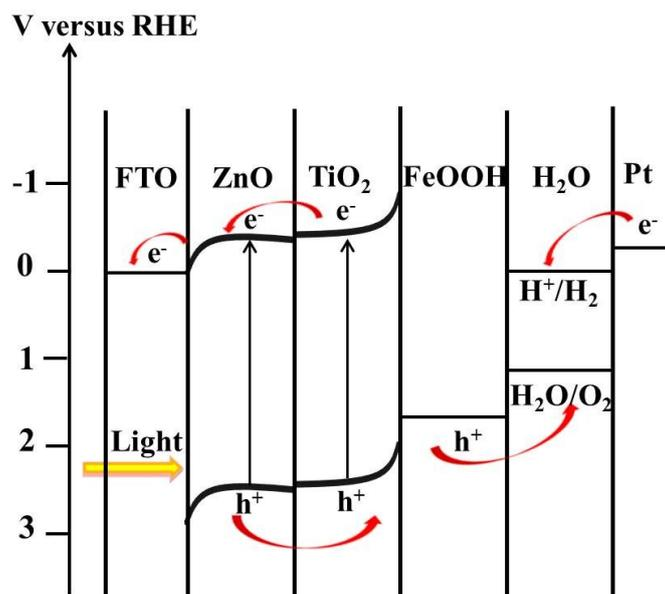
**Figure S7.** Schematic of energy band (quasi-static equilibrium under solar illumination) for 3D ZnO/TiO<sub>2</sub>/FeOOH heterojunction arrays for PEC water splitting.
