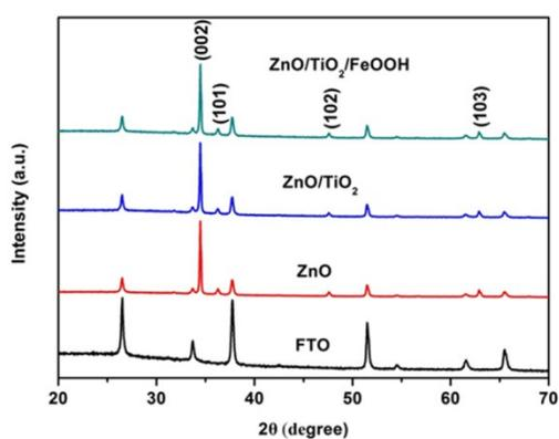
**Figure S1.** XRD patterns of ZnO, ZnO/TiO<sub>2</sub>, and 3D ZnO/TiO<sub>2</sub>/FeOOH heterojunction arrays.
