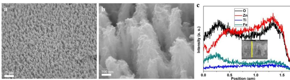
**Figure S2.** Characterization of 3D ZnO/TiO<sub>2</sub>/FeOOH heterojunction arrays. (a, b) SEM images, (c) line scan results.
