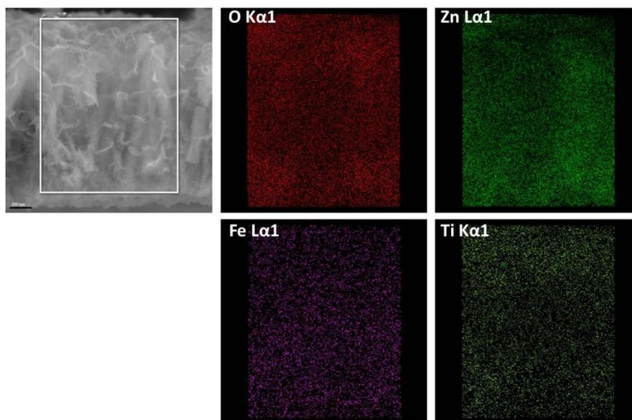
**Figure S3.** EDX elemental mapping of 3D ZnO/TiO<sub>2</sub>/FeOOH heterojunction arrays.
