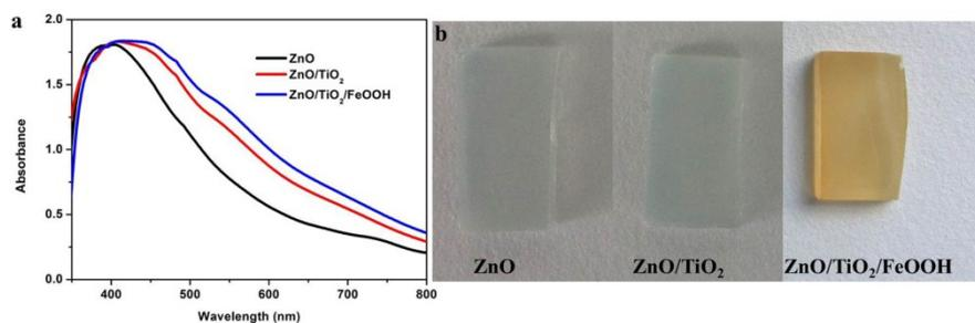
**Figure S4.** (a) UV-vis absorption spectrum and (b) photograph of ZnO, ZnO/TiO<sub>2</sub>, and 3D ZnO/TiO<sub>2</sub>/FeOOH heterojunction, respectively.
